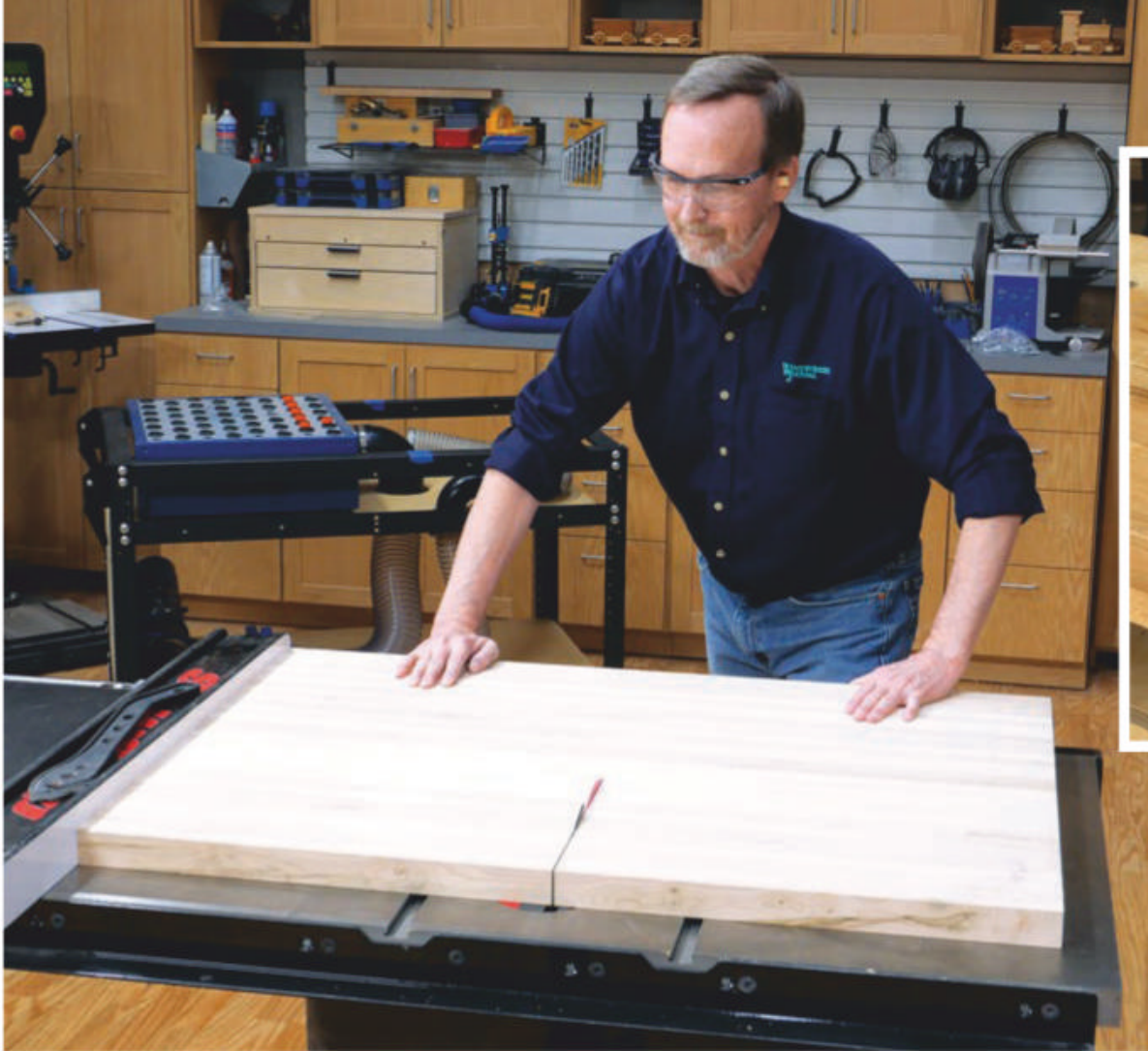
Sawing a 28" x 40" piece of Rockler's butcher block worktop in half creates a section of tabletop for a benchtop spindle sander and the top for a tip-down extension table at the end of the sanding station. The author eased the sharp edges and ends of these workpieces with a 1/8" roundover bit in a compact router.
