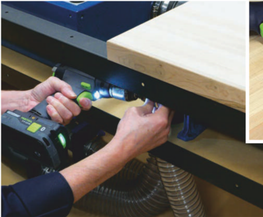
A right-angle drilling attachment (see inset) sure came in handy for driving short screws up through holes in the station's steel stretchers for attaching the butcher block worktop and shelf panels.
