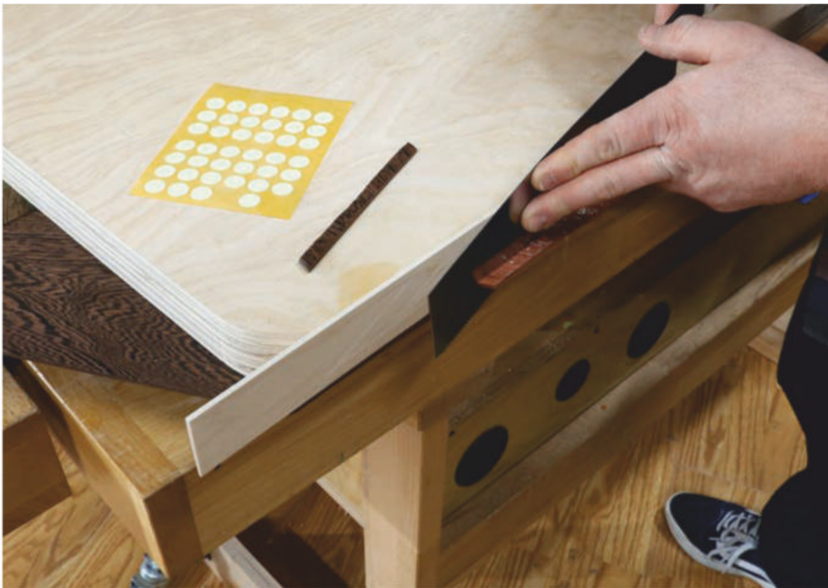
Using a 1/4"-wide spacer attached to the edge of the tabletop core with adhesive sticky dots, the author trimmed away most of the extra chevron length. All four sides were trimmed this way.
