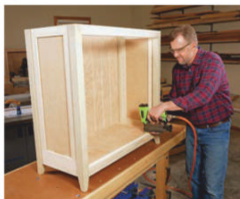
Attach the four cleats to the bottom interior of the cabinet with glue and screws or brads. Then set the bottom panel into place, and secure it with 18-gauge 1½" brad nails driven into the cleats.
