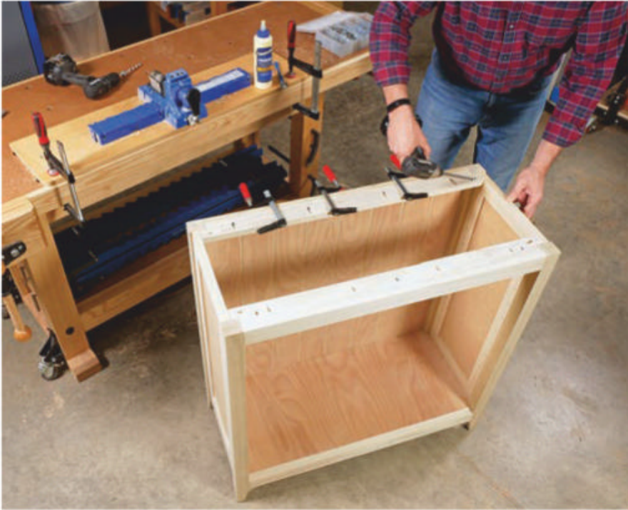
Install the top stretchers on the back panel and upper front rail with glue and pocket screws. Position them slightly below the top edges of the cabinet to ensure that the top panel will screw down tightly against it.
