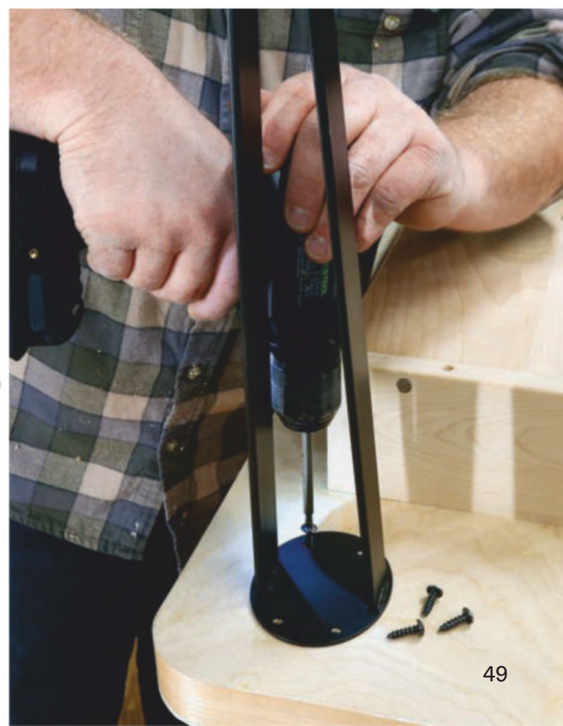
Boring holes for the trimhead screws is a three-step operation. The screws are seated inside the cubby sides where the 1/4" clearance hole stops. The screws hold the cubby tightly to the tabletop.
