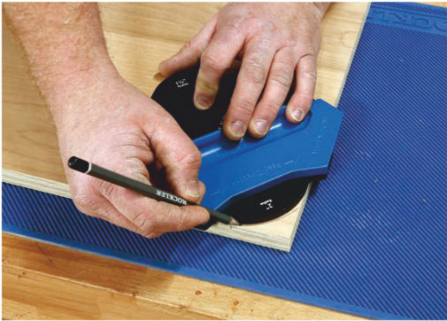
The author marks out the radius on the corners of Top #1. There are a host of ways to get this task done, but uniformity of the shape is very important. The corners are rough-cut with a band saw, staying close to the lines.
