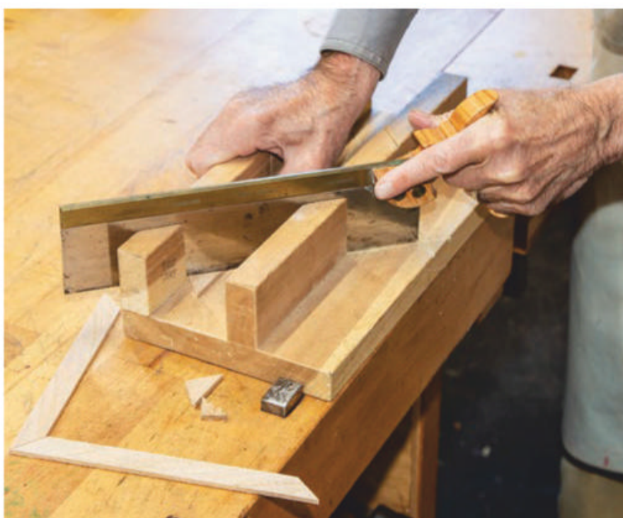
The author uses this 10" Independence 15-point crosscut-filed backsaw for sawing precise miters in his shop-built miter box.
