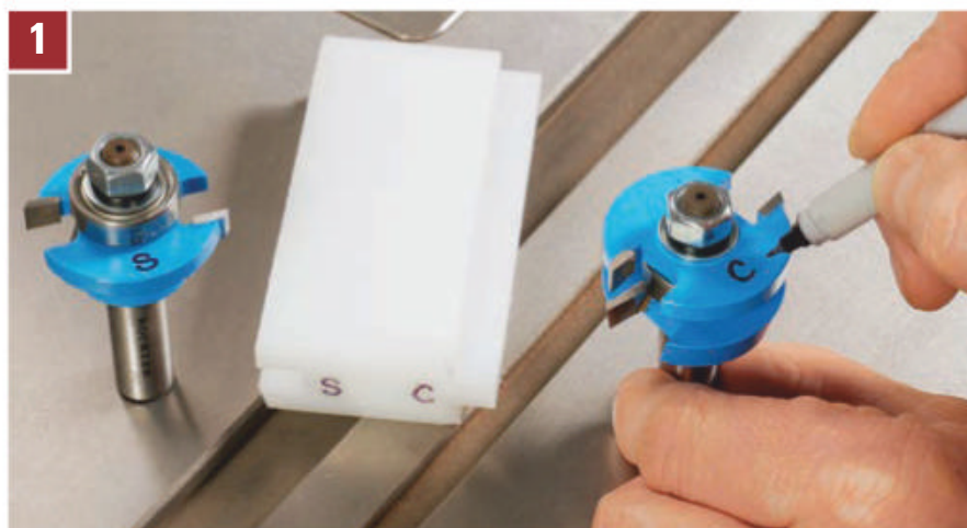
A setup block for some rail-and-stile bit sets, like Rockler's Shaker-style set (item #40431) shown here, can help dial in bit settings efficiently. Label the block and each bit with an “S” and “R” or “C” to denote the joint cuts.
