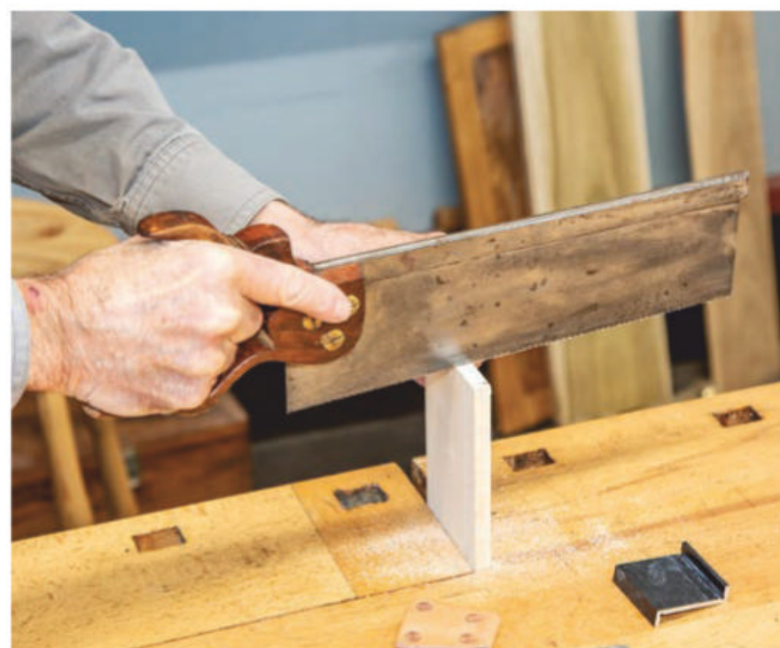
Here's the proper hand grip for a backsaw, with index finger extended. Note that the saw is also held level to the workpiece.
