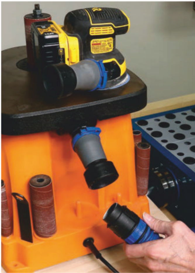
Rockler's new Click-Connect system and FlexiPort Hose Kit provide adapters to fit a variety of handheld and benchtop sander dust ports. An adapter on the hose makes for quick attachment to these tools.
