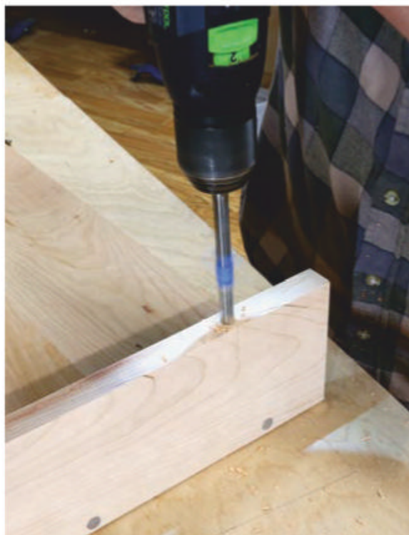
Boring holes for the trimhead screws is a three-step operation. The screws are seated inside the cubby sides where the 1/4" clearance hole stops. The screws hold the cubby tightly to the tabletop.
