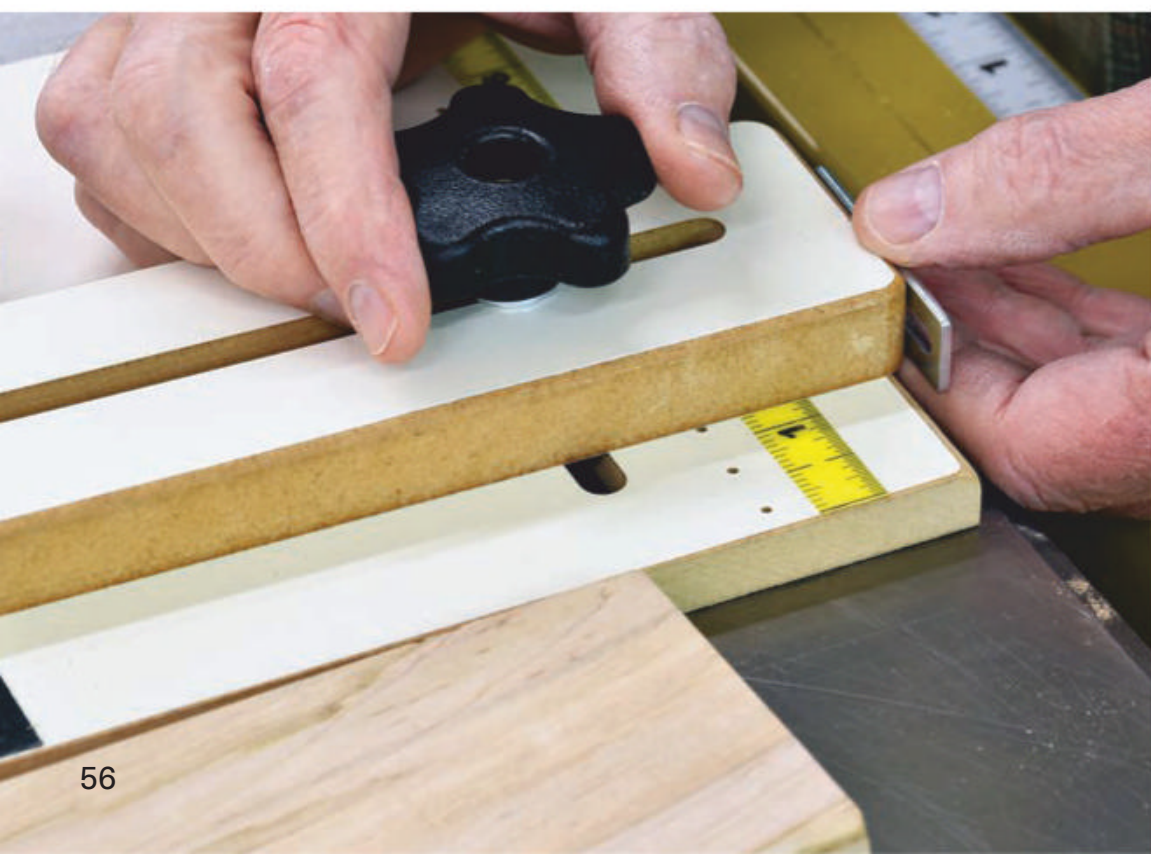
A rabbet cut made along the edge of a workpiece can be accomplished with the rip fence. Clamping on a sacrificial wooden fence protects the saw's standard factory fence facing.
