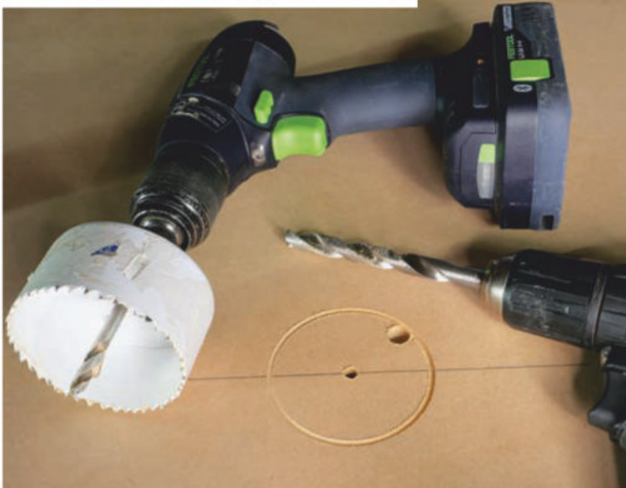
A 3" hole saw made quick work of cutting the pass-through hole in the upper shelf for the station's 2½" dust hose. Notice the 1/2"-diameter hole next to the hole saw's kerf; it provides a channel for dust to escape.
