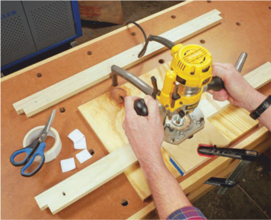
The author routed three elongated screw holes through the front top stretcher using a 3/16" straight bit and guide collar, run inside a shop-made template. These holes will allow for top panel wood movement.
