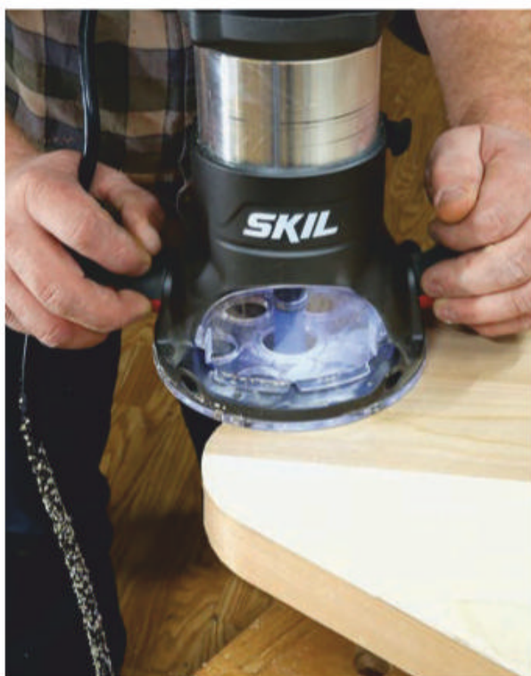
A flush-trim bit chucked into a handheld router was used to trim the chevron top flush to the edge of the tabletop.
