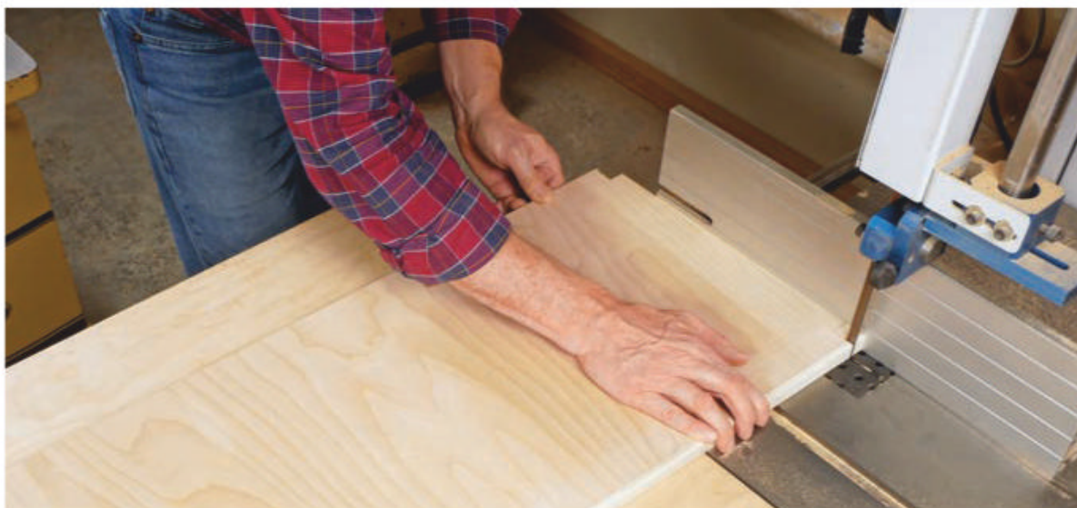
After the solid-wood edging piece is glued to the bottom panel, mark the four corners for leg notches and trim them to shape at the band saw or with a handheld jigsaw. Mark and make these cuts carefully — your accuracy here will show when the cabinet doors are opened.
