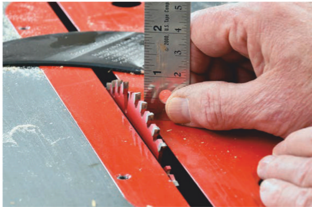
Set the blade height to match that of the desired cove cut. This is also a good time to remove your saw's riving knife.
