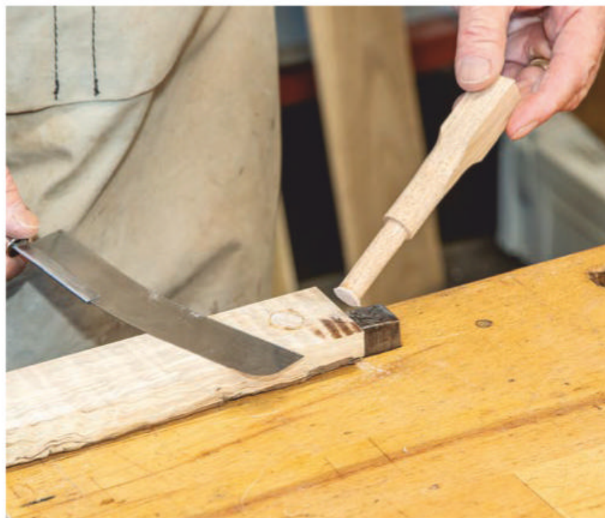
A Japanese flush-cut saw is not really a backsaw but belongs in every toolbox. This one (Rockler item 65231) is U.S.-made and trims dowels and such flush without marring the surrounding wood surface.
