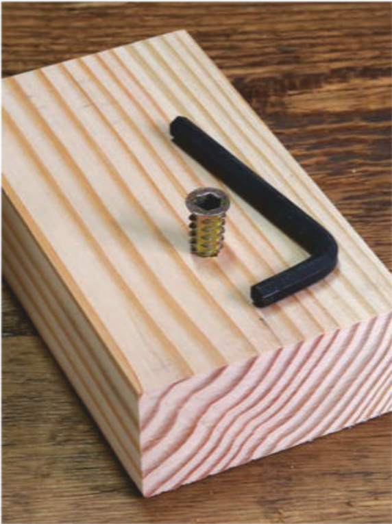
This tapered/flanged insert has a hex nut section above the internal threads. This detail and its tapered shape make it easy to twist in.
