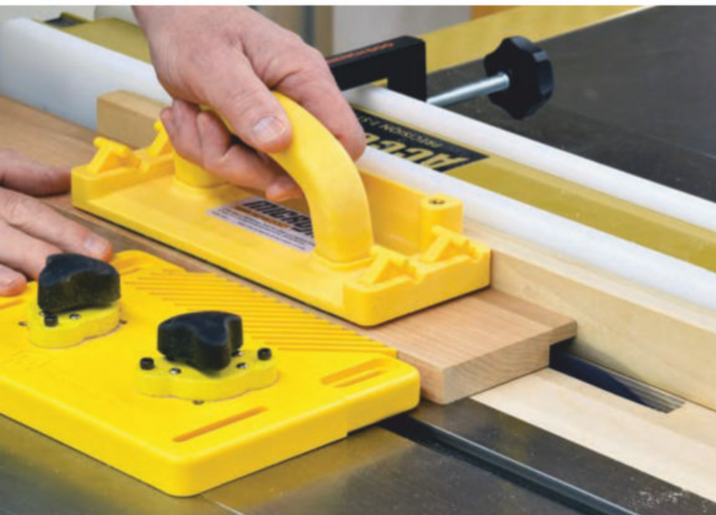
A rabbet cut made along the edge of a workpiece can be accomplished with the rip fence. Clamping on a sacrificial wooden fence protects the saw's standard factory fence facing.
