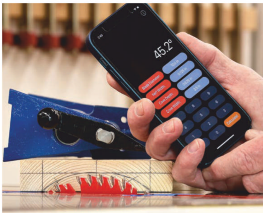
Sight over the table's top and adjust the workpiece angle until the blade's arc lines up with and exactly matches the one you've made in pencil. An angle-setting app or chart is another option.
