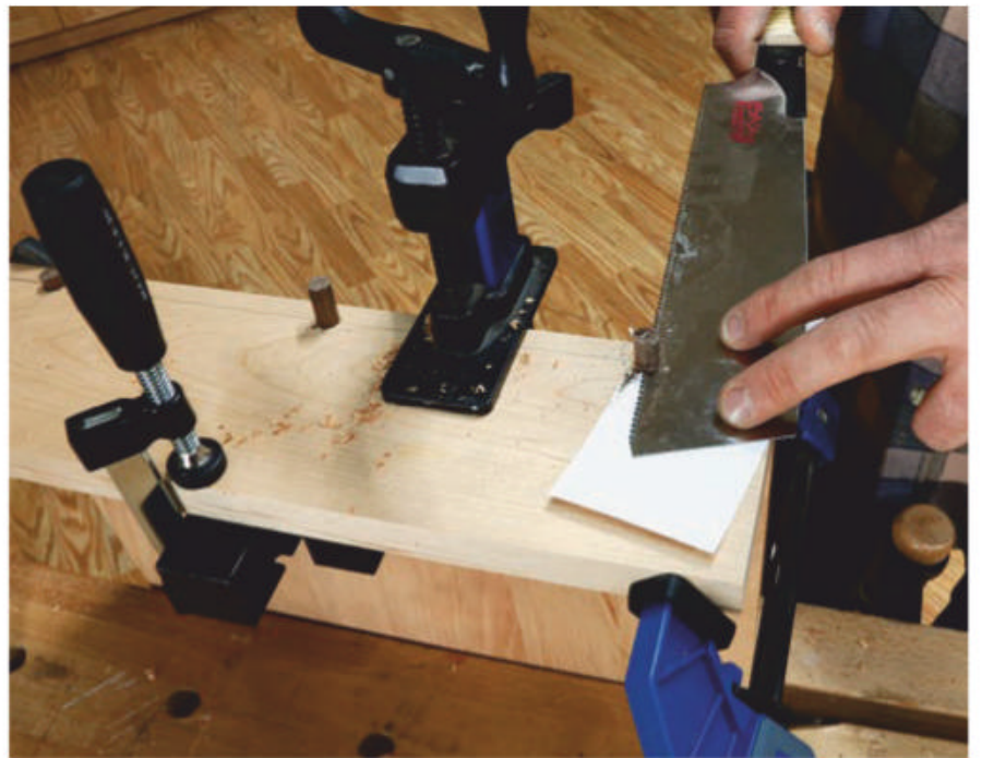
These walnut dowels make nice accents on the side of the cubby, but any species of dowel will work. Cut the dowels flush to the cubby sides with a handsaw, using a piece of paper as a shield to prevent saw marks.
