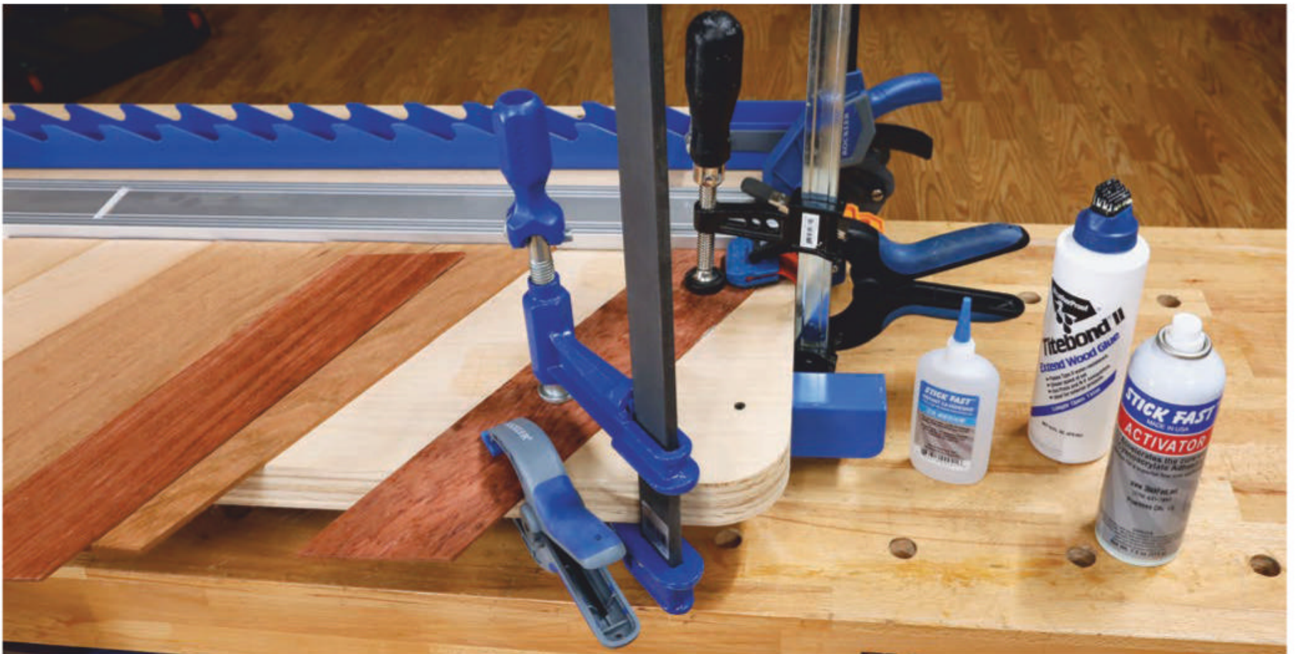
The very first chevron is secured to the plywood tabletop with a combination of CA and woodworking glue. Use an accelerator to speed the process up, but also use clamps to hold it down as it cures. This chevron will locate all the rest of them on one side of the table core.
