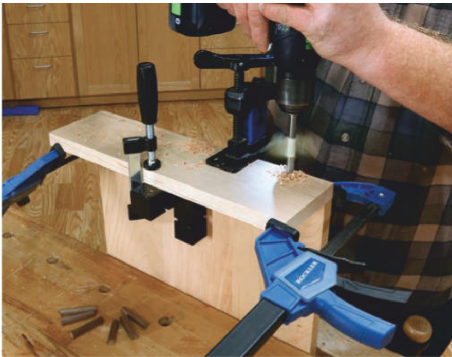
With the cubby sides clamped and glued to the cubby bottom, bore 3/8-diameter holes for the dowels. Put a small bit of glue in the holes and drive the dowels home. Allow the glue to cure.
