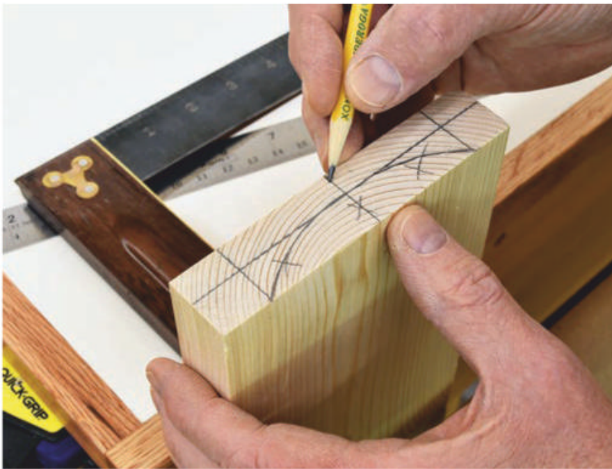
Pencil in the rough arc of your cove. A center mark and other registration markings will make it easier to sight-in the angle during setup.
