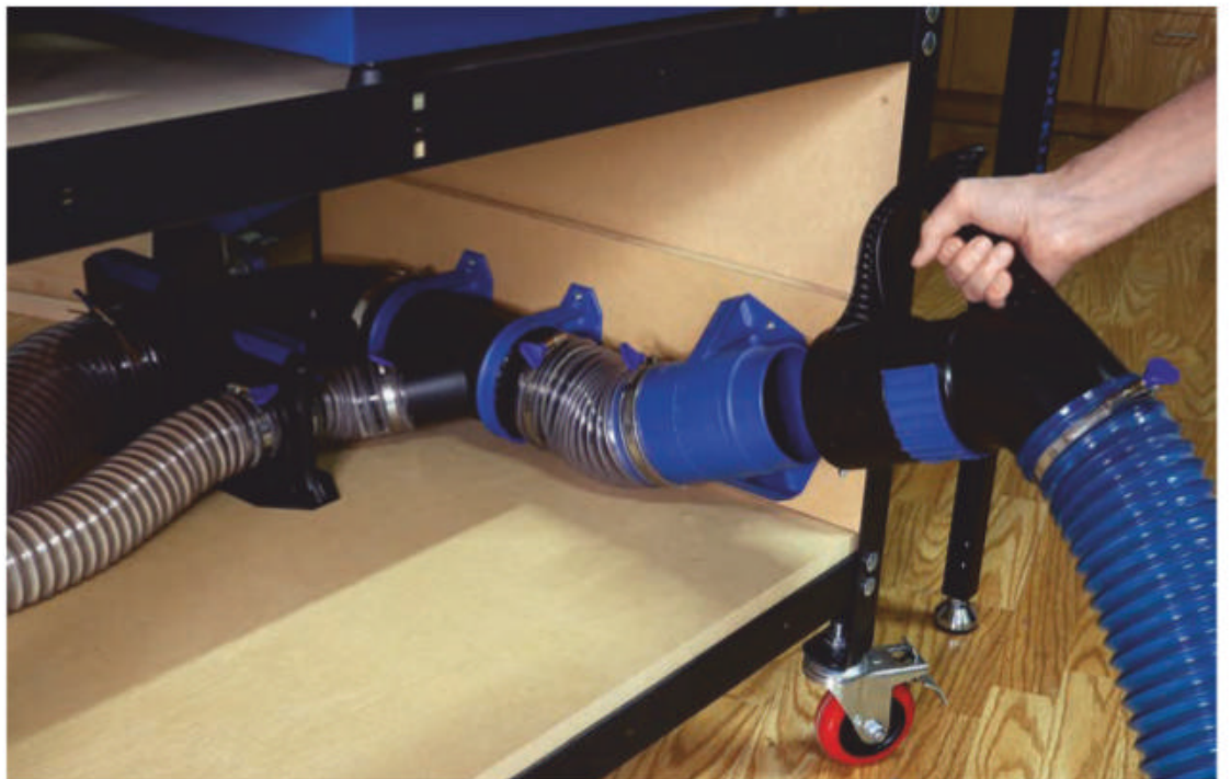
One of the author's goals for the dust collection system of this project is that it would be able to be connected to a single dust collector. Rockler's Quick Change Tool Handle friction-fits into the outer adapter on the trunk line to make dust collection quick, easy and tool-free.
