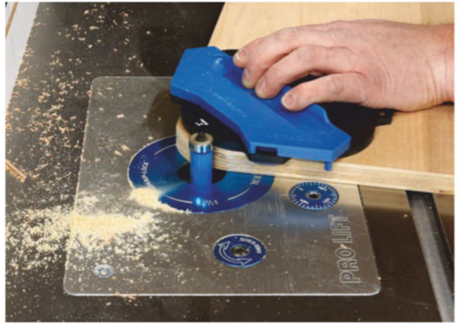
One of the benefits of using this template system from Rockler is that you can flush-trim the radius. For that reason, all four corners will be identical, which of course will give this project a refined appearance.
