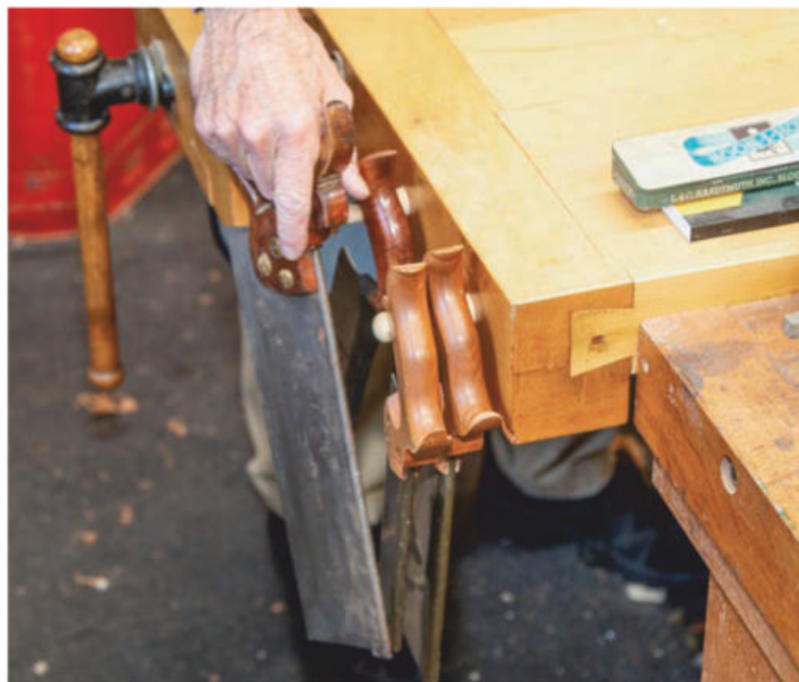
The author stows a variety of backsaws on pegs at the end of his workbench so they can be accessed quickly and conveniently. He finds them useful for a wide range of cutting tasks.
