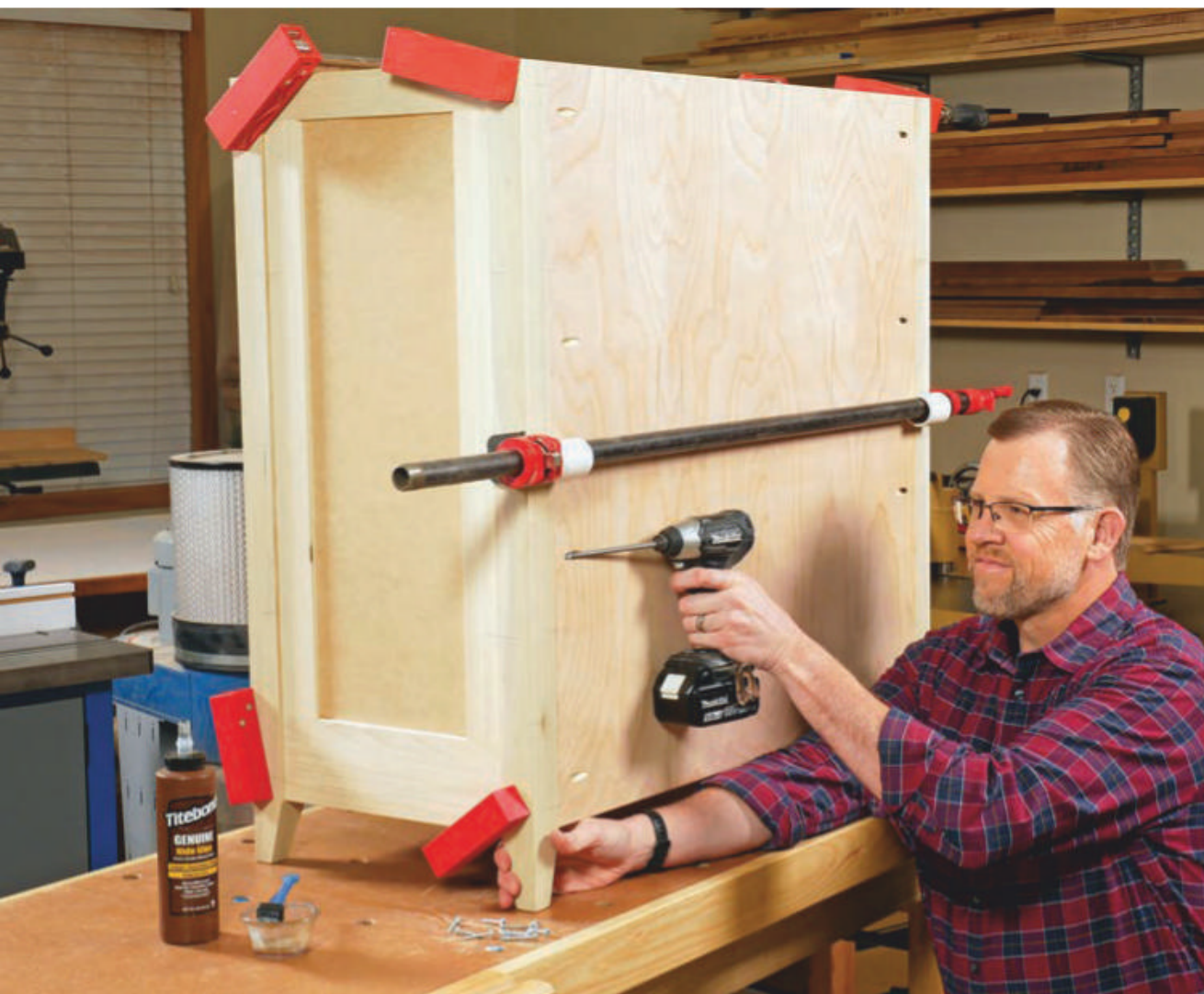
Assemble the side frames, front top and bottom rails and the back panel with glue to form the cabinet's carcass. Since plywood edges tend to soak up more glue than solid wood, the author reinforced the back panel joints with pocket screws to strengthen them.
