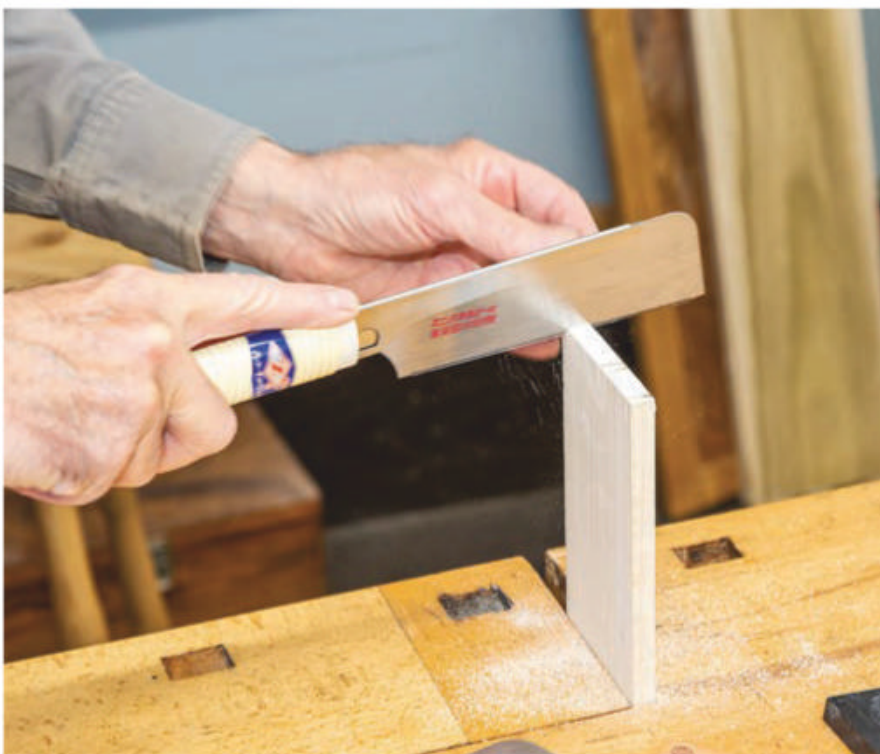
This Z-Saw dozuki saw (Rockler item 66376) only costs $30, and replacement blades are $20. It works very well. Replaceable blades mean that a woodworker does not need to have a dull saw sharpened.
