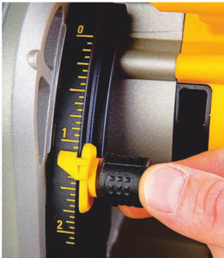
A spring-loaded cursor and scale make it easy to set track saws for depth-of-cut, particularly those on saws such as this DeWALT model that read in Imperial measurements.
