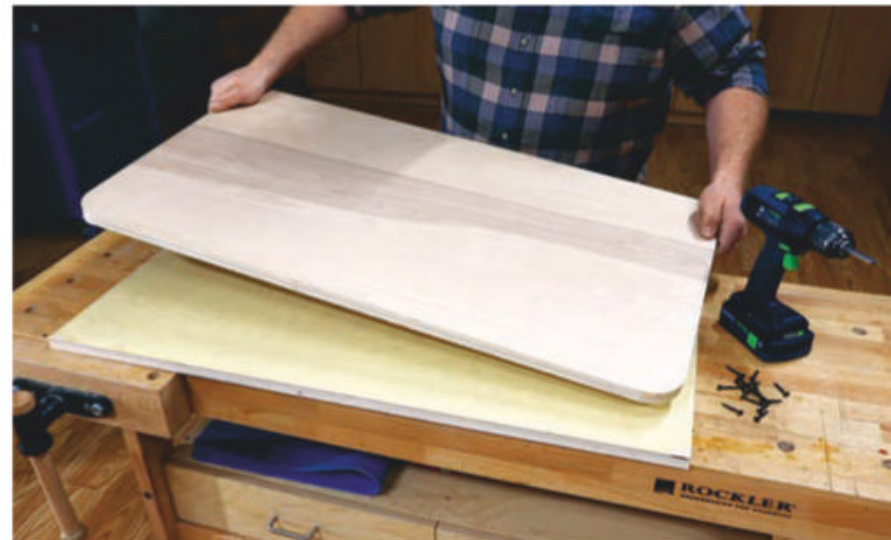
Gluing the two plywood pieces together can be a bit tricky as they tend to slide around. Use clamps across their width. There needs to be about a 1/4" overhang on both ends.
