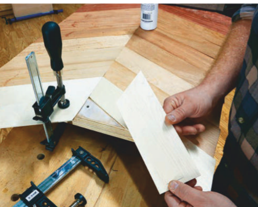
The last two small pieces of hardwood are fitted into the opening in the chevron pattern. Glue and clamp them in place and allow the glue time to cure.
