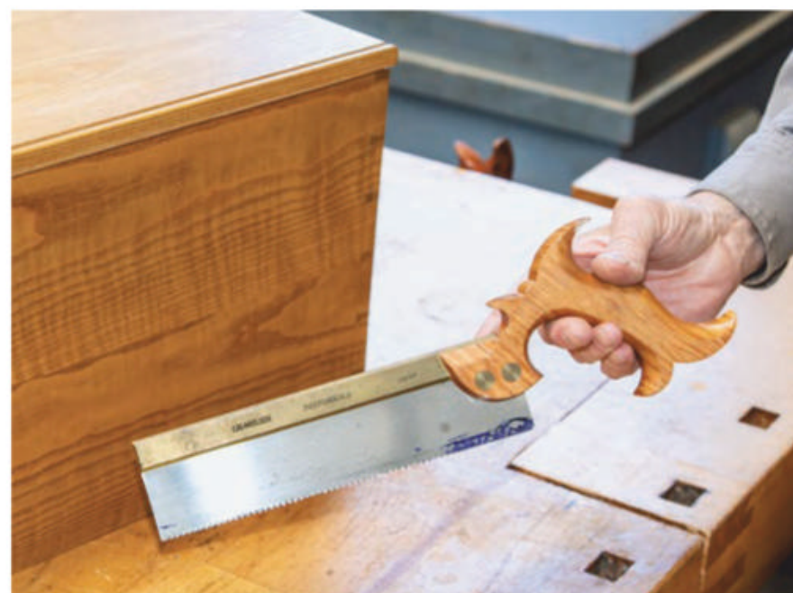
This 10" Independence 14-point rip-filed backsaw is a good choice for the dovetails in this larger chest. Backsaws have a metal or sometimes plastic spine on their back edge to stiffen the saw blade.
