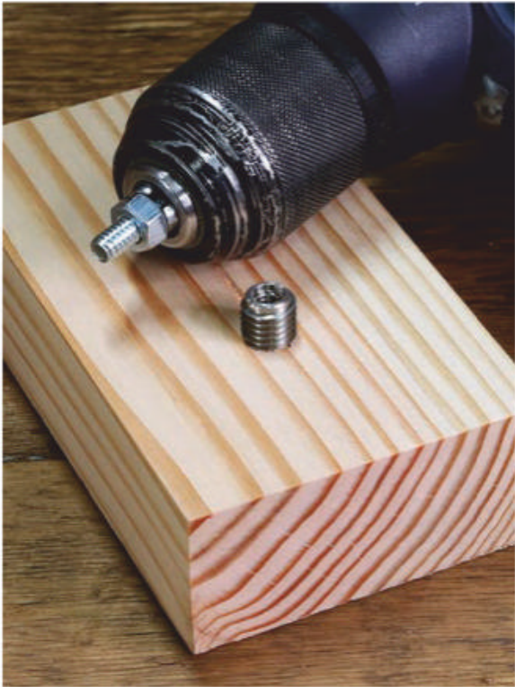
Another option: a threaded rod chucked into a drill, with a nut up against the chuck. Thread the insert onto the rod and use the drill to drive it in.
