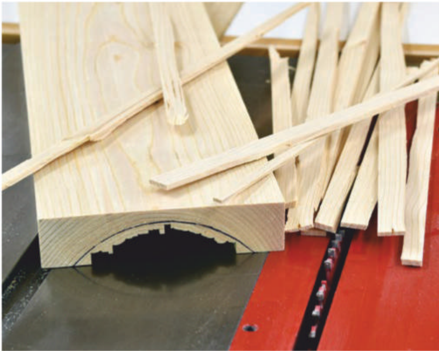
Coves create boatloads of dust. To minimize dust (and shorten cutting time), remove excess material before cutting the actual cove. Here, the author has made a series of straight rips and snapped out the waste.
