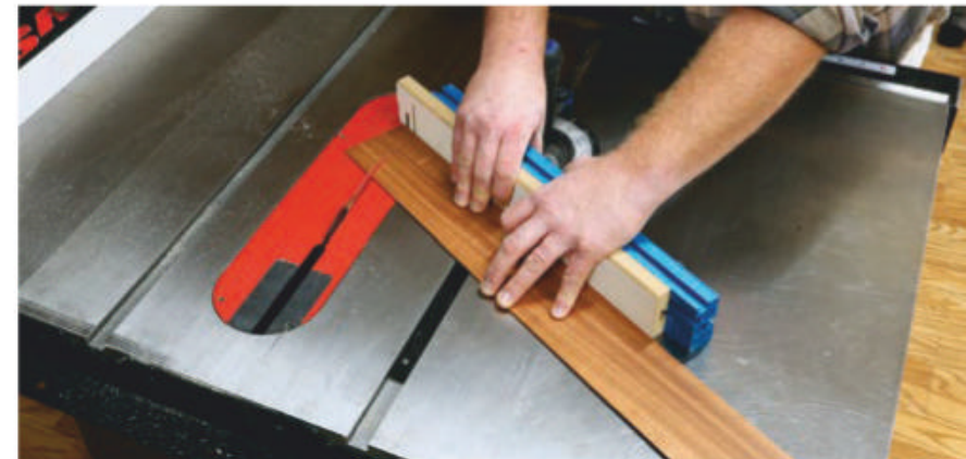
The key to successfully creating a chevron pattern is accurately cutting the widths of the pieces and the angle where they will be joined together.
