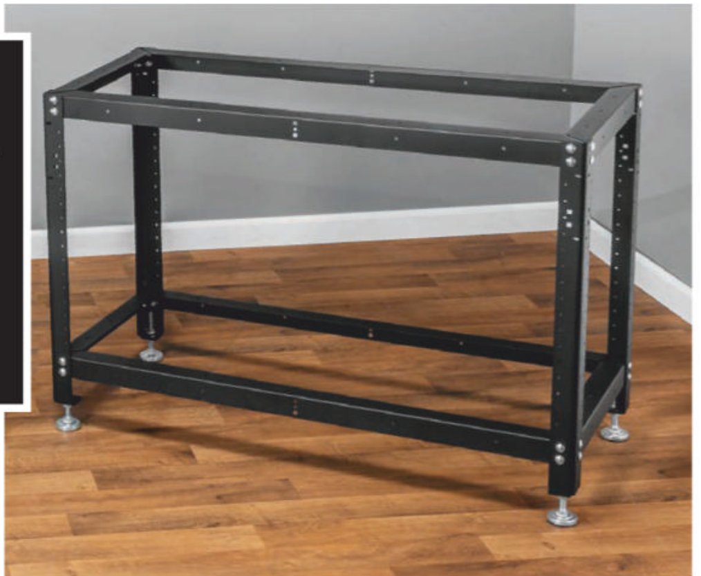
The framework of this sanding station is made up of Rockler's steel Rock-Steady legs and two sizes of stretchers. The author recommends using 4" casters (see inset) because their locking levers are easier to flip by foot than other smaller wheel options.
