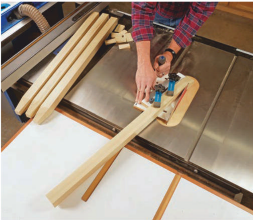
Rockler's Small Parts Taper Jig with integral hold-down clamps worked well to position and secure these leg blanks at a severe angle for cutting pairs of short tapers on each leg at the table saw.
