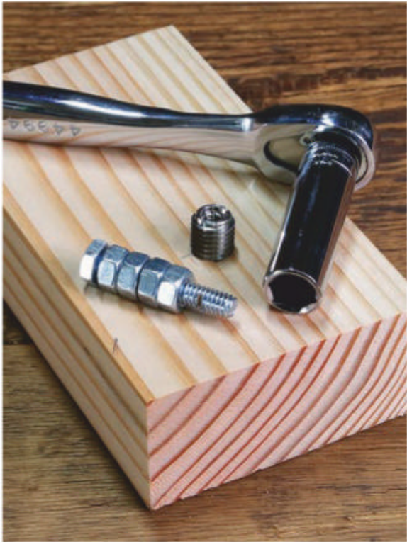
One way to install threaded inserts is to use a bolt with a few nuts on the shaft. Thread on the insert and wrench the insert into the wood.
