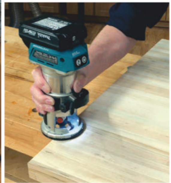
Sawing a 28" x 40" piece of Rockler's butcher block worktop in half creates a section of tabletop for a benchtop spindle sander and the top for a tip-down extension table at the end of the sanding station. The author eased the sharp edges and ends of these workpieces with a 1/8" roundover bit in a compact router.
