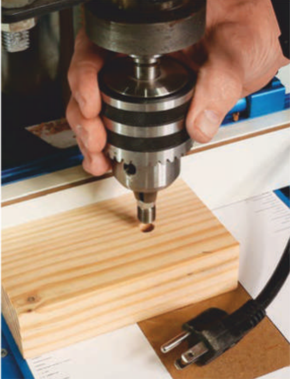
Hand-twisting the inserts in using a drill press and a threaded rod ensures that the insert will be driven in squarely to the surface of the wood.
