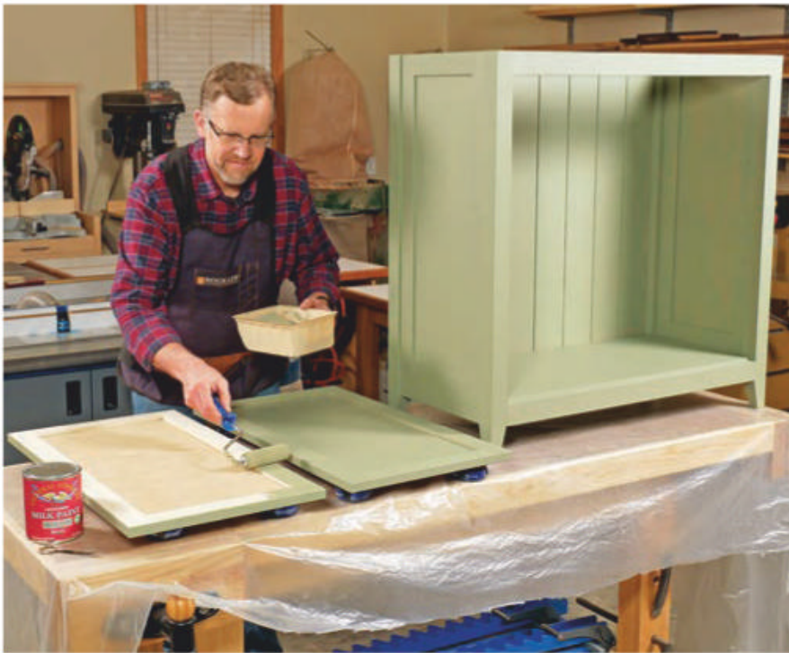
The durability, flat sheen and attractive colors of milk paint make it an appropriate choice for Shaker-inspired furniture. Apply two coats to the cabinet and doors with a brush and foam roller.
