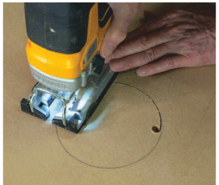
The author used a handheld jigsaw to cut a 5"-diameter hole through the upper shelf for the 4" dust hose to pass through. Here, a 1/2"-diameter clearance hole for the saw blade starts and ends the cut.
