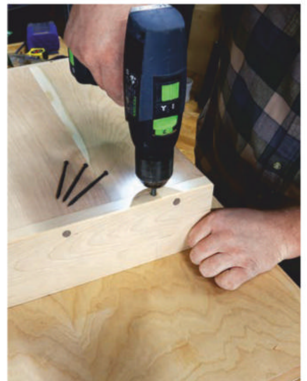
Boring holes for the trimhead screws is a three-step operation. The screws are seated inside the cubby sides where the 1/4" clearance hole stops. The screws hold the cubby tightly to the tabletop.
