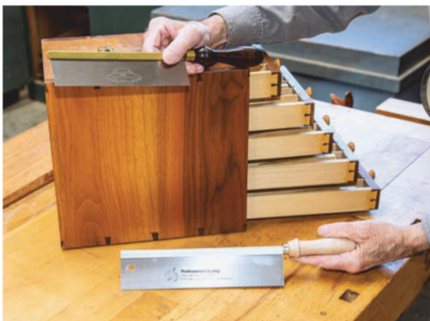
This 8" Crown 22-point rip-filed Gent's saw (Rockler item 98823) or the 8" Two Cherries gent's 14-point rip are both ideal for cutting the very small Empire dovetails in this case that the author built for his carving chisels.
