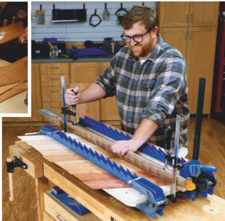
The very first chevron is secured to the plywood tabletop with a combination of CA and woodworking glue. Use an accelerator to speed the process up, but also use clamps to hold it down as it cures. This chevron will locate all the rest of them on one side of the table core.
