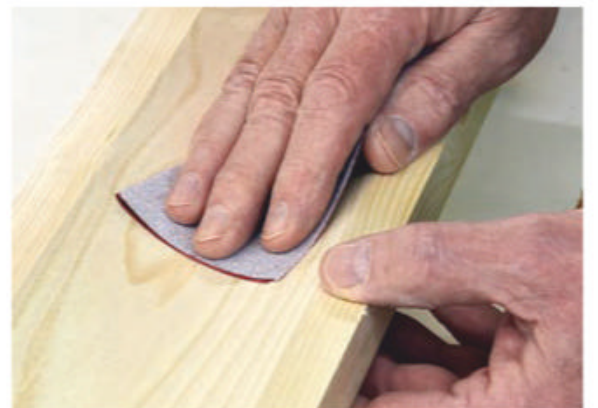
Once the cove is complete, sand off any "spiral" marks left by the saw blade.
