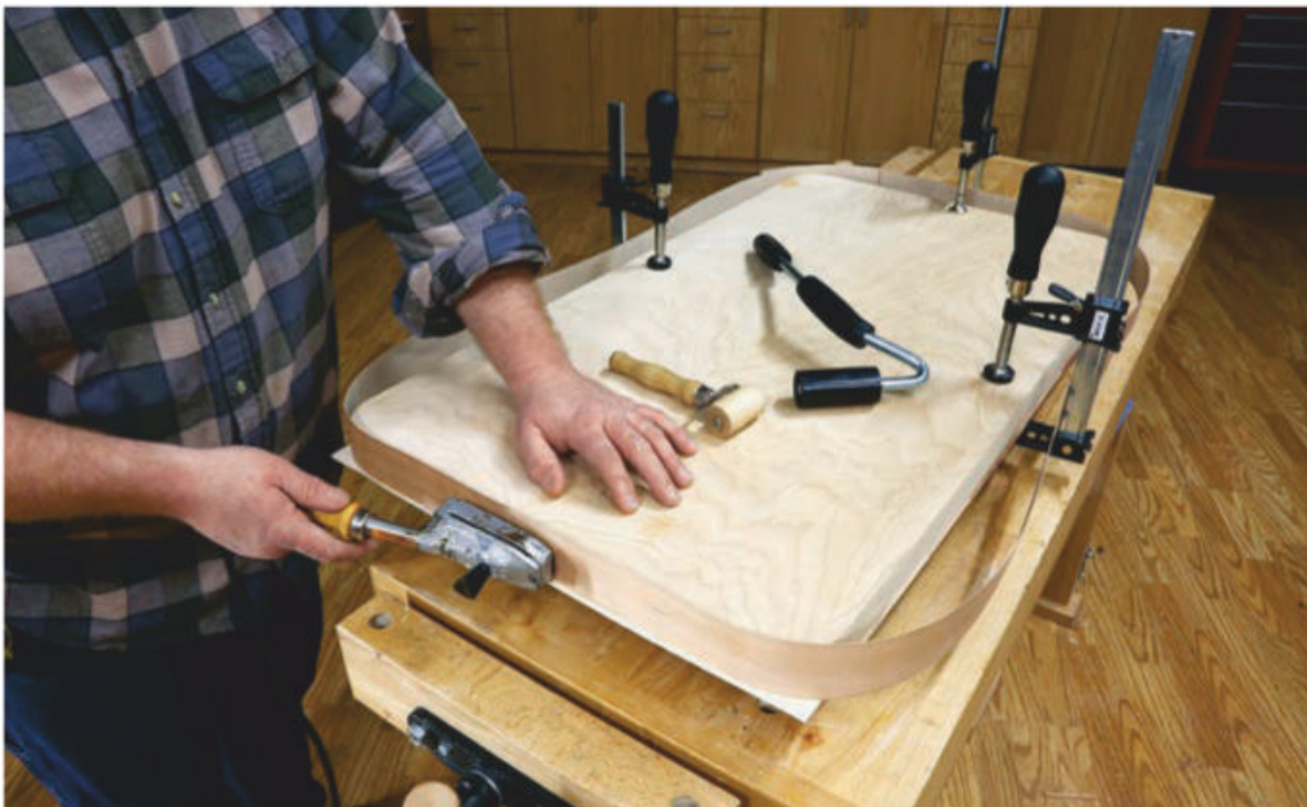
Attaching hot-melt edge banding to the tabletop core hides the plywood edges and creates a "hard-wood" looking edge underneath the chevrons.
