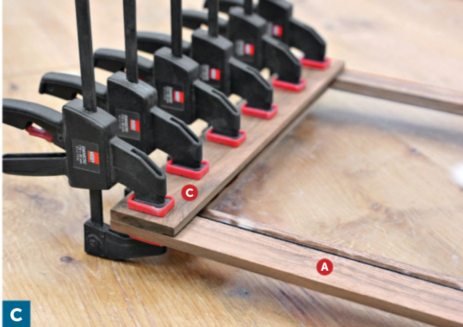
When gluing the retainers (C, D) to the frame, avoid any glue squeeze-out in the shallow rabbet. These rabbets will create a groove for the artwork.
