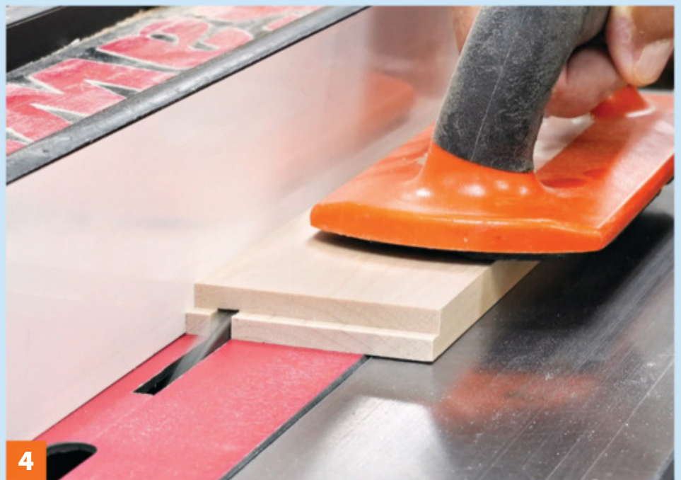
4 Cut the \frac{1}{4} "-deep groove for the drawer bottom on the inside face of each drawer front, back, and side. A push pad helps apply even pressure throughout the cut.
