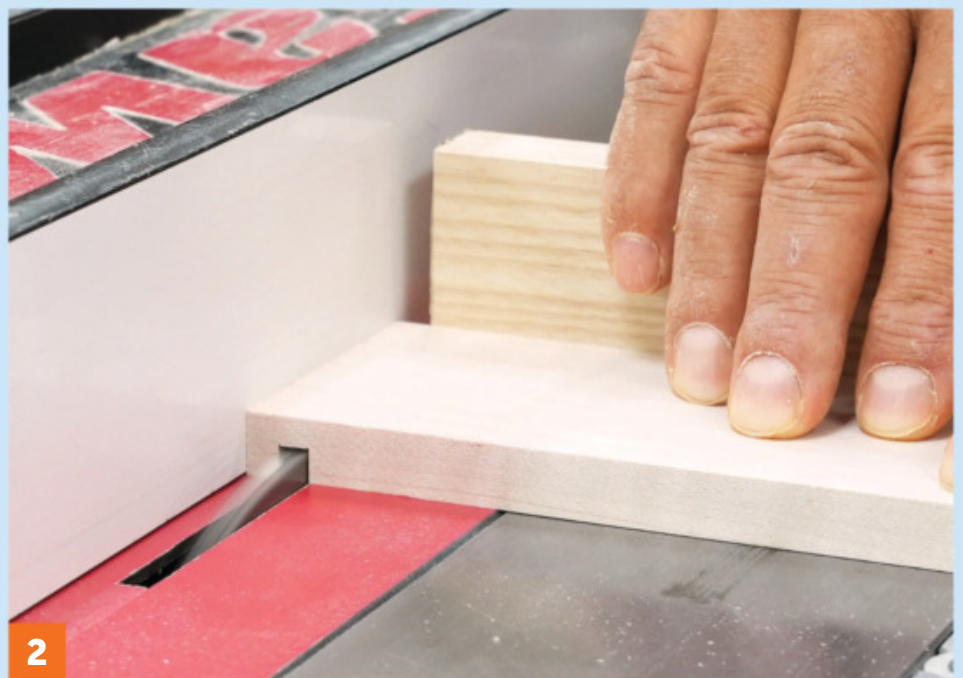
2 Attach an auxiliary fence to your miter gauge to steady the drawer side and prevent chip-out when the blade exits the workpiece. Butt the drawer side against the rip fence and make the cut.
