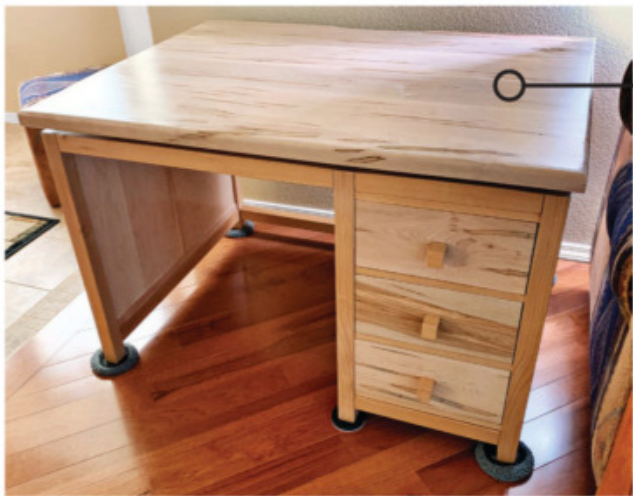
• JEFF KOWELL of Colorado Springs, Colorado, designed and built this desk for his daughter, incorporating an alder frame with wormy maple top and drawer fronts. Having designed this project from scratch, he considers it a turning point in his woodworking.
