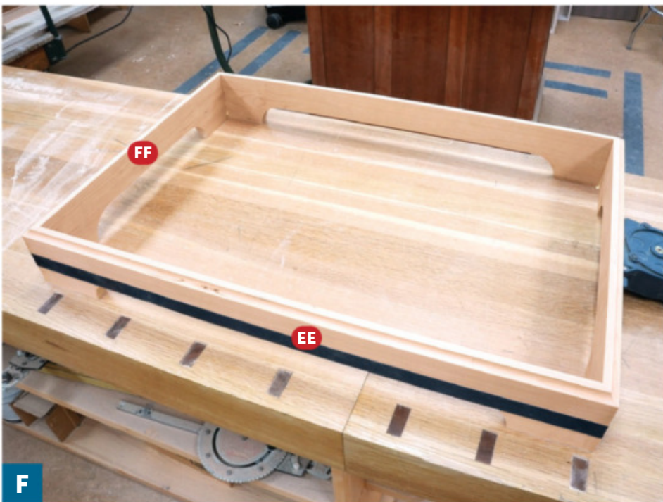
A biscuit in each beveled corner helps keep the corners aligned as you tighten a band clamp around the aprons. Check for gaps at each corner and ensure the assembly is square.
