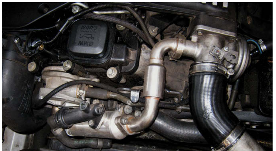
A complete EGR system, as seen on an E46 320d BMW. In this case, the exhaust gas passes through a gas-to-water cooler (cylindrical gadget in the middle) before going through the vacuum-operated valve (to the right) into the engine's air intake.
