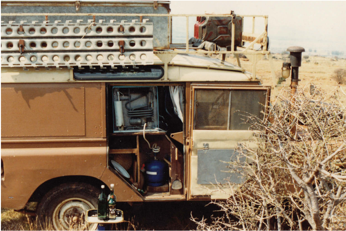
Interior sliding locks were fitted to all the doors. Notice the glass dirt-trap on the snorkel tower.
