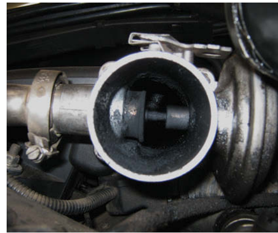
Typical inside view of a working EGR valve: some deposits near the valve, but not enough to impair air flow. Modern engines don't appear to suffer as-severe gunk deposits, mostly thanks to the addition of EGR coolers, which reduce the reaction between the hot exhaust gas and the crankcase breather vapours.
