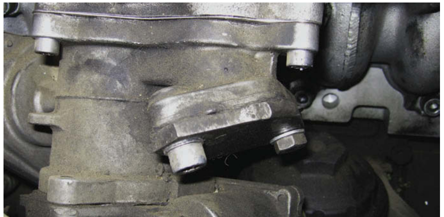
A home-made EGR delete: a simple blanking plate bolted to the air intake side of the EGR system. This VW diesel's ECU did, however, complain about insufficient EGR flow, which is why it was caught standing in a workshop...
