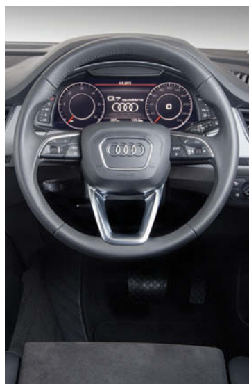
Far left The ZF-sourced, torque converter automatic can be controlled by paddles on the steering or in sport mode on the gear lever. Above left and below Audi's 'Virtual cockpit' is a first of its kind in the motor industry and after some time getting used to it, works brilliantly.
