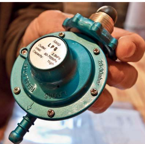
SIGNS OF THE TIMES. A gas regulator must have certain info printed on it, such as the outlet pressure and direction of the gas flow.
