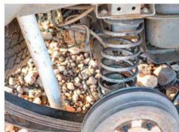
TILL HERE AND NO FURTHER. The previous owner had two additional leaf springs fitted to the KB, but whoever installed it had failed to properly secure it with longer U-bolts.
