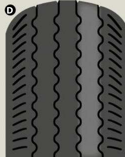
BAD WHEEL ALIGNMENT
