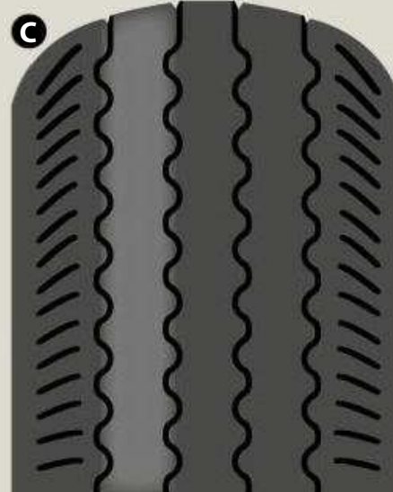
BAD WHEEL ALIGNMENT
