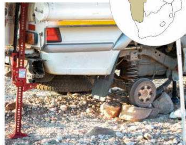
TILL HERE AND NO FURTHER. The previous owner had two additional leaf springs fitted to the KB, but whoever installed it had failed to properly secure it with longer U-bolts.
