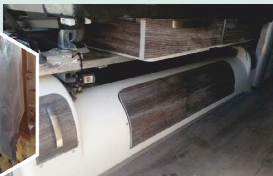
SPECIAL COATING Anton's Iveco received a special layer of paint called Raptor coating – essentially more scuff and rust resistant than ordinary paint.
