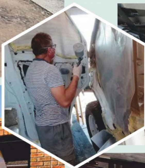
SPECIAL COATING Anton's Iveco received a special layer of paint called Raptor coating – essentially more scuff and rust resistant than ordinary paint.
