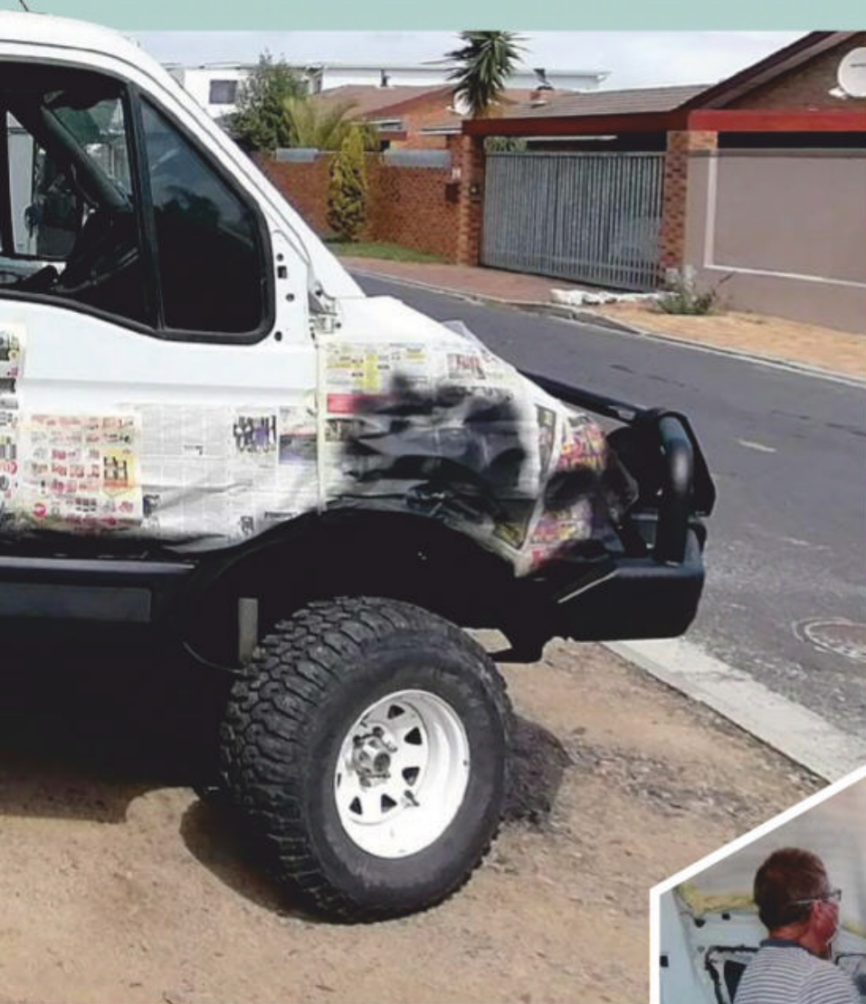
SPECIAL COATING Anton's Iveco received a special layer of paint called Raptor coating – essentially more scuff and rust resistant than ordinary paint.
