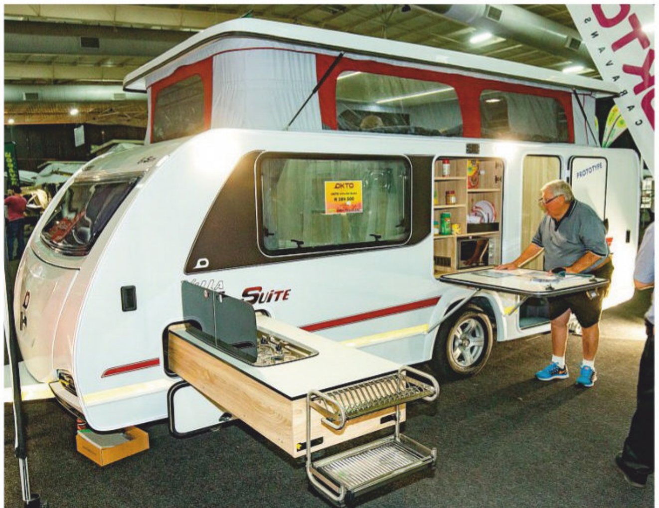
ROUGH STUFF The Gravellor's 15" wheels, tread plate and bull bar better prepares the caravan for dirt roads.
