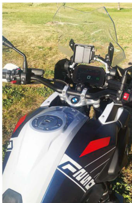
SMART BIKE. The Trophy comes with a pre-installed mount (below left) for a BMW-branded GPS which can be operated with a wheel next to the left grip (bottom right). The 'clocks' provide access to a lot of bike systems (below).
