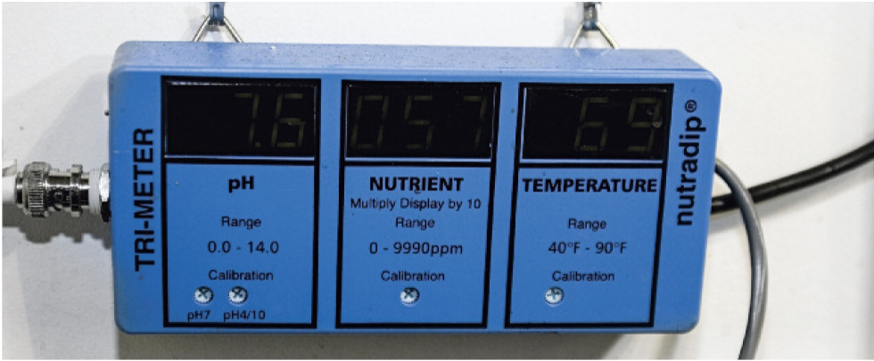
A monitor that keeps track of pH fluctuation, nutrient PPM, and reservoir temperature.
