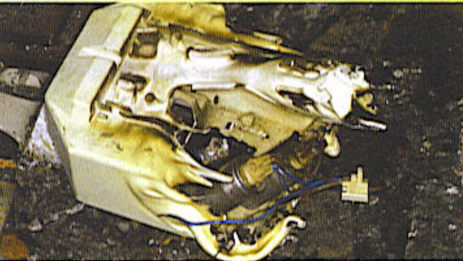
Avoid scenes like this, and never operate lamps on an overloaded circuit.
