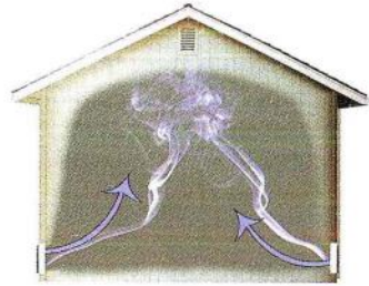
Ratio = 1:4 – four times more air exits than enters the room
