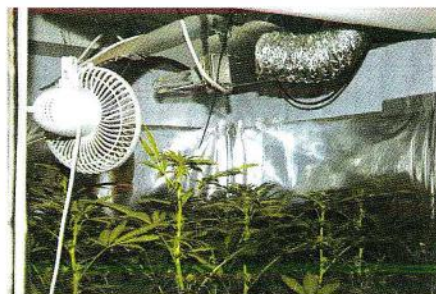
Fan mounted with bungee cords
