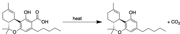
FIGURE 3.2 Decarboxylation reaction of THCA to THC.
