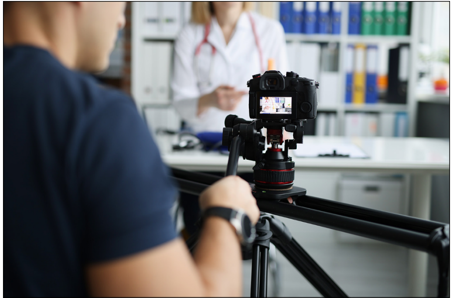
FIGURE 5-7: Sliders move cameras back and forth on rails.
