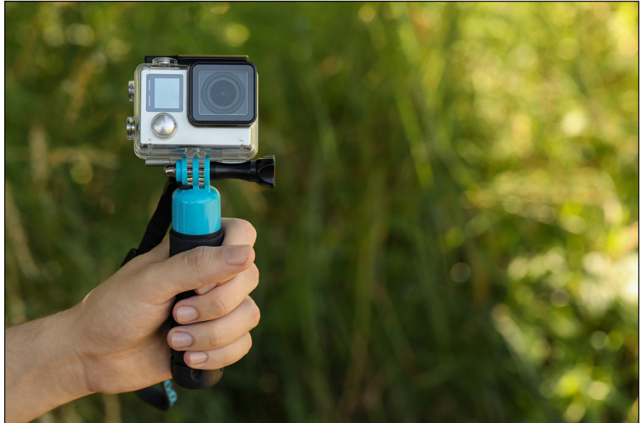
FIGURE 5-4: Monopods are typically less steady but more convenient than tripods.
