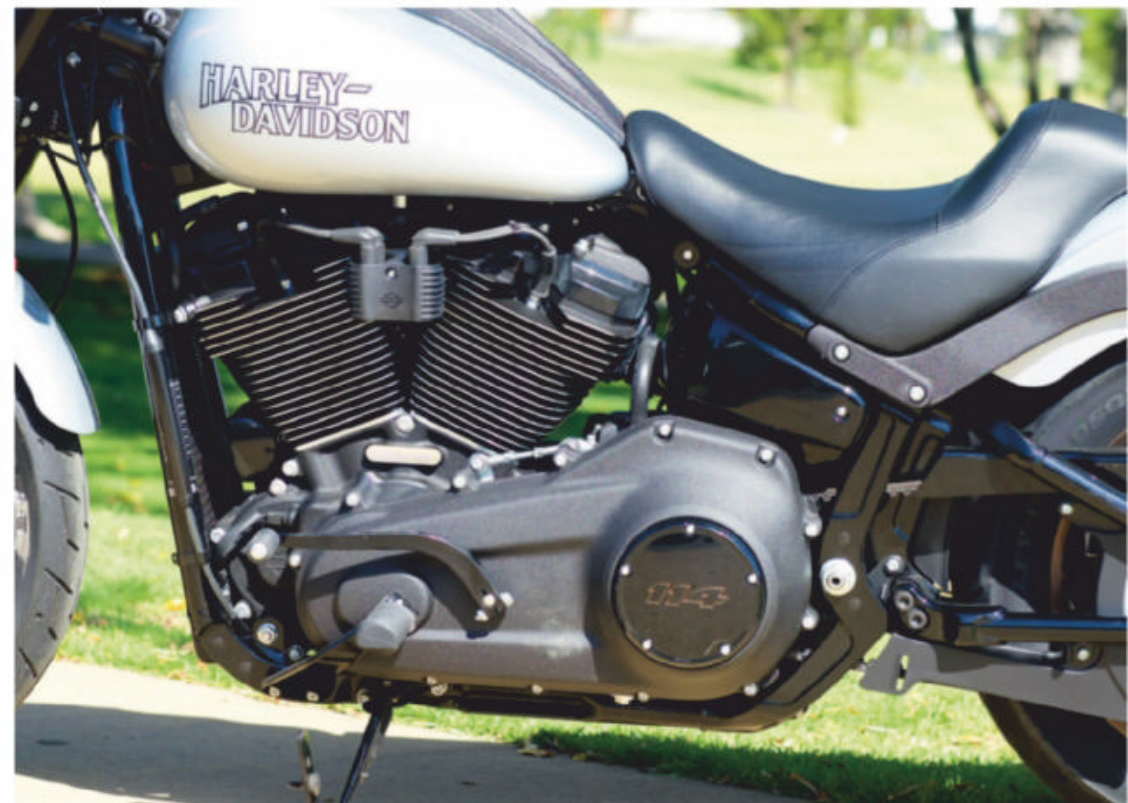
Mid-set controls aid cornering clearance.
