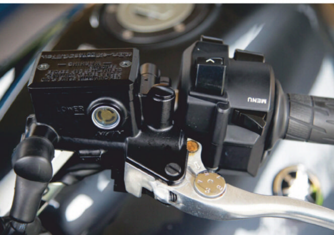
Out of fashion but very good to use hydraulic clutch with adjustable lever.
