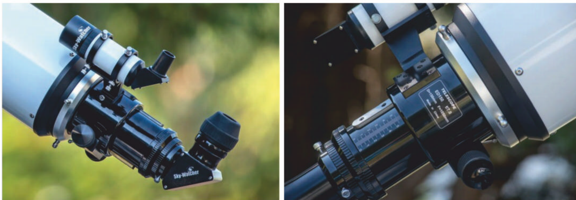
▲ Left: The telescope's solid 3.4-inch rack-and-pinion focuser and mounted 8×50 right-angle finderscope are rotatable by loosening the large metallic 'captain's wheel' ring with machined spokes. Right: A millimetre scale to aid in repeating focus positions is printed on the focuser drawtube. Also visible is the 10:1 fine-focus knob.
