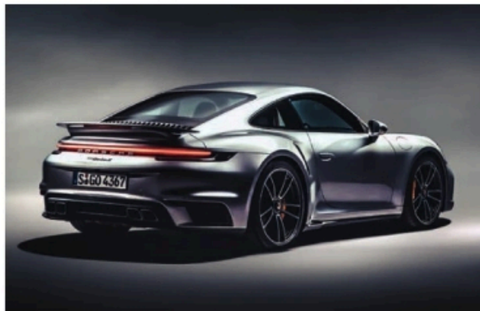
Rear wing and diffuser help boost downforce by up to 15% and brakes are carbon-ceramic as standard
