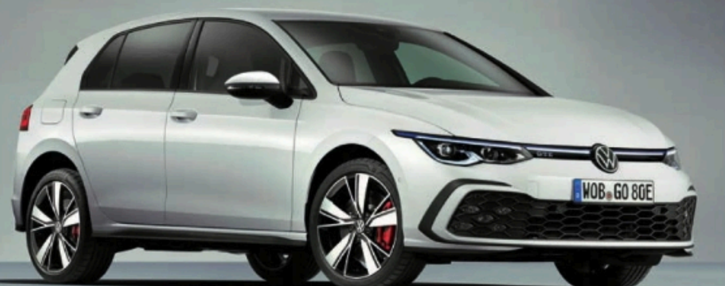
GTE marries a 1.5-litre turbo petrol engine to an electric motor
