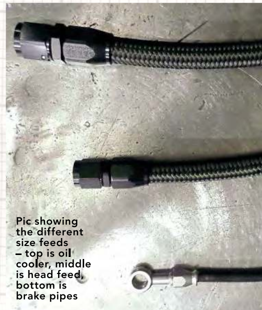
New head oil-feed pipe, and old one for comparison
