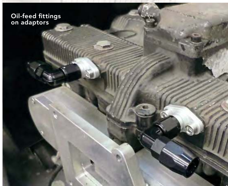
Head oil-feed pipe lower part and new replacement parts
