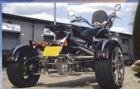
Honda Valkyrie / F6C shaft drive with Polished Stainless Steel cradle, Reverse gearbox.
