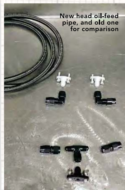
Pic showing the different size feeds – top is oil cooler, middle is head feed, bottom is brake pipes
