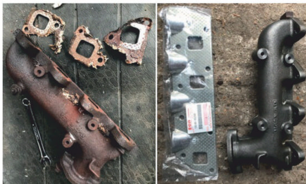
Old (left) and new manifold and gasket provide quite a contrast. Top left: all back in place
