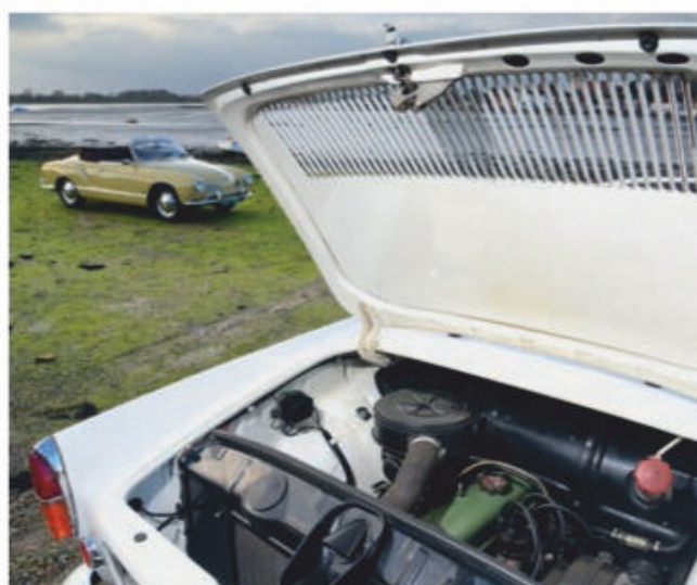
Tidy and tiny 956cc four-cylinder is less torquey of the two
