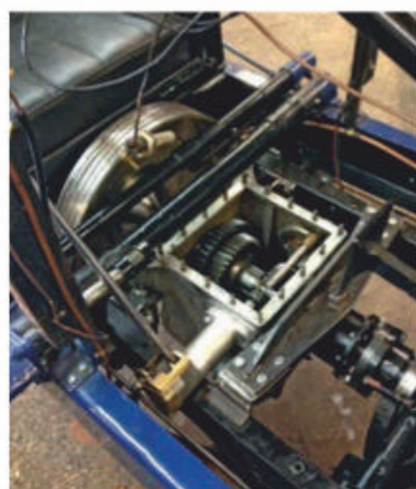
The Sunbeam's new gearbox (left); the 350HP with Malcolm Campbell at Pendine in period
