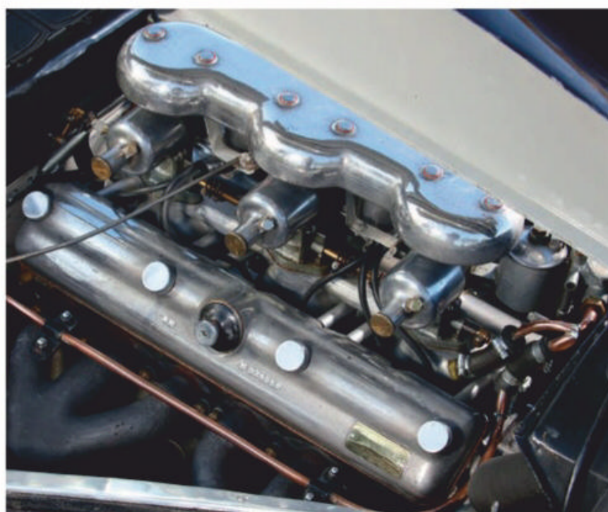
Three SU carburetors feed the 2-litre straight-six. Above: period toolbox remains in the boot
