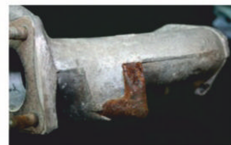
Old manifold's rusty elbow sprang a leak
