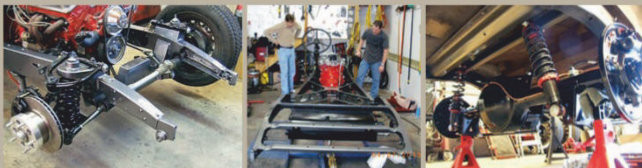
Second restoration involved rather more extreme works, and getting everything positioned perfectly took skilled craftsmanship. Ubiquitous hot-rod parts include Mustang II front end, smallblock Chevy V8 and '70s Ford 9in rear
