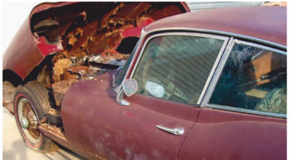
Damage was extensive to the left-hand-drive E-type, with most body panels very corroded
