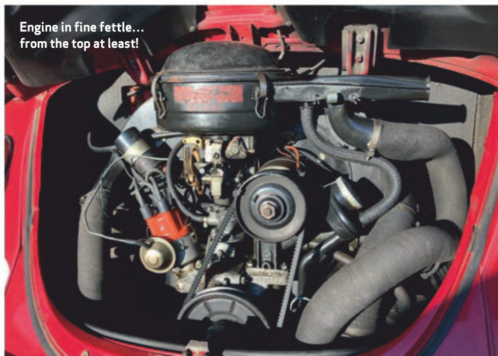
Split section of air-cleaner intake cut off
