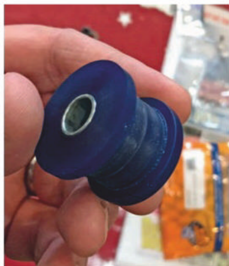
Filed to size, linkage bushes fit perfectly
