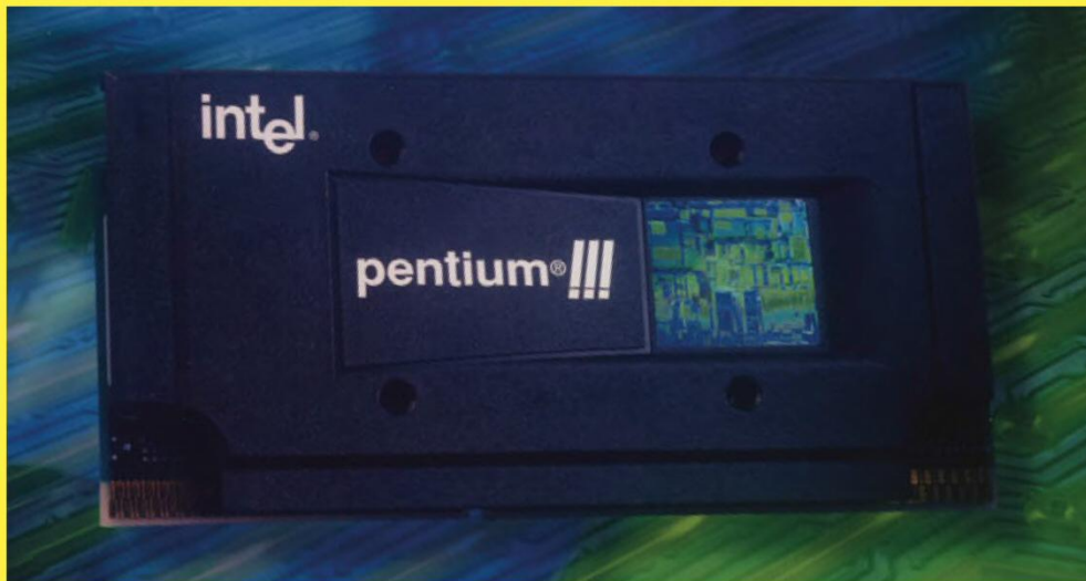
The Pentium III maintained the front with the hologram, but used the new SECC2 packaging, which left the circuitboard bare at the back
