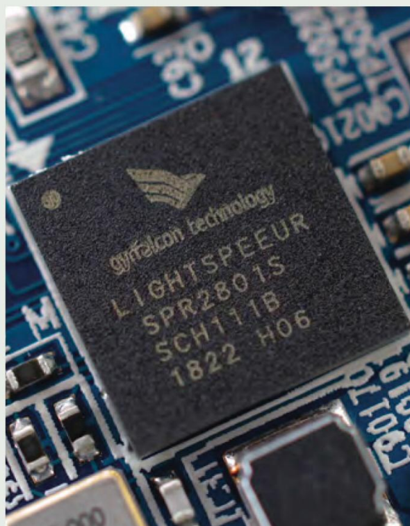
The Lightspeeur NPU is designed to accelerate neural network workloads at a very low power draw
