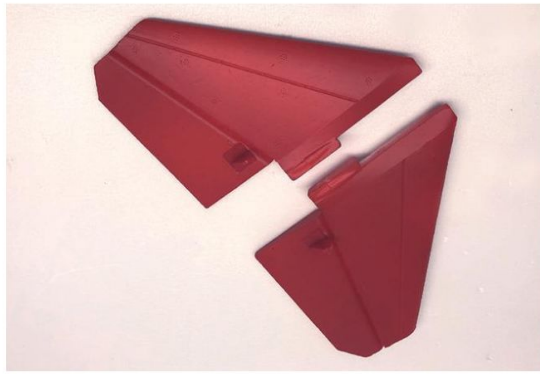
Horizontal stabilizer/elevator assemblies prior to attachment to fuselage. They have molded-in hinges.
