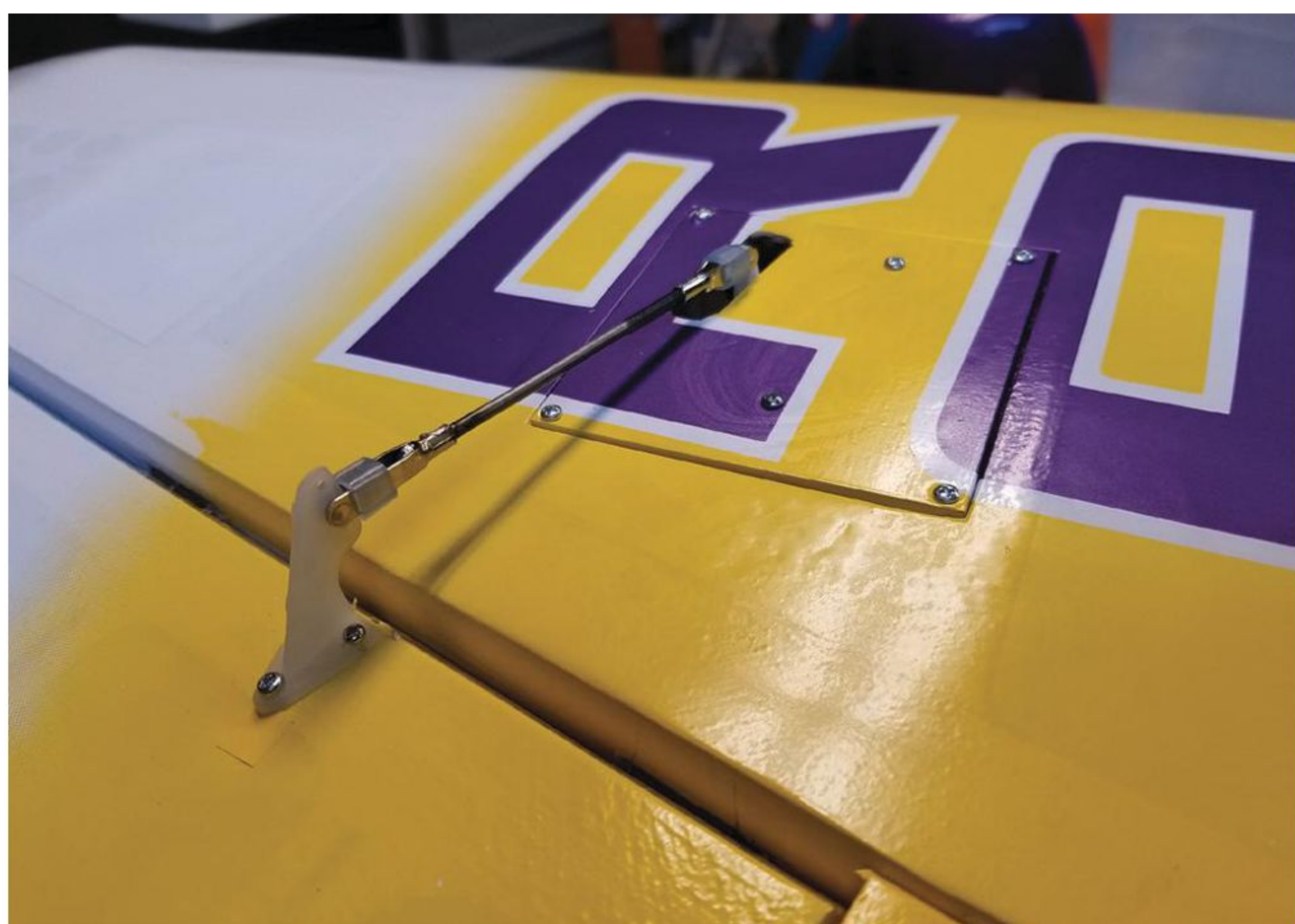
The aileron and flap servos are installed under flush-fitting hatches on the underside of the wing panels.
