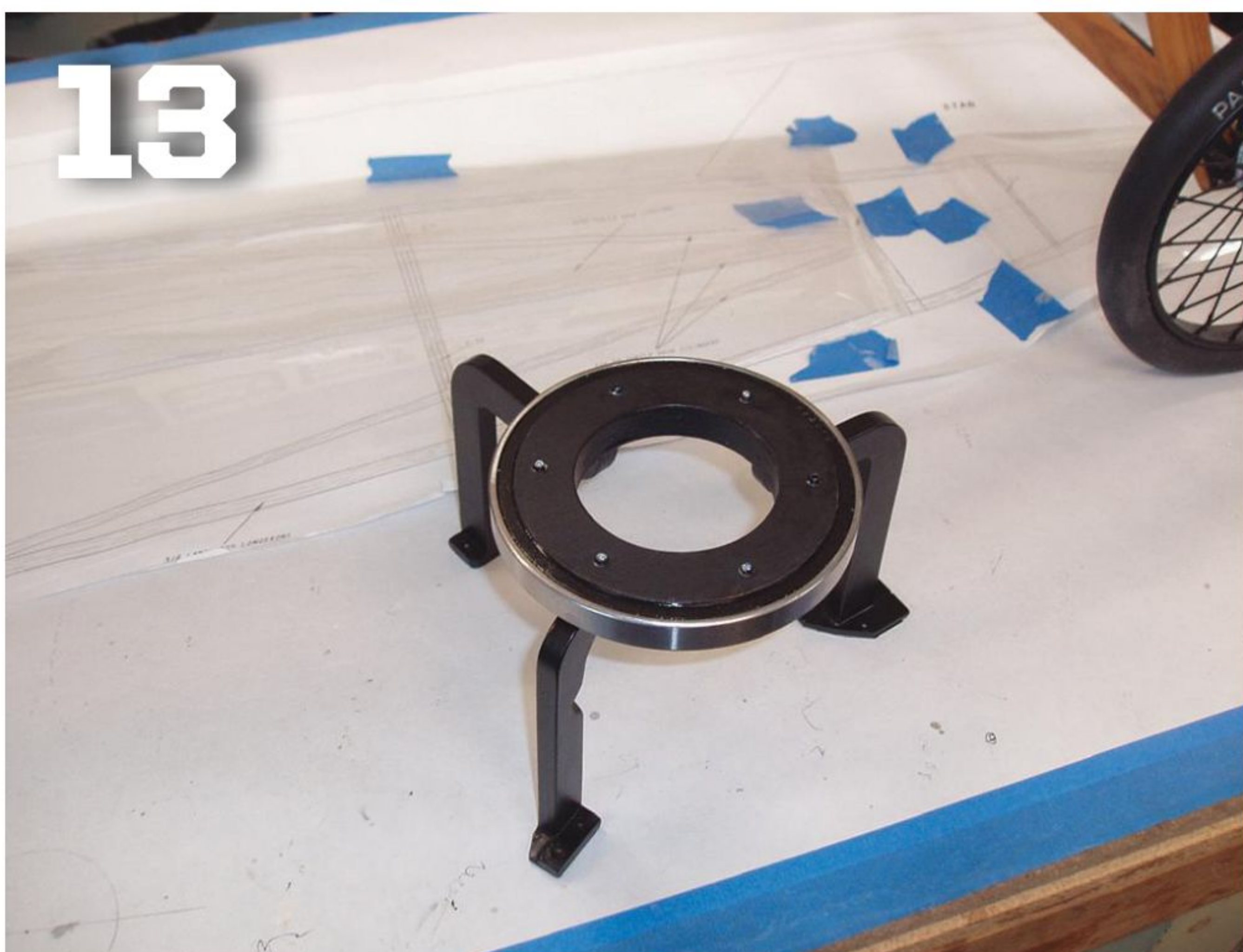
13 This funny little thing is the attachment mount for the dummy engine, with the bearing installed. The awkward leg design is necessary to fit around the DLE engine. Made of plywood, the legs fasten securely to the firewall with screws.
