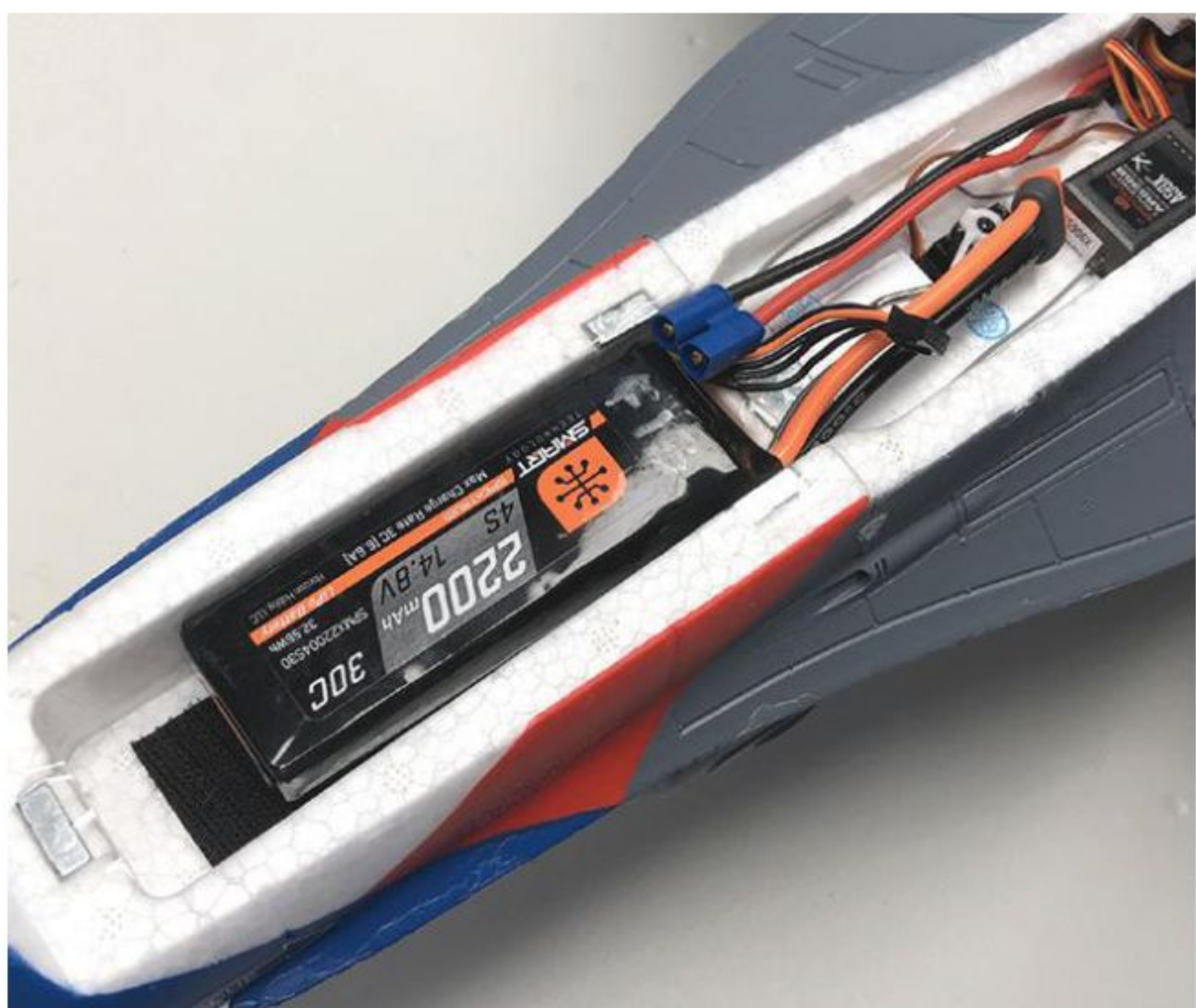
Battery compartment with canopy hatch removed. I used a Smart Technology 4S 2200mAh pack and the pre-installed Spektrum AR636B receiver.
