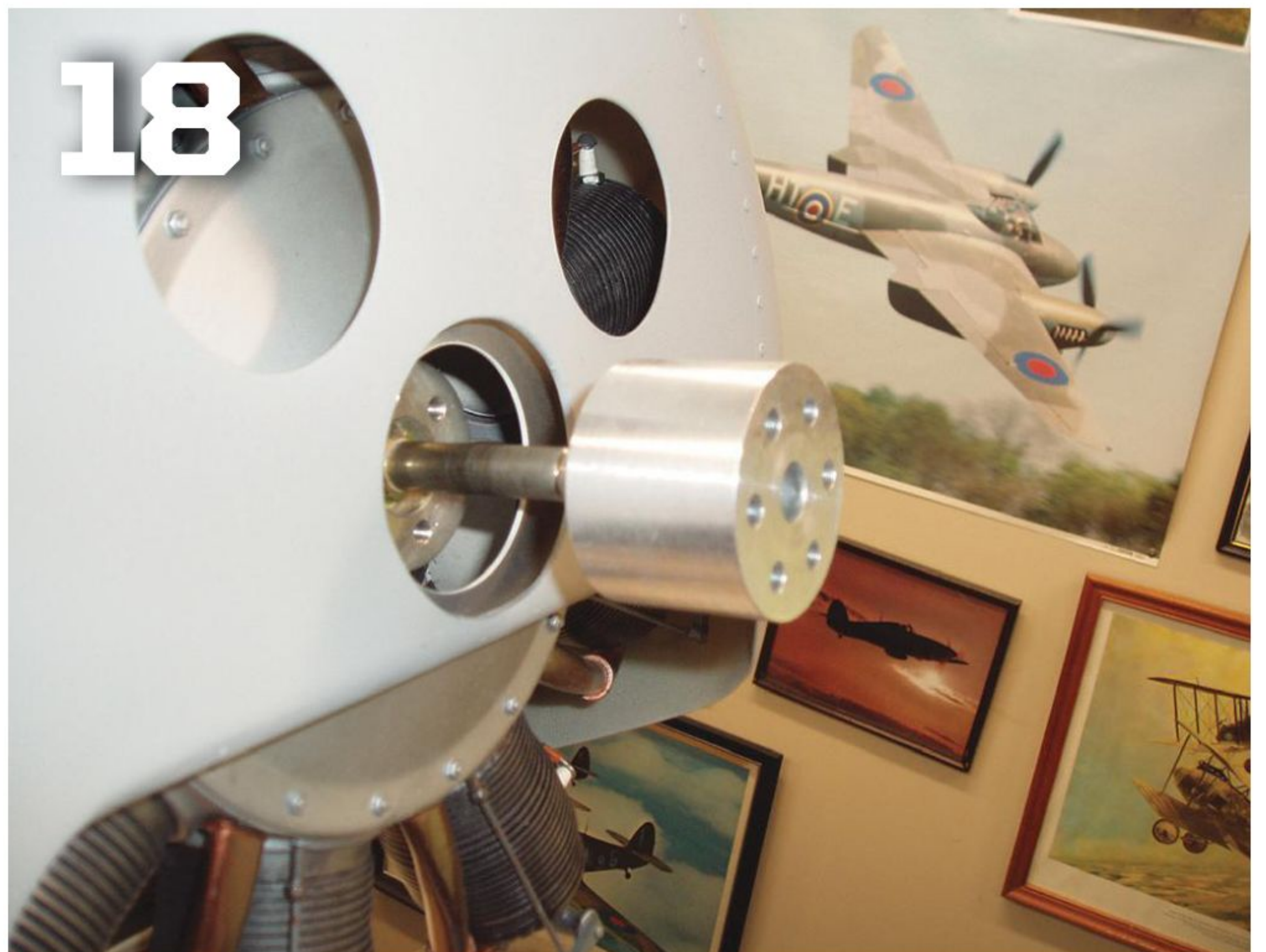
Here is the 1 1/4-inch shaft extension necessary to get the prop clear of the cowl.
