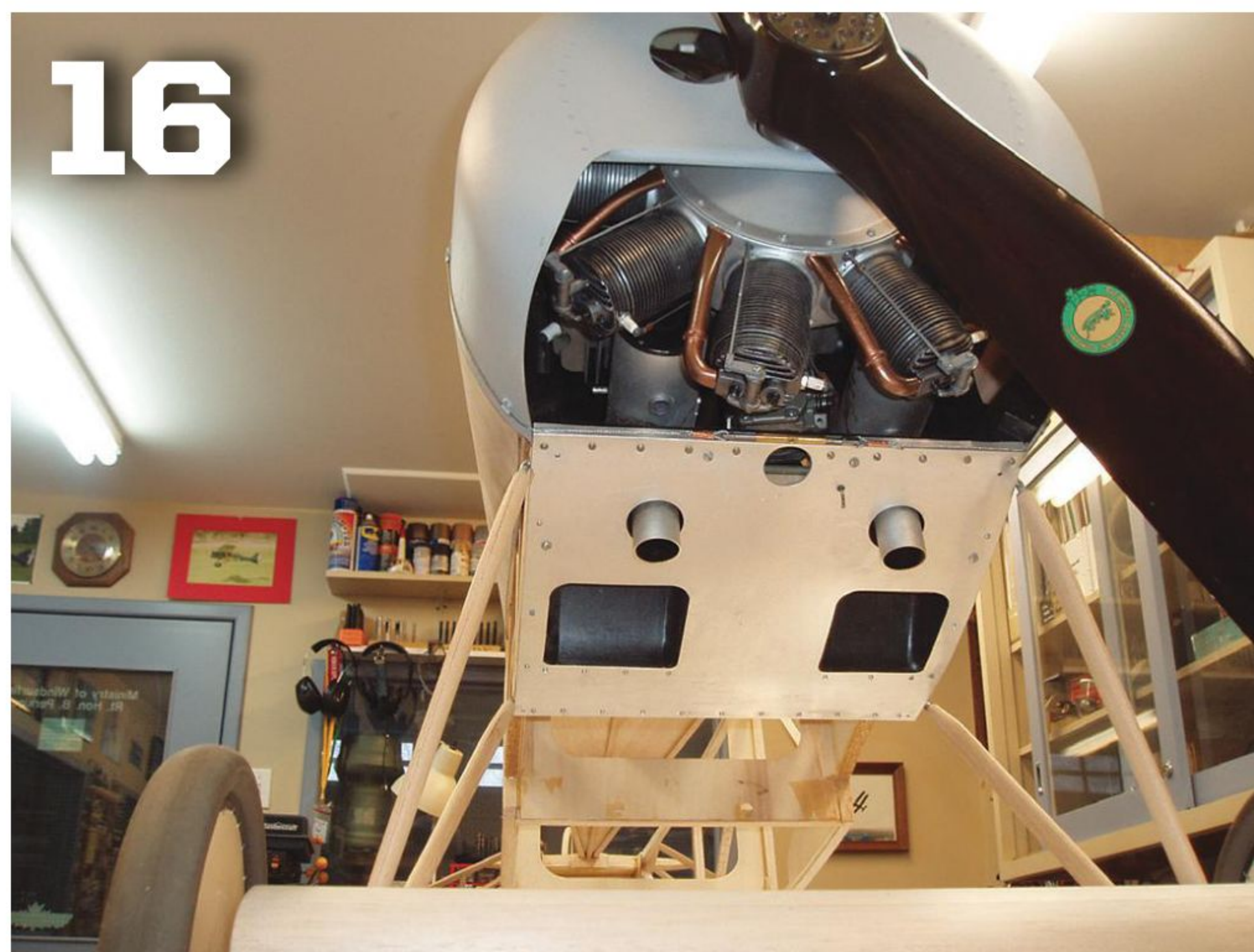
16 This view shows the cooling air and exhaust outlets on the underside. The dummy engine spins quite freely!
