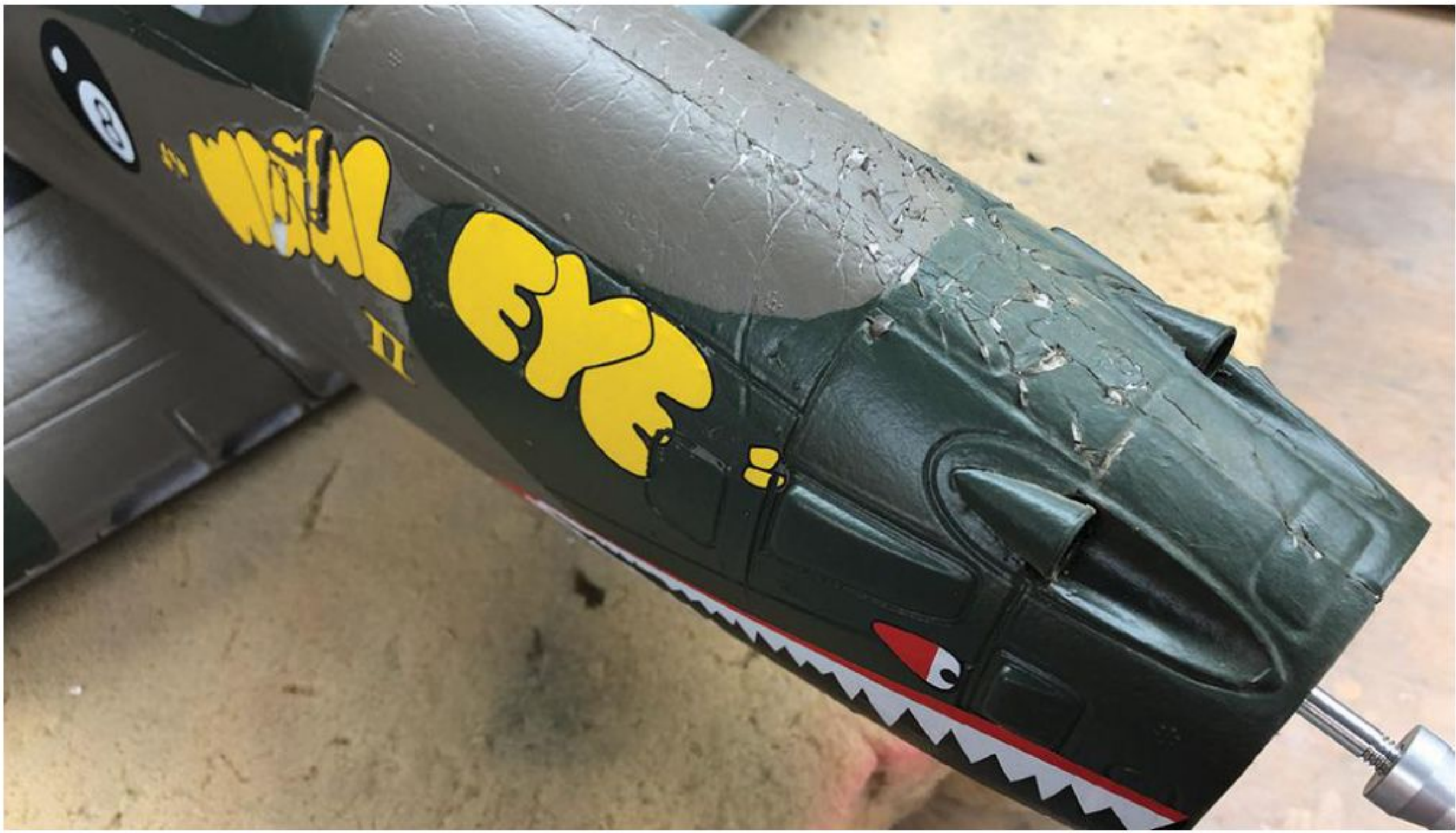
Here, you see some of the crinkles that have formed on the fuselage's nose resulting from the crash. Start the makeover by removing the propeller and spinner, then take the rest of the airframe apart.
