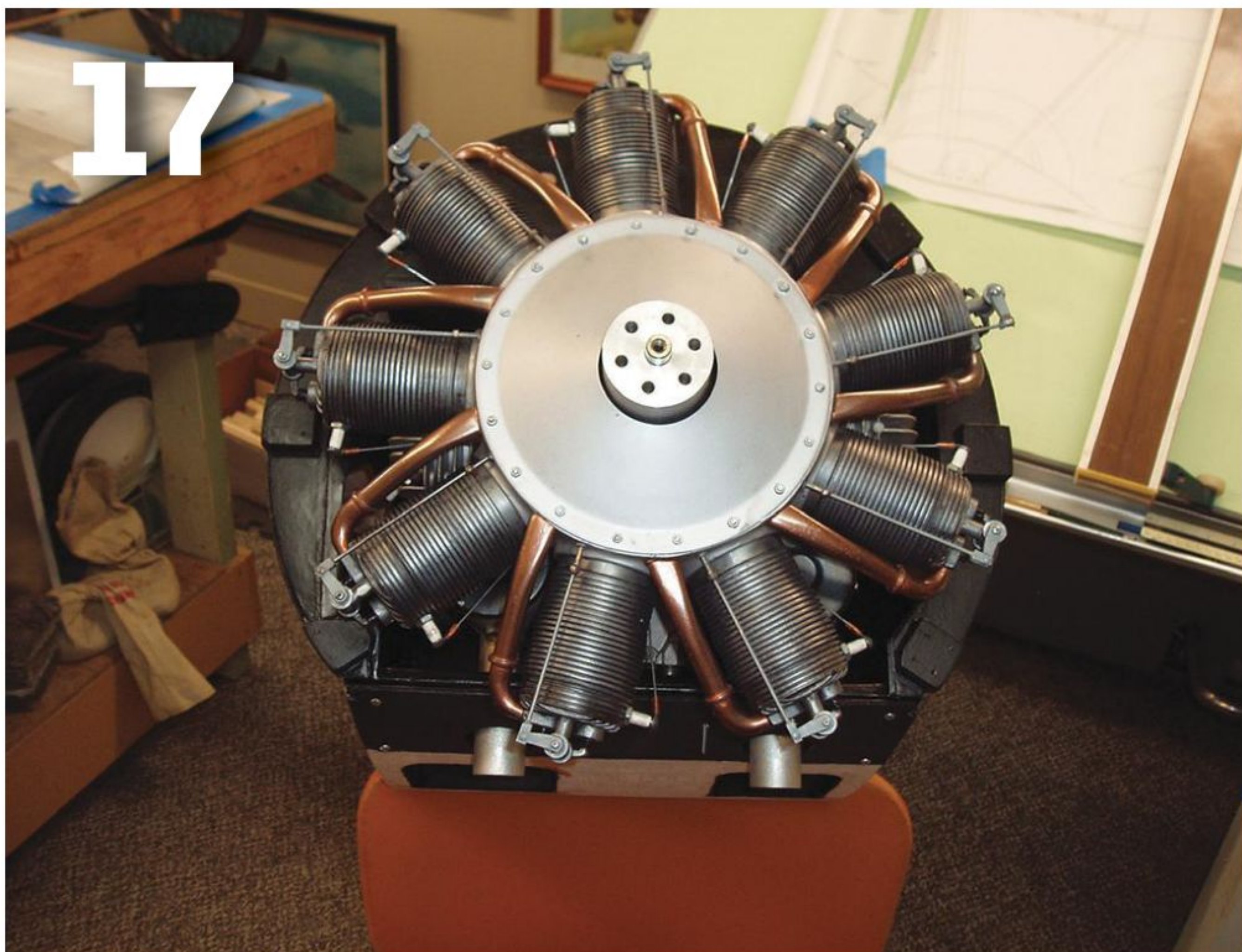
Dummy engine mount installed over DLE engine.
