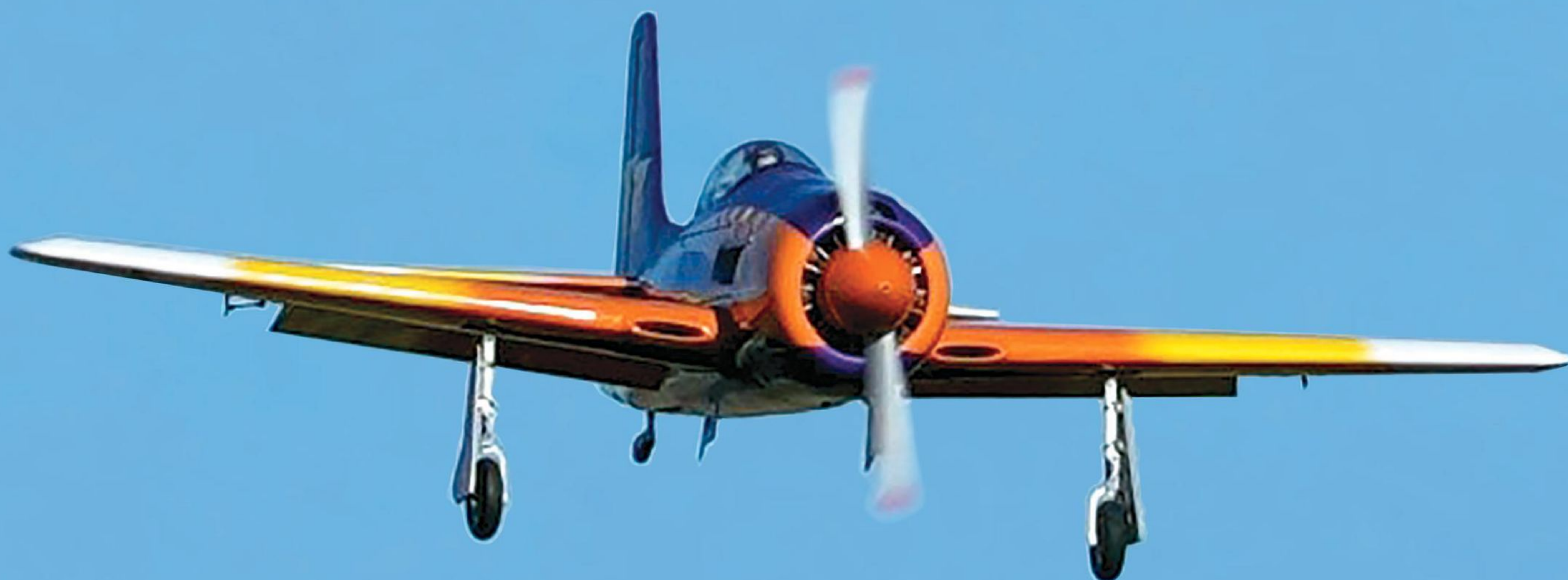
Coming in for a landing with flaps and landing gear extended. The Rare Bear has good slow-speed performance.
