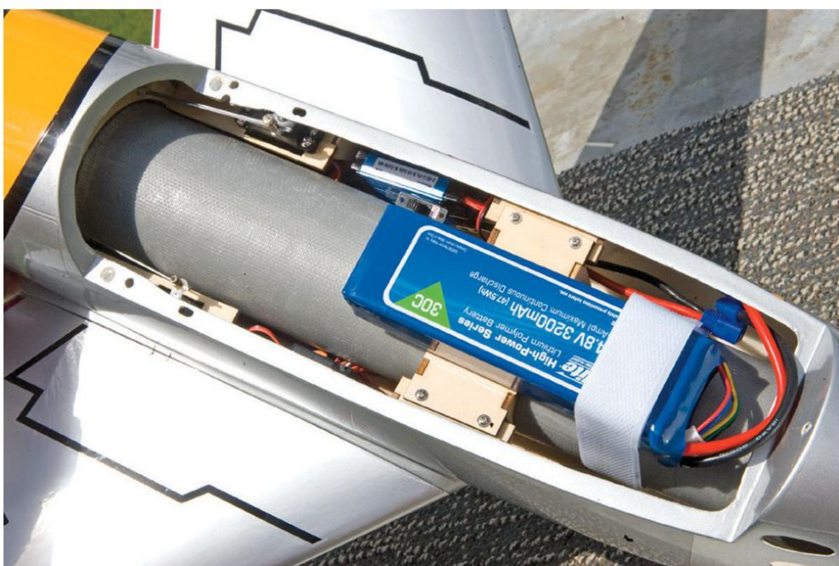
Battery packs are also very important. LiPo batteries are available in several cell counts and capacities. Be sure to match your pack to your jet's requirements.
