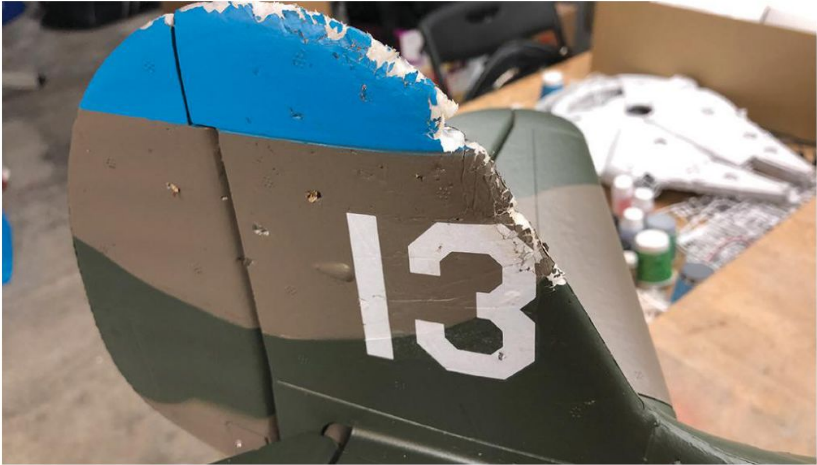
The aircraft hit the ground inverted, so the vertical tail took the brunt of the damage.
