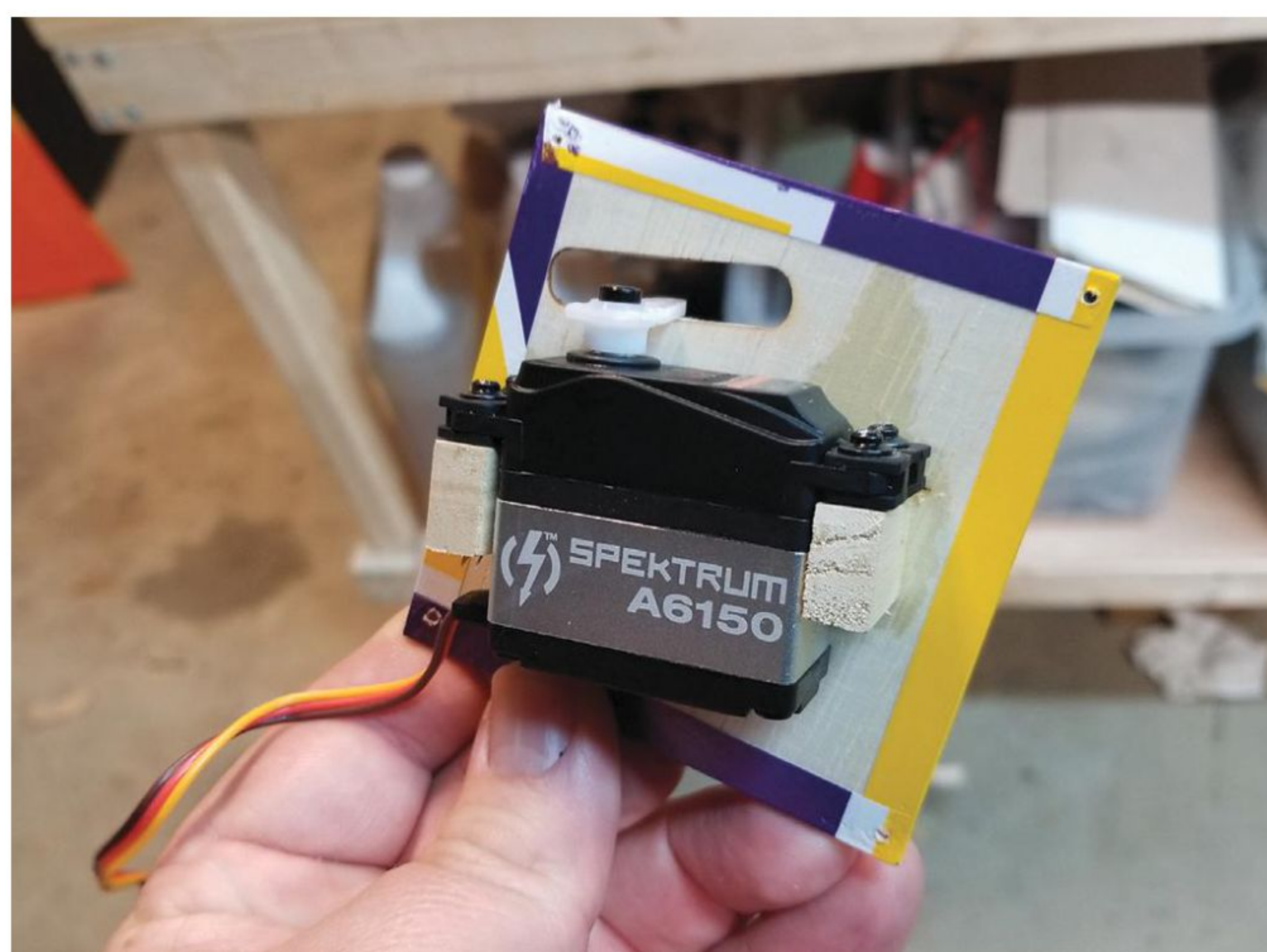
A6150 Spectrum HV servos were used throughout the model. They provide excellent control response.
