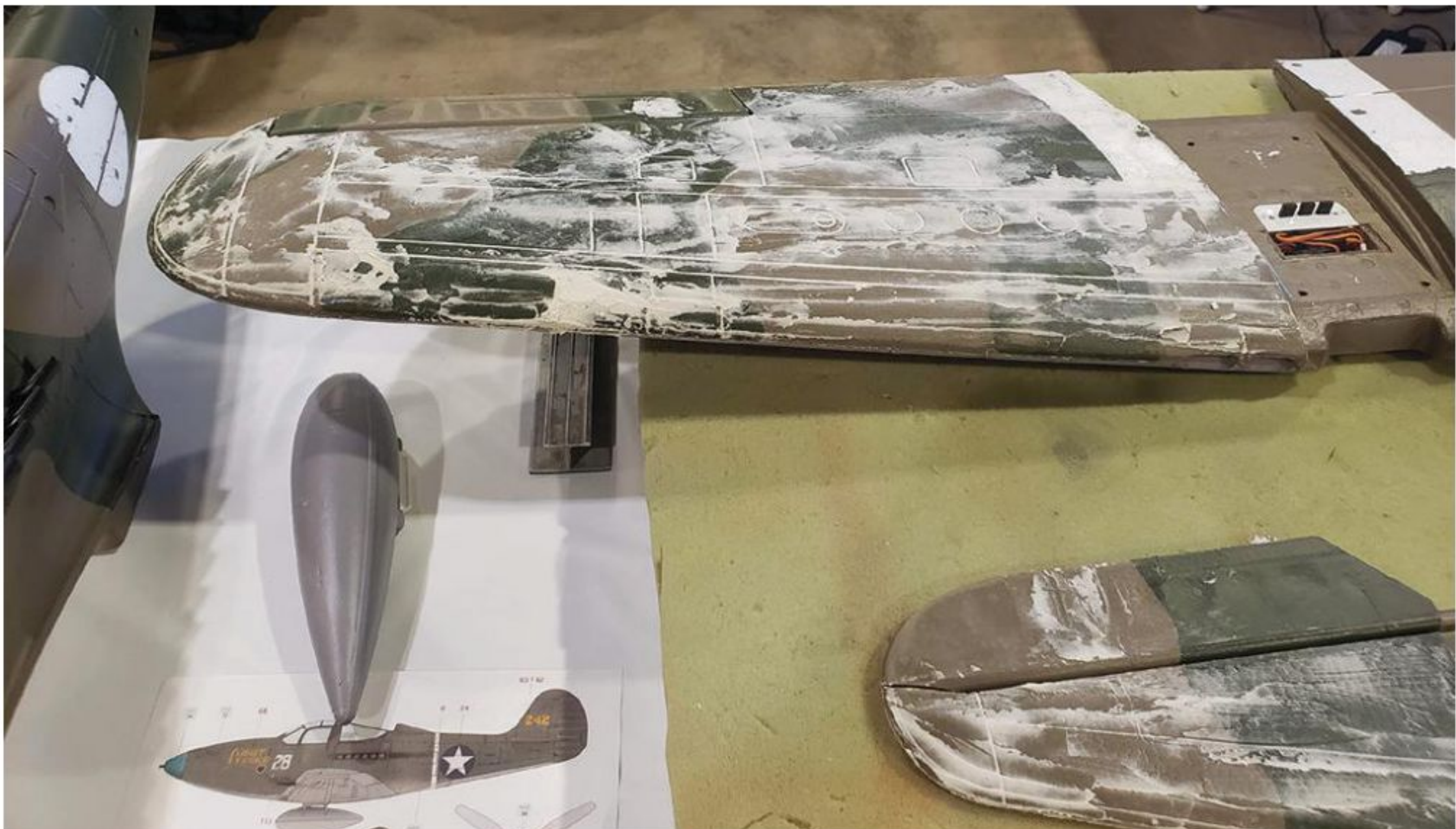
After a good cleaning and a light sanding with 180-grit sandpaper, apply some spackle filler to fill the damaged areas and molded-in panel lines.
