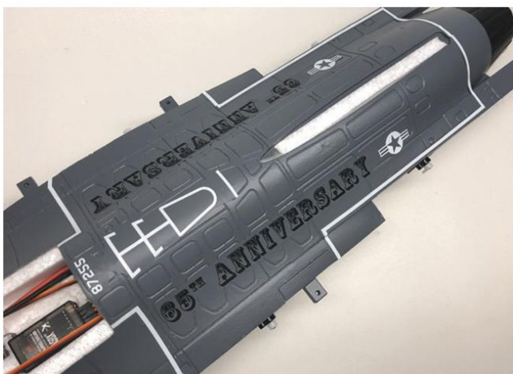
Upper aft fuselage prior to vertical fin installation. I used 15-minute epoxy on all foam-to-foam applications.
