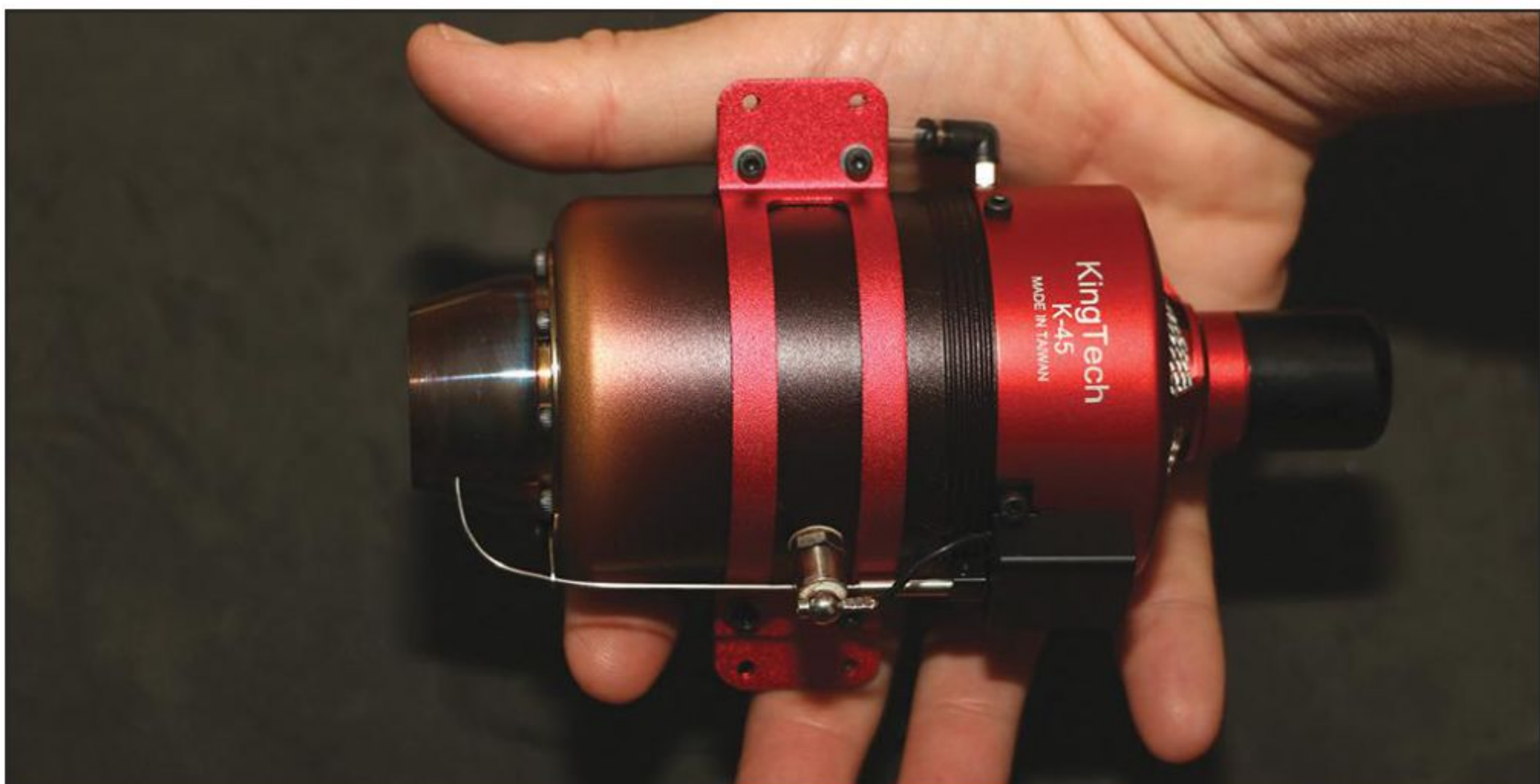
So small it fits easily in the palm of my hand! This view shows both the glow ignitor used during startup to ignite the atomized fuel/air mixture, and the exhaust gas temperature probe.
