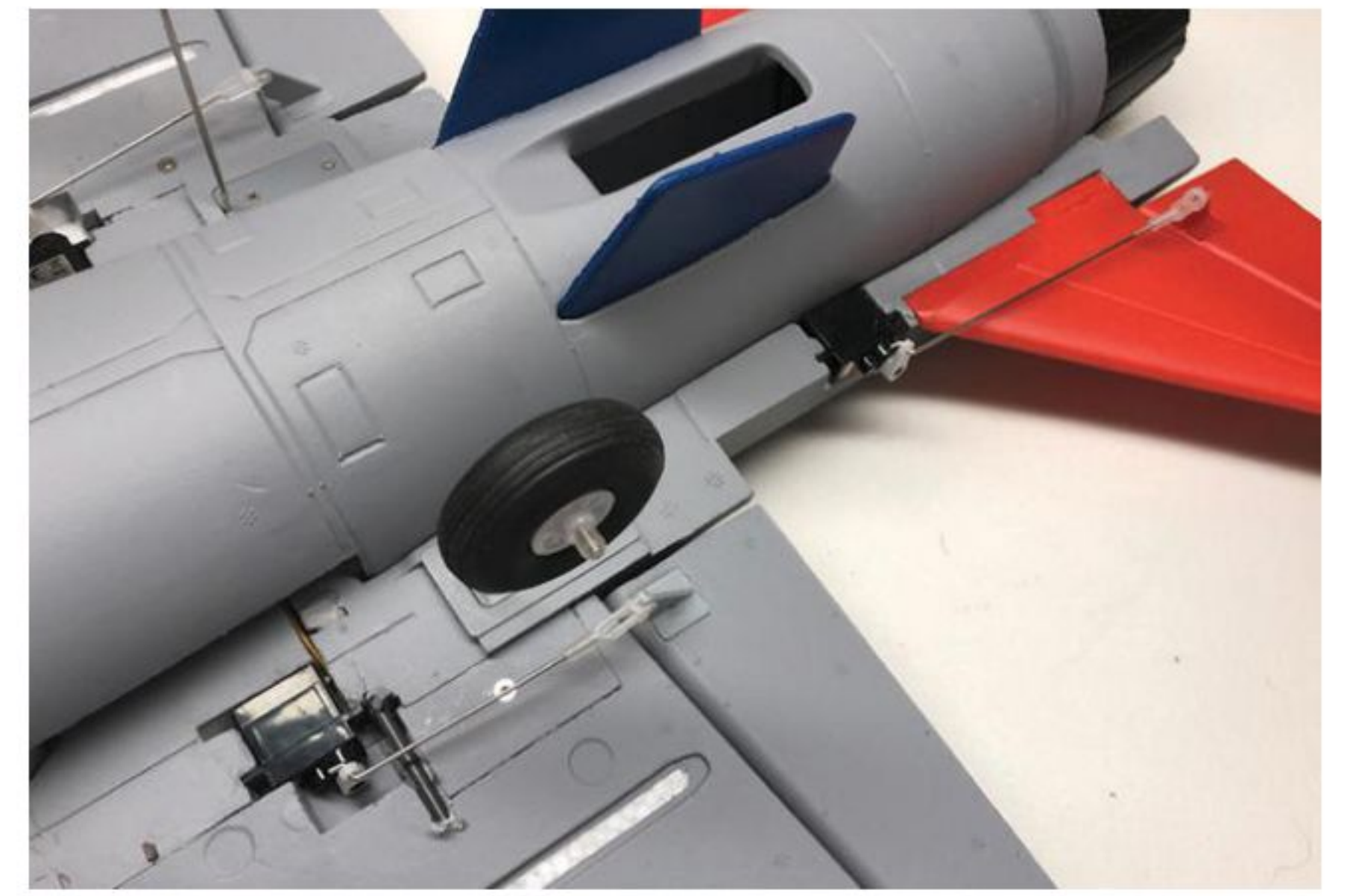
Bottom view showing aileron and elevator servos, ventral fins, and aux inlet for fan unit. Landing gear is easily removable.
