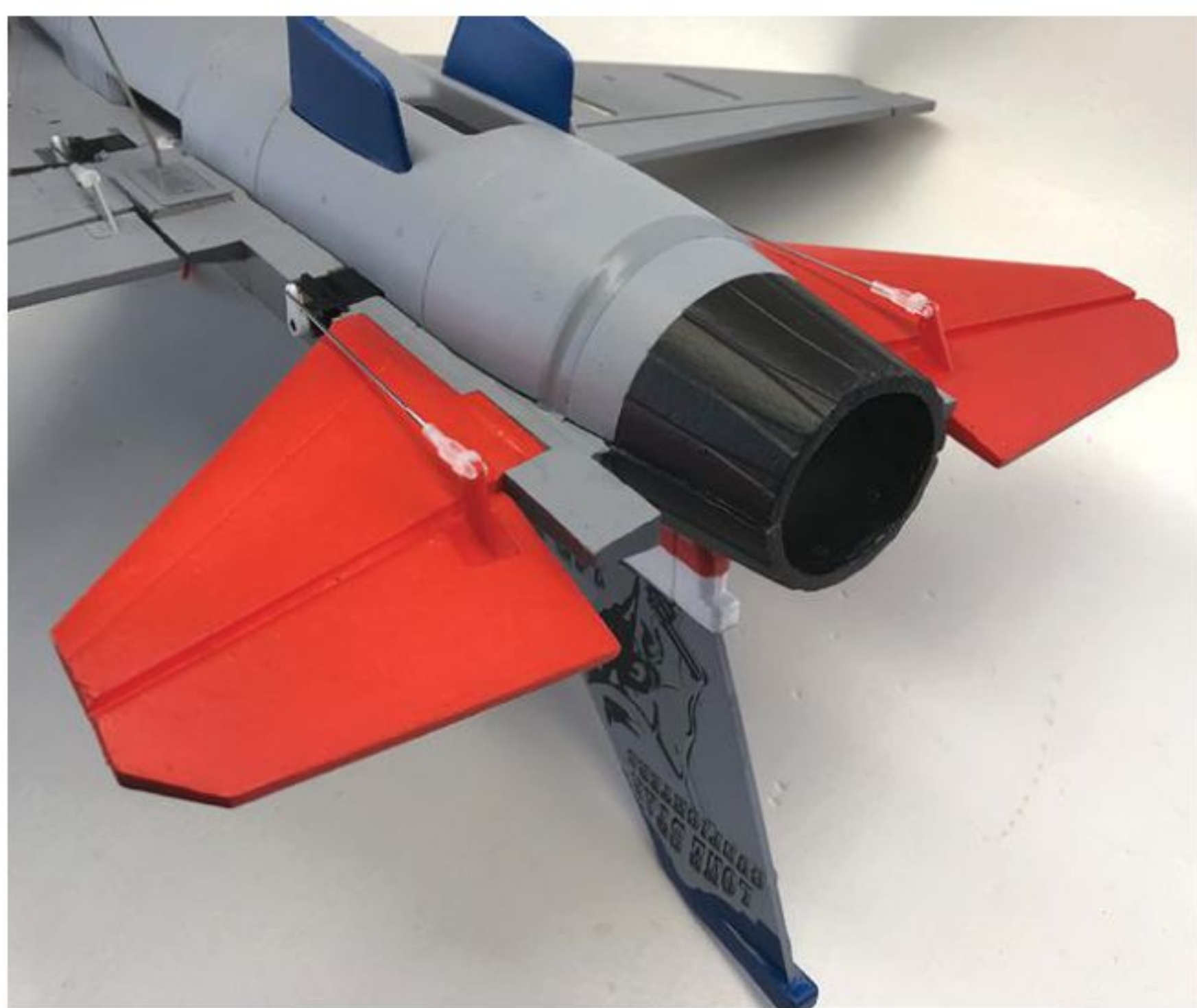
Aft section shows the stabilizer, elevator, and fin installations. Control linkages are short and straight, providing positive control.
