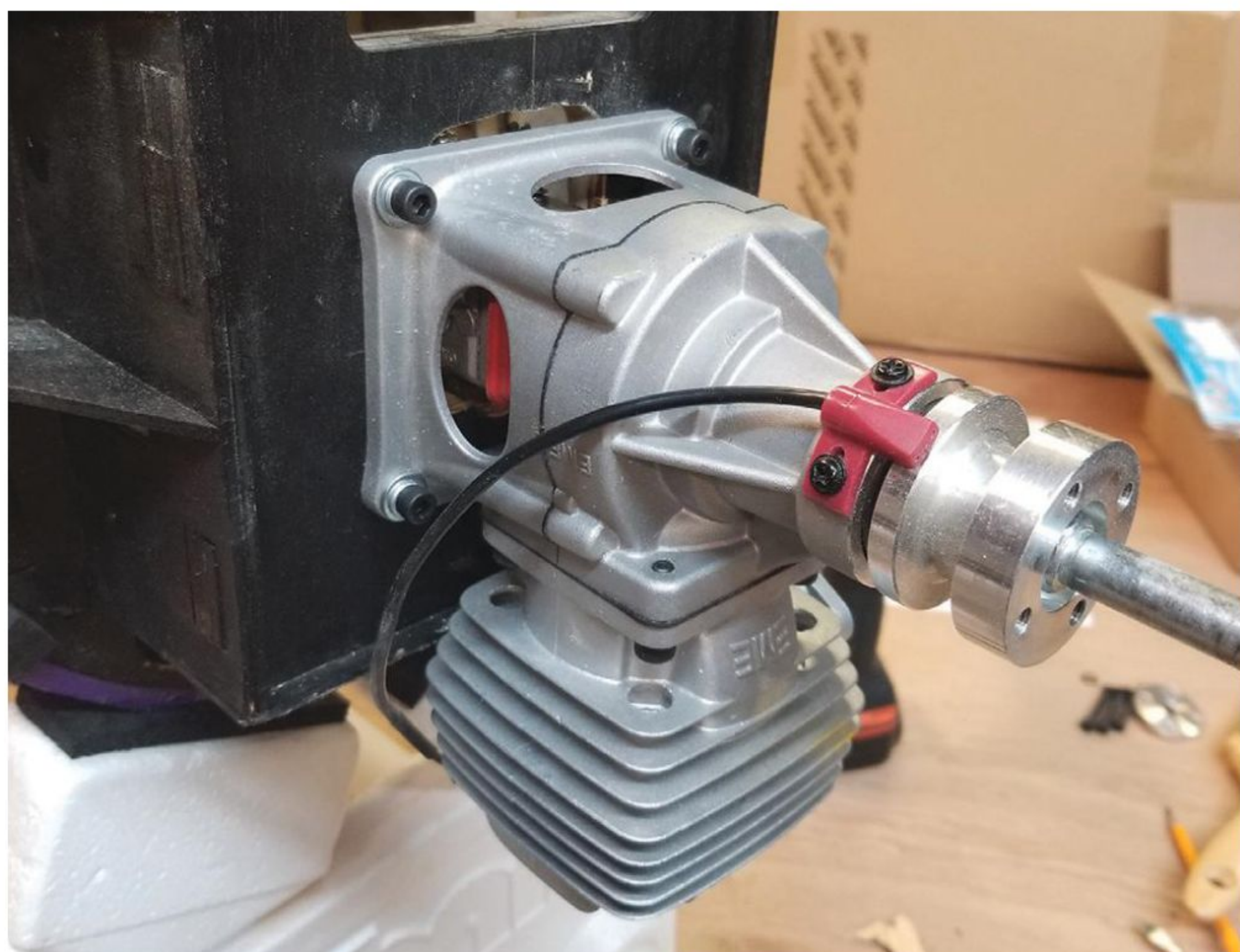
Here is the EME 60cc engine I used to power the Rare Bear.
