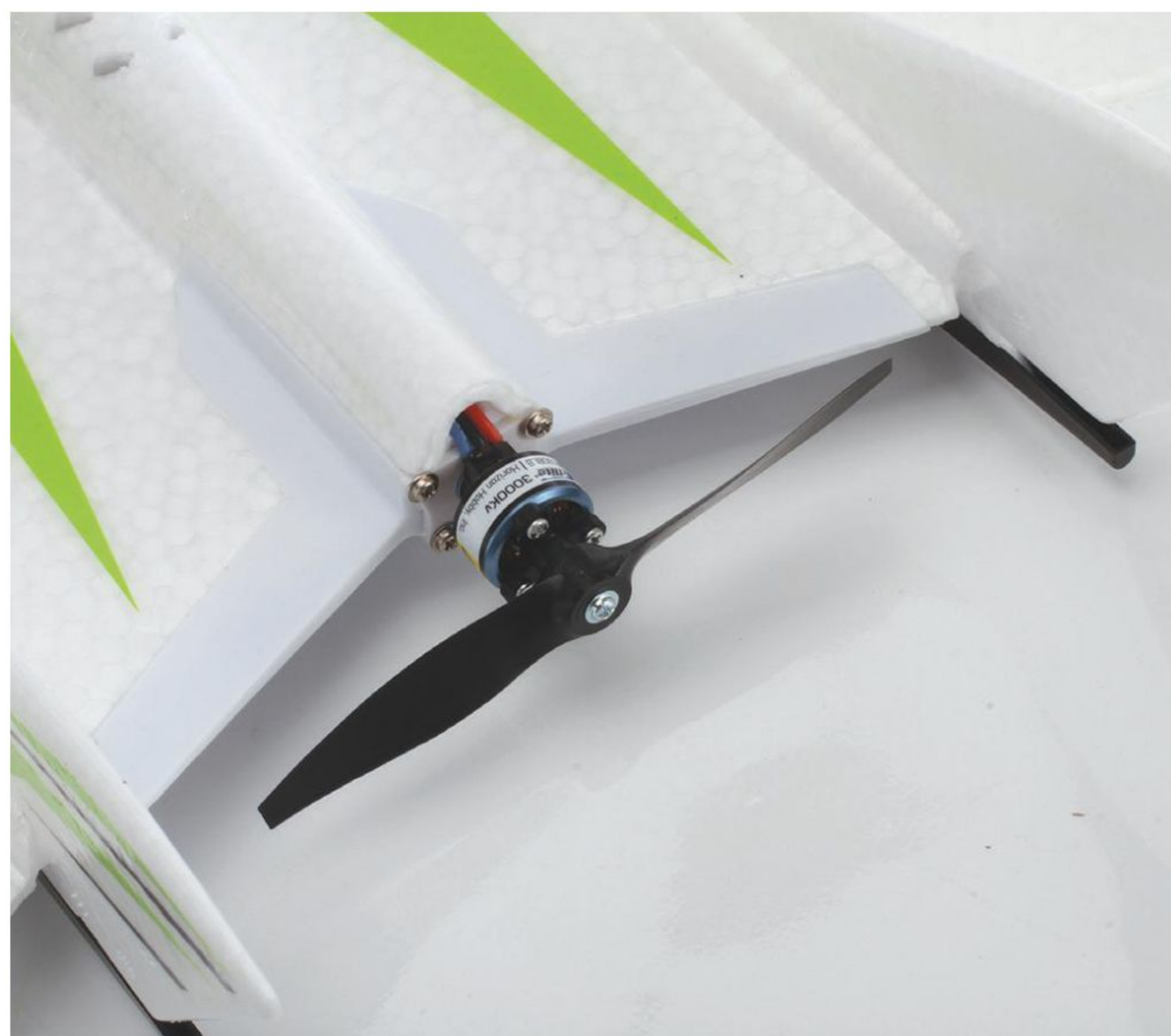
Here, you see the F-27 Evolution's pusher motor and propeller.
