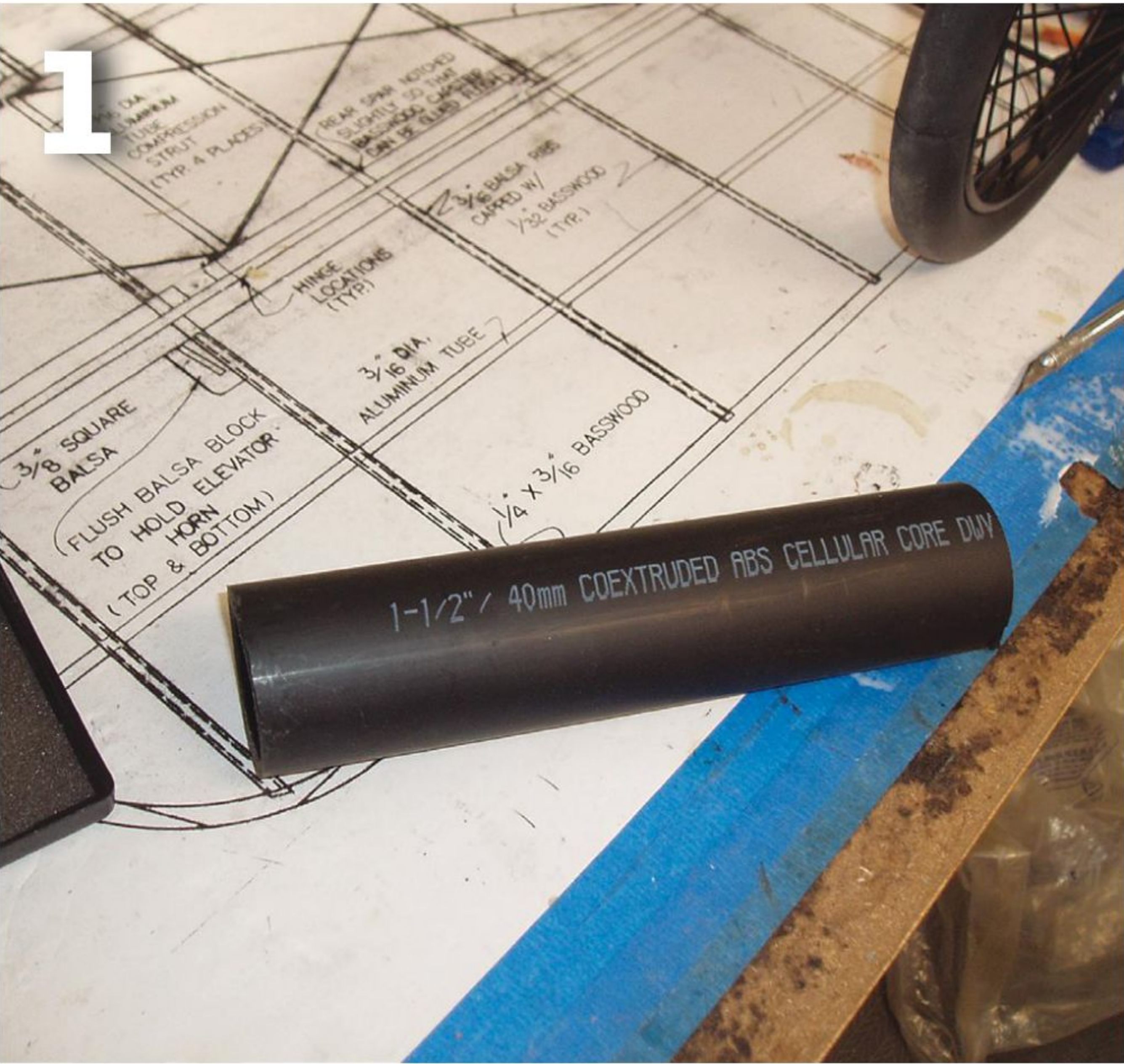
For my scale 9-cylinder Le Rhone rotary engine, I found that 1 1/2-inch ABS water pipe was the perfect size for turning the cylinders on my lathe.
