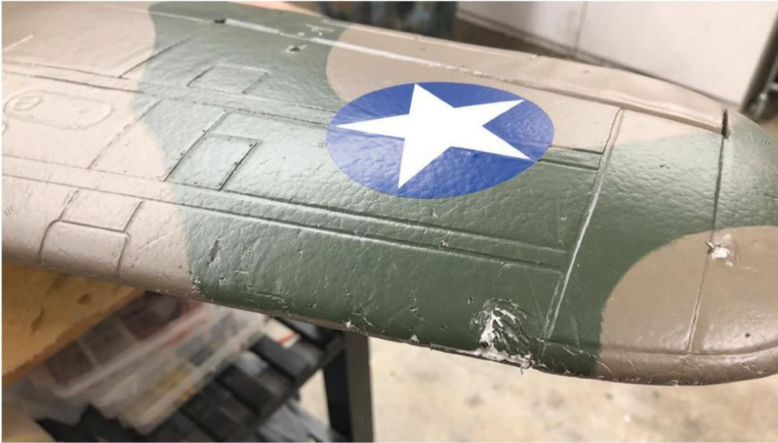
A dent in the wing's leading edge. This will be easily taken care of with some lightweight spackle filler.
