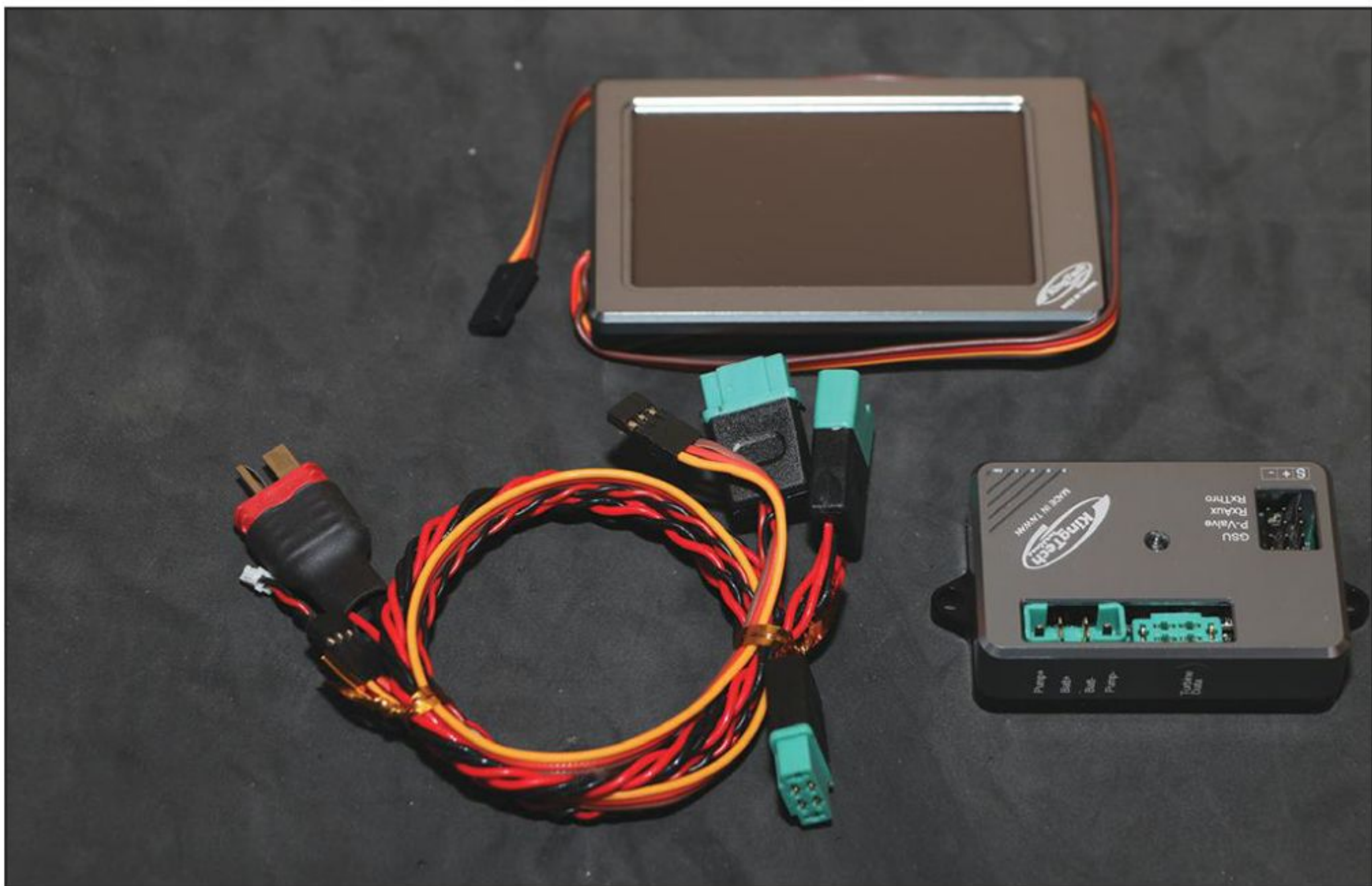
Touchscreen ground support unit (GSU), wiring harness, and electronic control unit (ECU).
