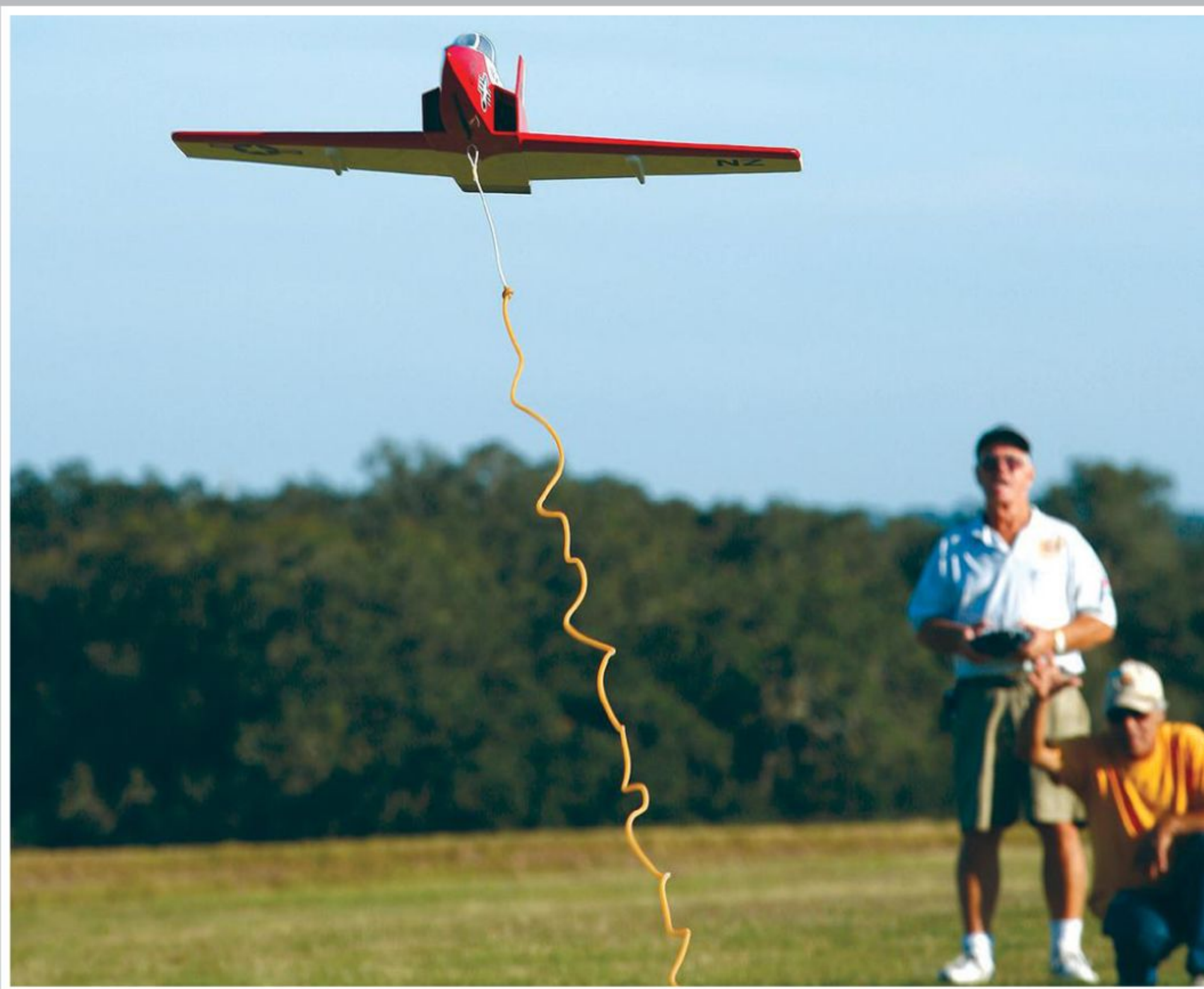
Expert model designer Nick Zirola Sr. built his Turbinator-E (a smaller e-powered version of his larger turbine jet) so that it can be easily bungee launched.
