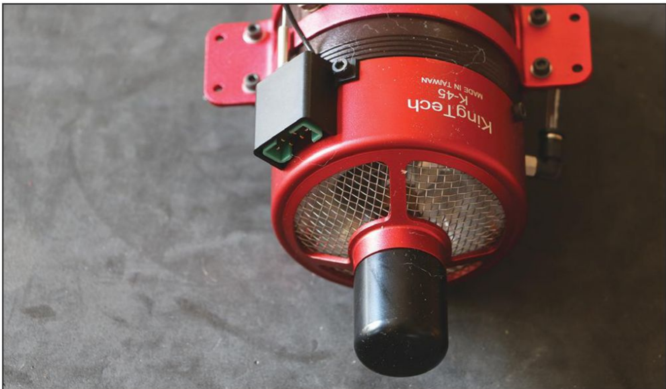
One of the new features on the G3 is the integrated FOD screen to prevent ingestion of debris that can destroy the turbine blades.
