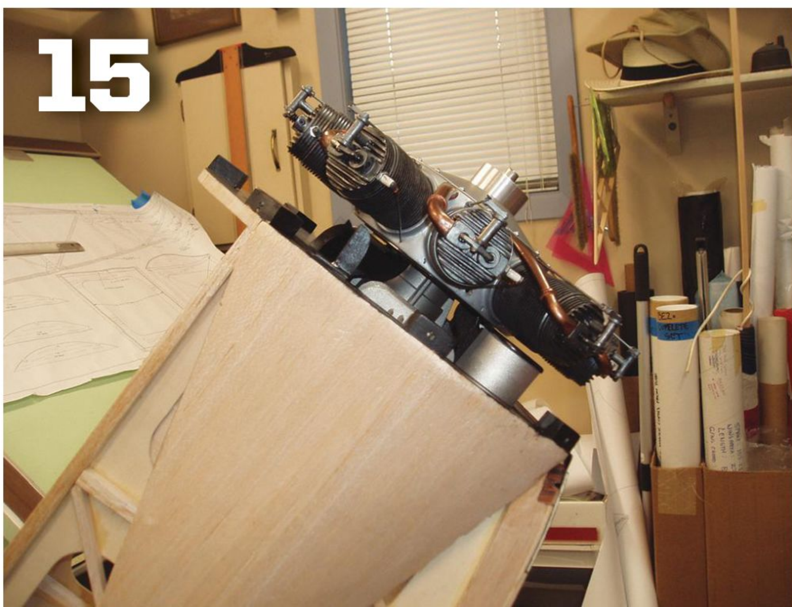
15 This side view shows the dummy engine installed. Clearance over mufflers is only 1/32 of an inch.
