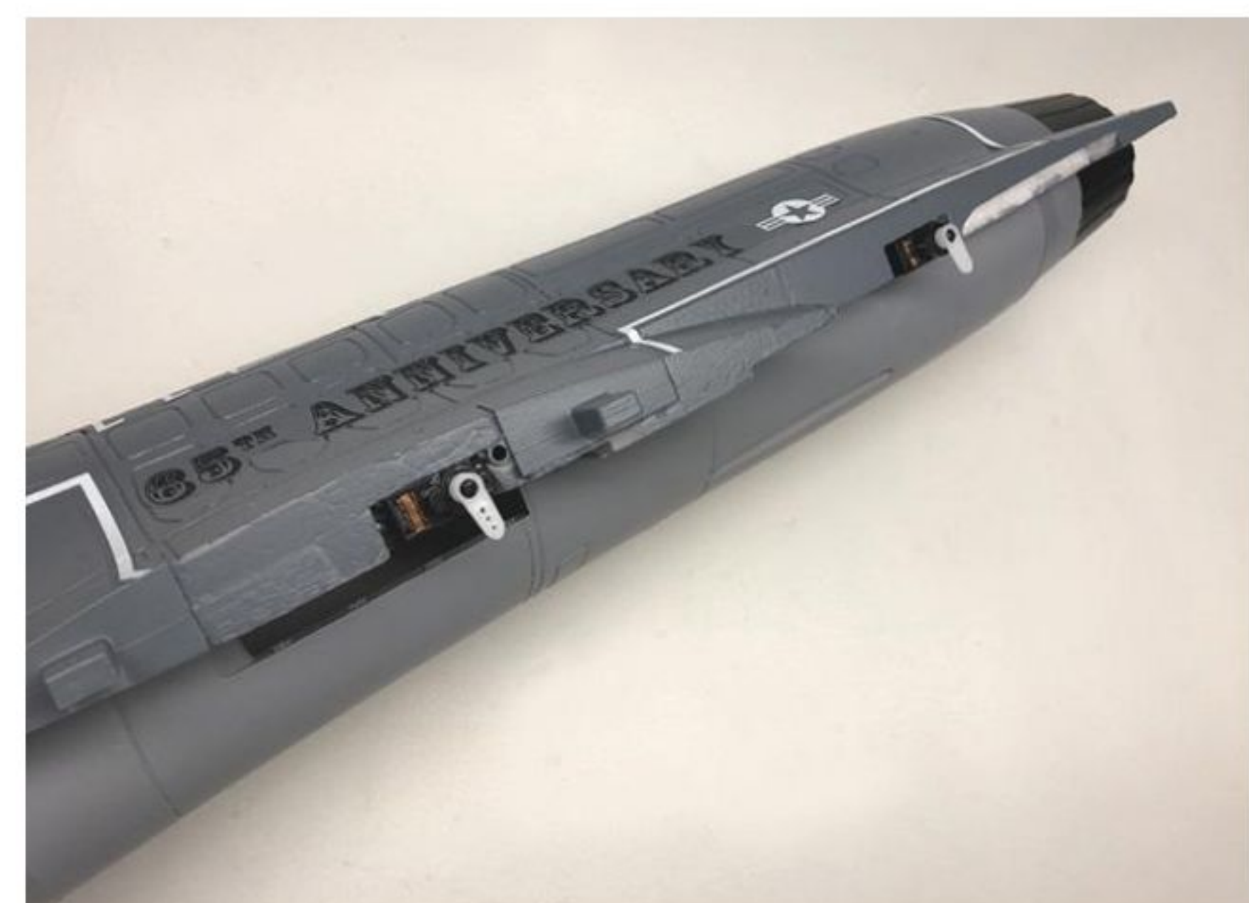
Left-hand side shows pre-installed mini servos for aileron and elevator surfaces.
