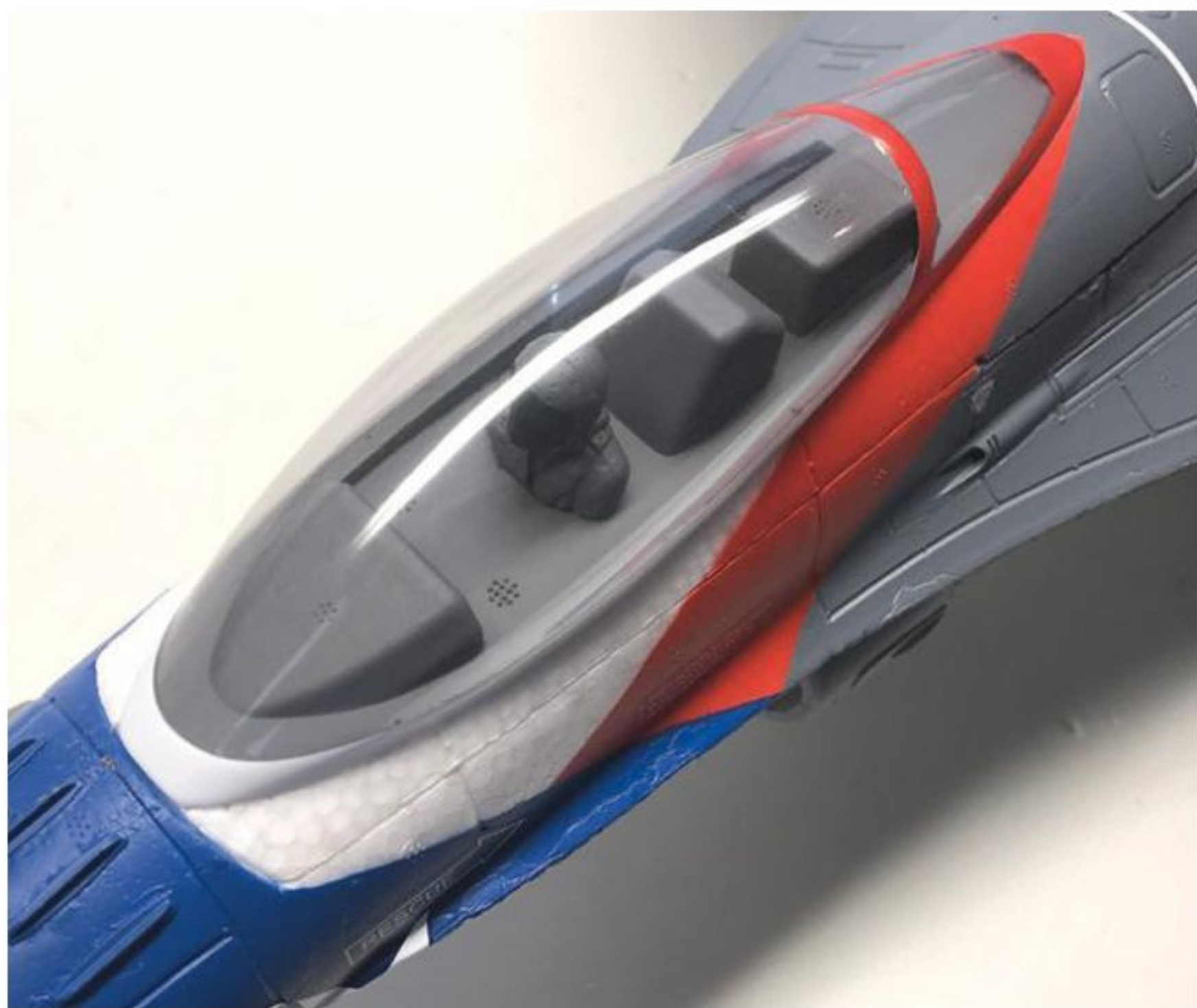
Canopy hatch fits snugly and is magnetically secured.
