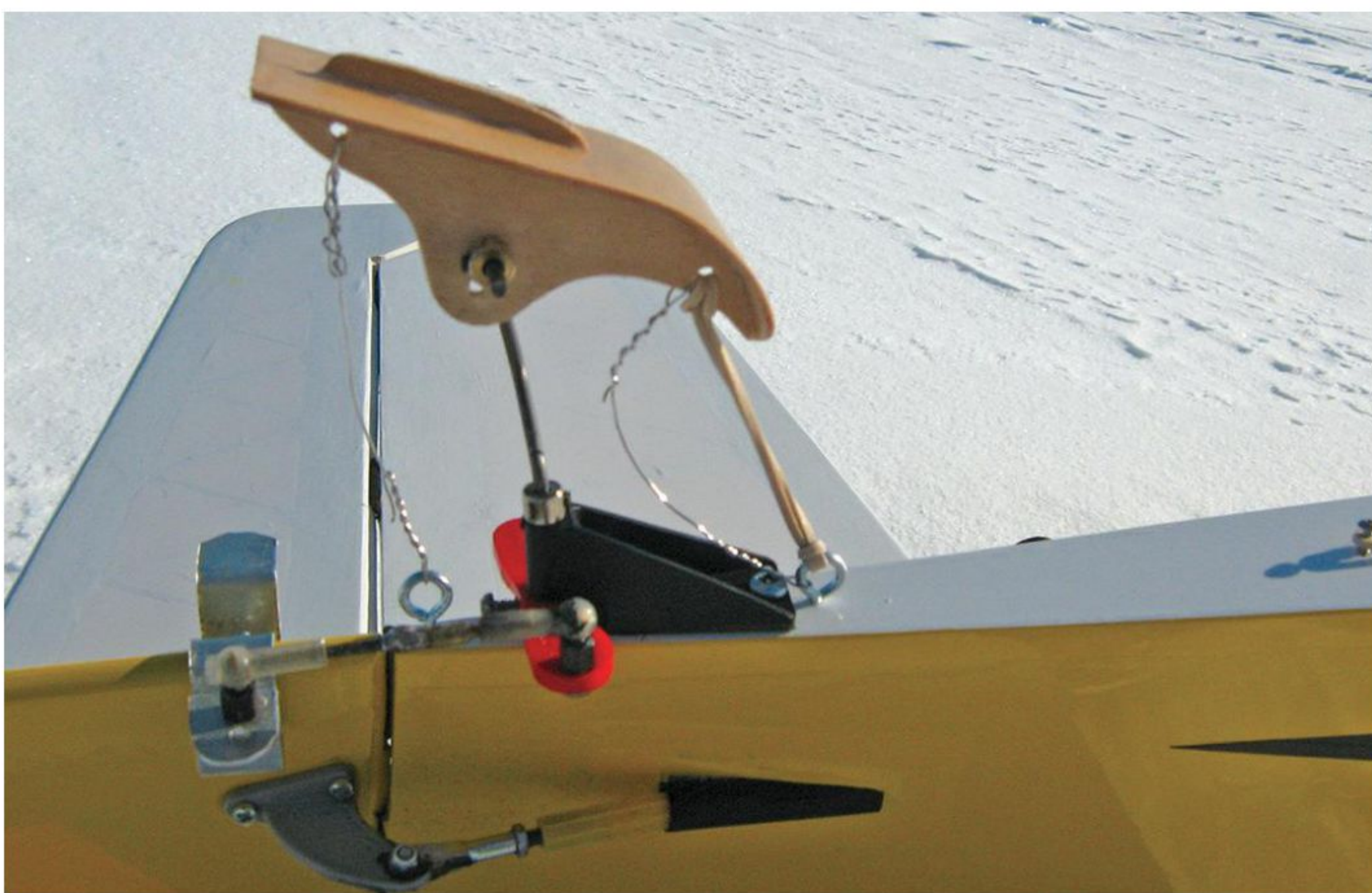
The tailwheel ski also uses limiter cables.
