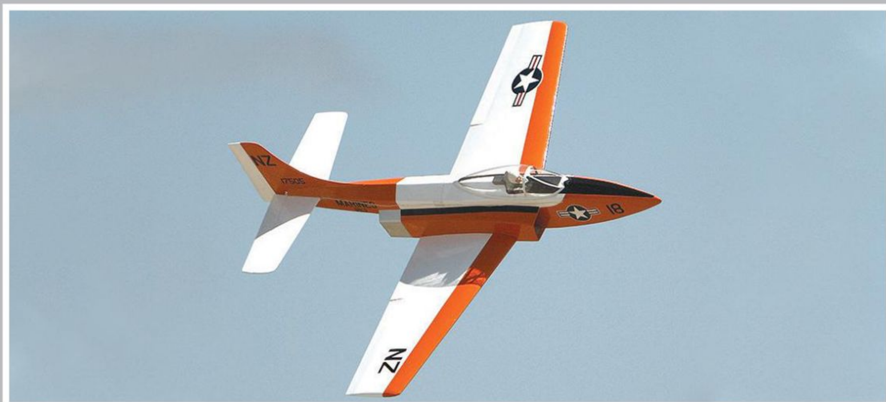
No landing gear means less weight and drag, which equates to more performance.
