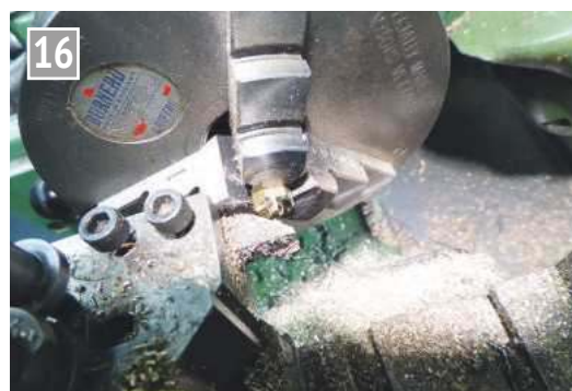
Beveling the rear and facing off the parting remains.
