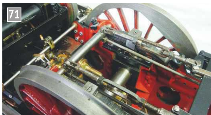
A4: Close up of brake rigging at leading coupled axle showing the adjusters.
