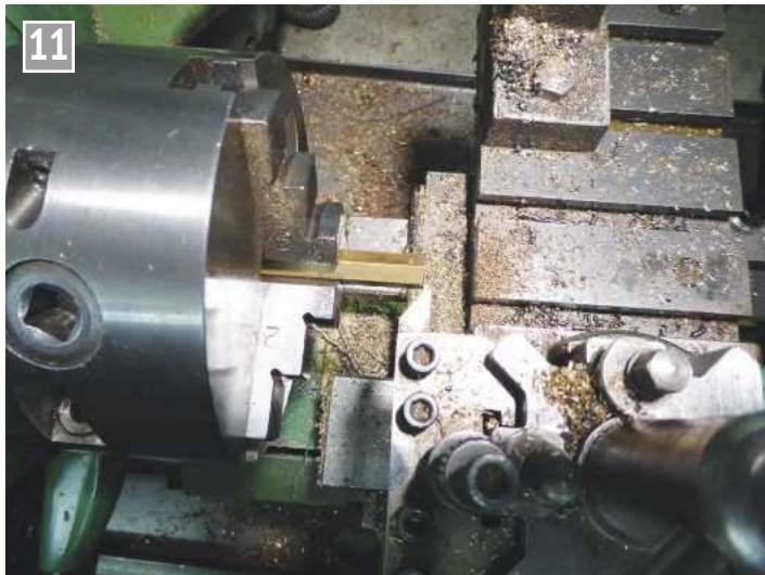
The beveling tool set up with its short horizontal face about level with the hexagonal face of the material ...
