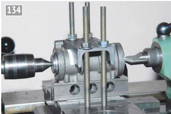
Setting the cylinder up for boring.
