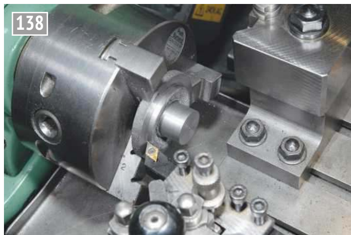
Machining the chucking piece on the cylinder cover.
