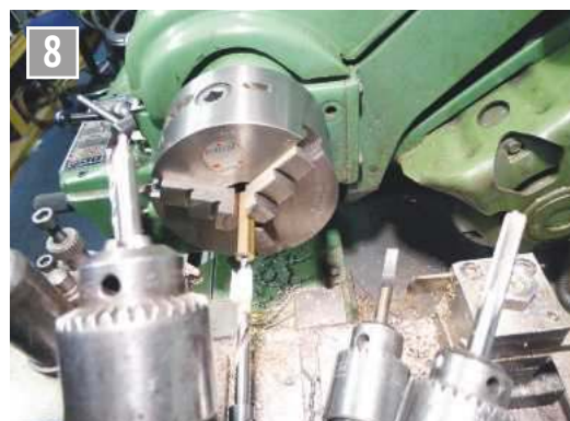
The tapping drill, complete with paper depth stop.
