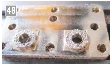
Finishing the pump plates.
