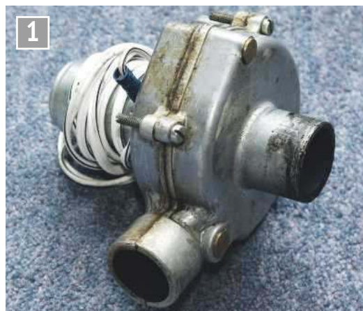
Typical (commercial) steam-raising blower.
