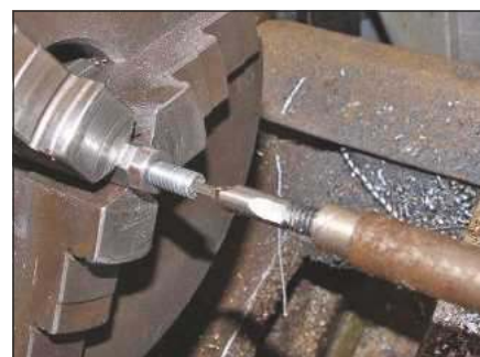
Malcolm Leafe describes a simple approach to Rotary Broaching.
