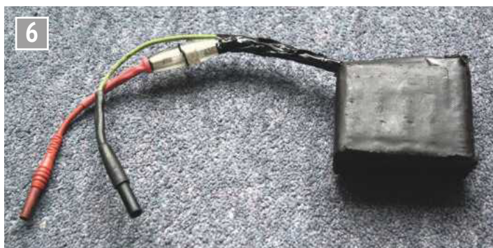
6 Assembled battery pack, complete with in-line fuse-holder. This particular example has seen 5+ years of service (without needing to change the cells).
