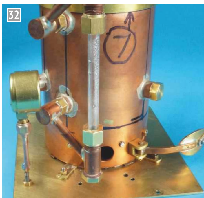
This plate supports the boiler.
