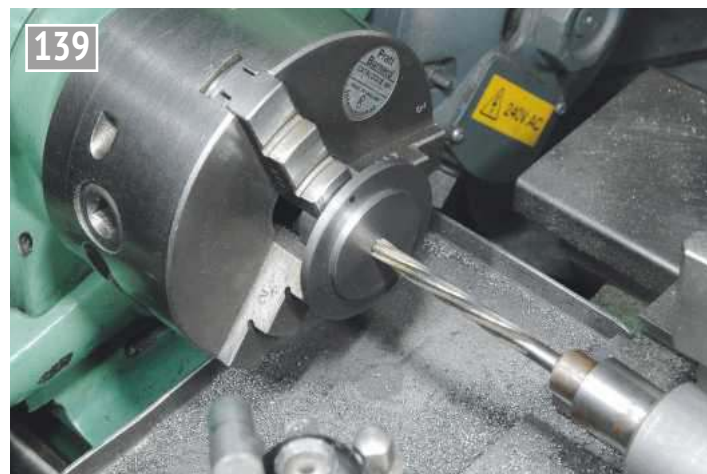
The cylinder cover register and bore are made at the same setting.
