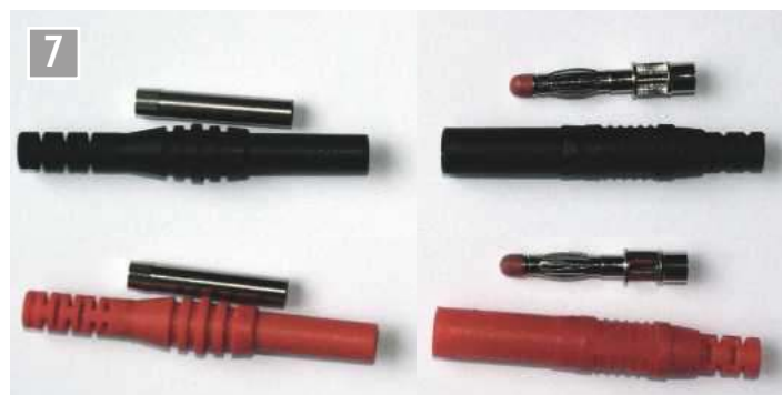
7 In-line sockets and plugs – note that the sockets (on the left) are the CPC version and the plugs (on the right) are from eBay; the former are of a higher quality!
