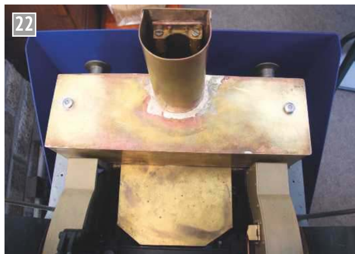
A view of the tanks assembled back onto the chassis with the tie bolts in place. Note the space around the bunker tank to be taken up by the rear steel cab structure.
