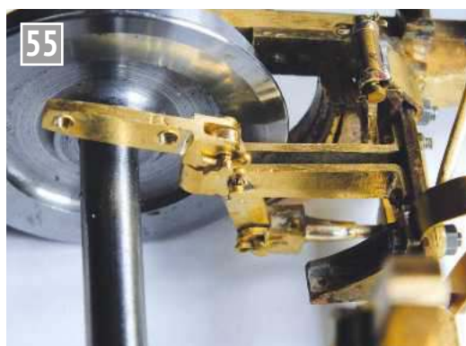
Fabricating a brake shoe holder.
