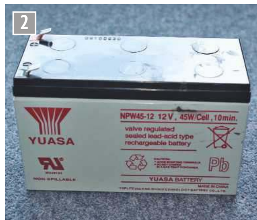
Typical lead acid 'gel' battery often used in powering steam-raising blowers.
