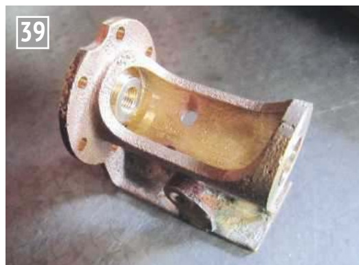
The coupler with the steam gland fitted.
