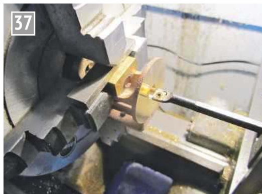
Facing and boring the coupler casting.
