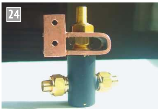
Here are the first two stages in producing the injector water valve bracket with the mounting pad silver soldered in place.
