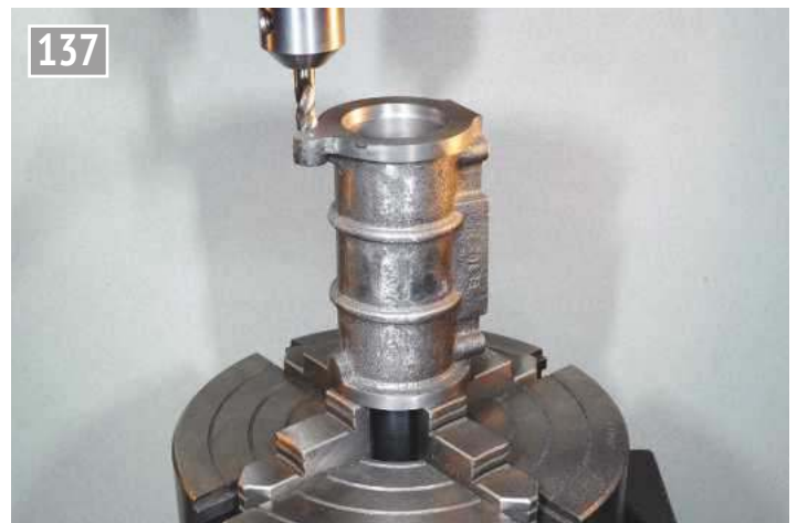
Shaping the outside of the flange.
