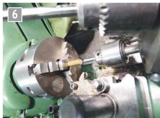
Centre drilling the faced hexagonal brass bar.
