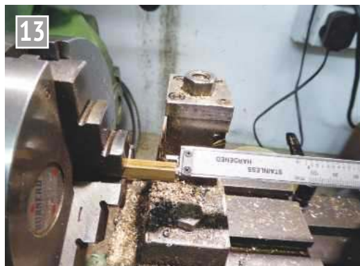
The depth gauge calliper, used to set the parting off depth. The one shown was a free gift to Model Engineer subscribers quite a while ago.
