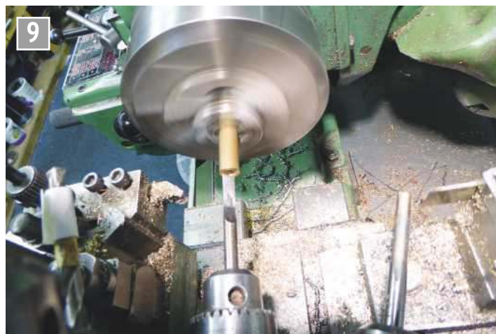
The 'D' bit gives a flat seat at the operating face of the nut.
