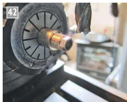
Forming a hexagonal end for the gland nut.
