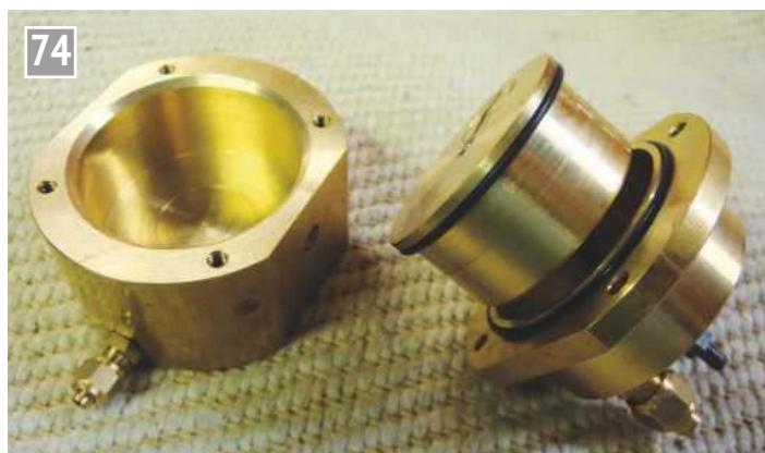
A4: Vacuum cylinder parts showing the rolling ring.
