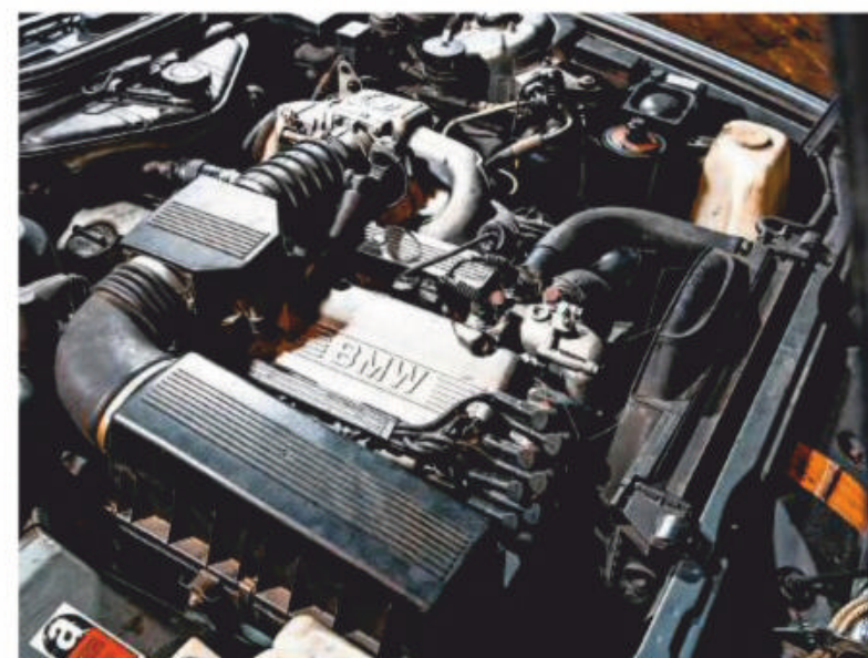
▲ M30/6 produces 197bhp in 730i form.
