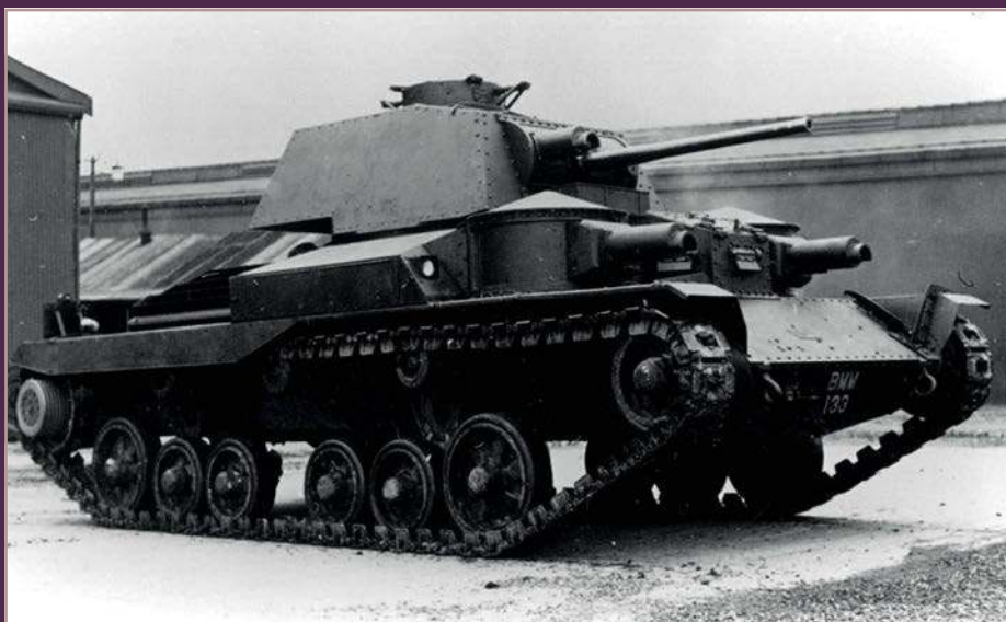
A9E1 1326-C6 A9E1 prototype showing many differences from the production vehicle. Hull front shape changed while the conical tops to the machine gun turrets and the commander's cupola were dropped.
