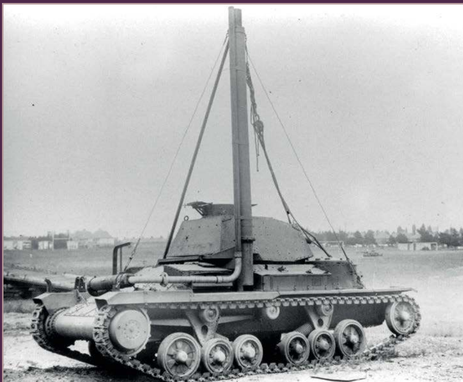
A9E1 wading 6668-B3 The prototype was later used for trials for wading. Various tubes were added to bring in air and remove exhaust gasses. As the tank was missing several rivets it filled with water and sank.
