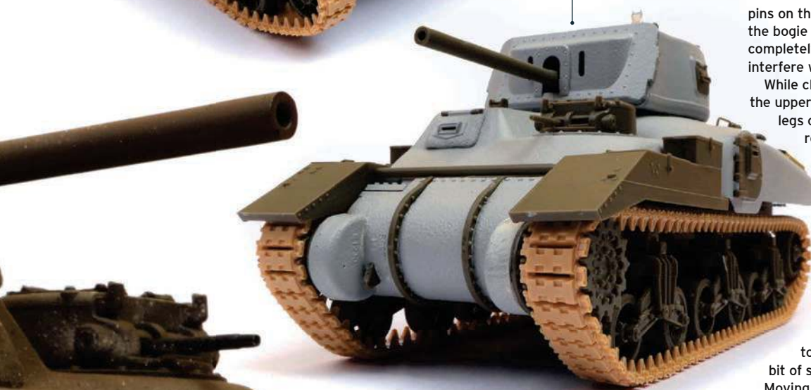
The hull and turret were retextured using a thick mix of Tamiya Extra Thin Liquid Cement and Tamiya White Putty.
