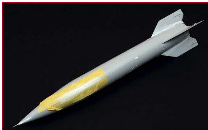
The gaps were filled with Milliput White two-part epoxy putty.
