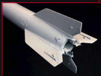
The large connectors resulted in a noticeable gap on one side.
