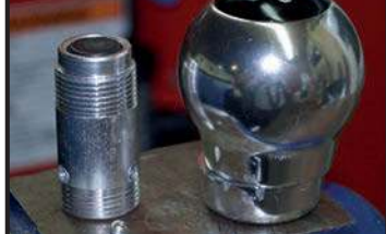
Photo 1. The Components. The Knob is sitting on the Threaded Collet, also only one of the three grub screws could be removed (this required some fettling)
