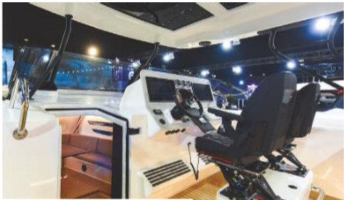
The standard suspension seats take the edge off when travelling fast in rough seas
