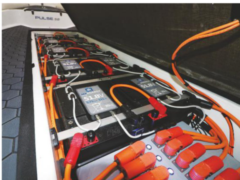
LEFT The battery pack is from a Nissan Leaf BELOW Fully integrated helm gives detailed info on remaining charge and real-time range
