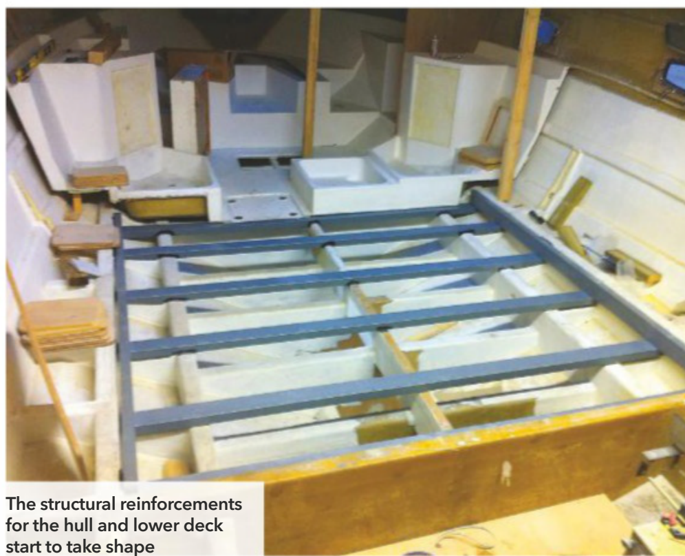
Jimmy built a latticework of frames to support every panel and retain a layer of insulation
