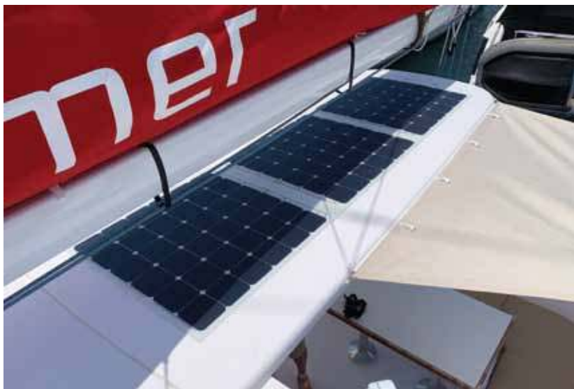
LEFT: Walk on solar panels.
