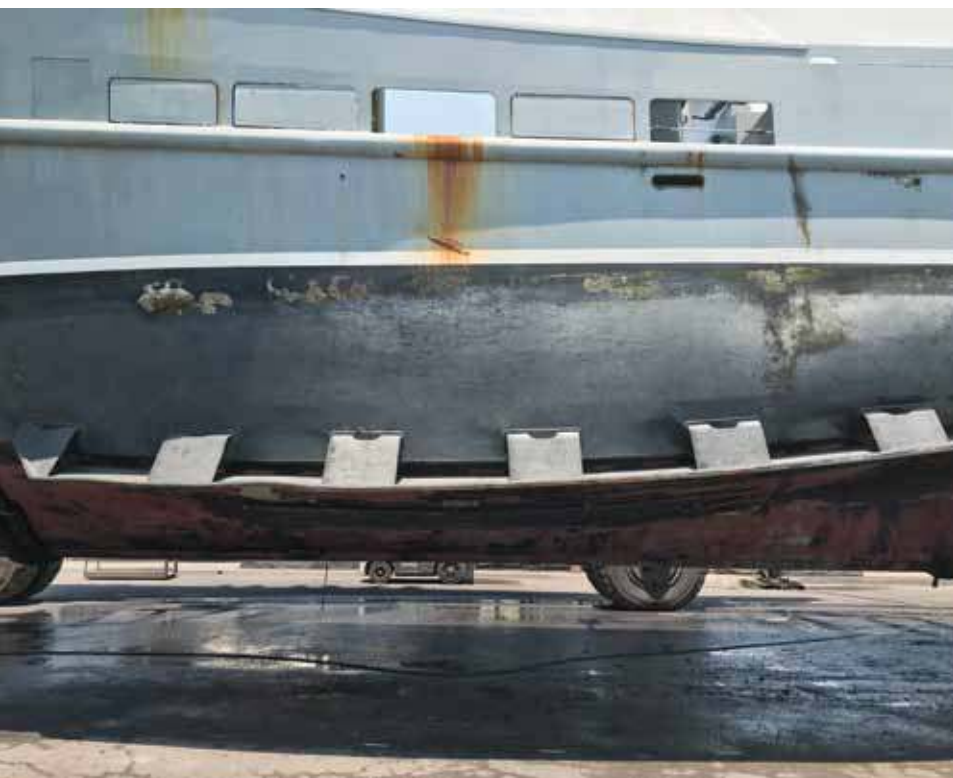
Basic bilge keels fitted to a fishing boat to reduce rolling.
