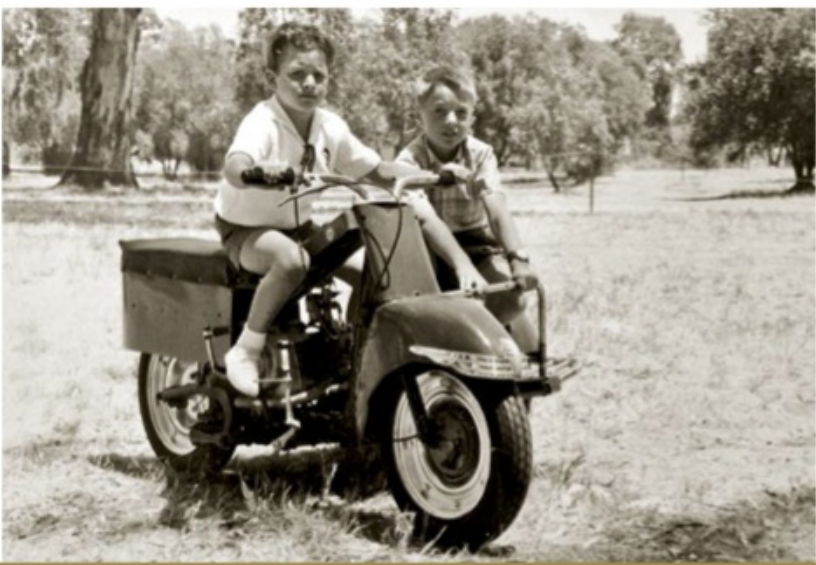
LEFT Murray's son Darren on the machine built for him by his father, using a Zundapp Bella scooter with a 90cc Honda engine.
