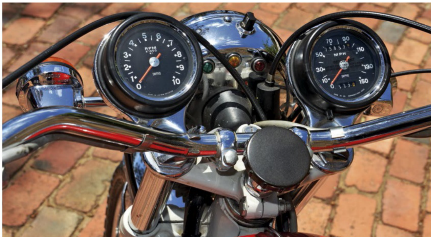
ABOVE Top clocks. Smiths instruments, substantially rubber mounted. BELOW LEFT The ubiquitous Triumph conical rear hub, used across the range including on the BSA off roaders. BELOW CENTRE Side covers are much less ornate, and smaller, than the original model.
