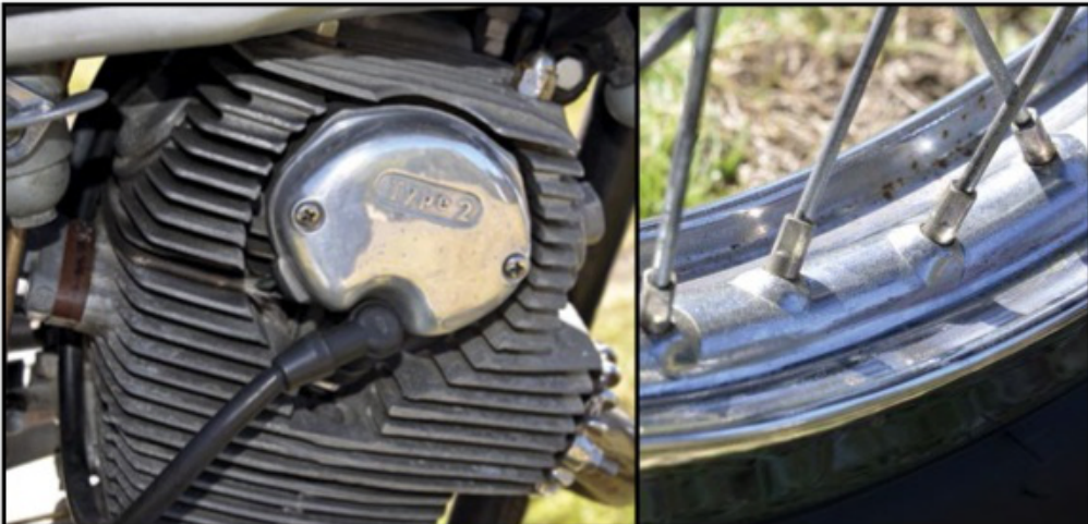
ABOVE LEFT Type 2 engine with 360 degree crank. ABOVE RIGHT The DID shouldered wheel rims which were original equipment on the CL72. BELOW LEFT Turn indicators began appearing late in the CL72 production run. BELOW RIGHT Hydraulic steering damper was a modern touch in the early 'sixties.
