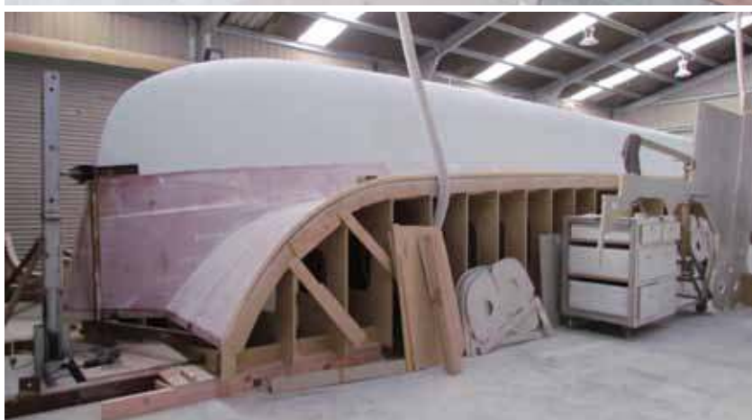
FROM TOP: Bulkheads Installed.
