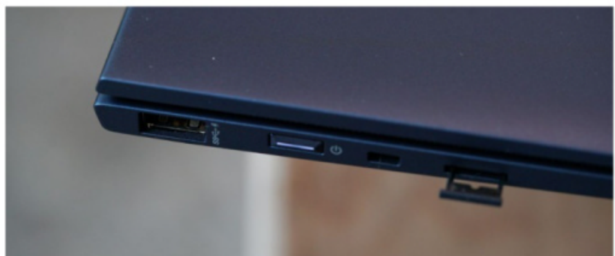
The Elite Dragonfly's left side features a USB Type A port, a power button, a lock port, and a SIM slot.
