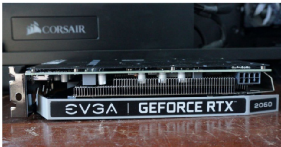
The EVGA GeForce RTX 2060 KO uses a single 8-pin power connection.
