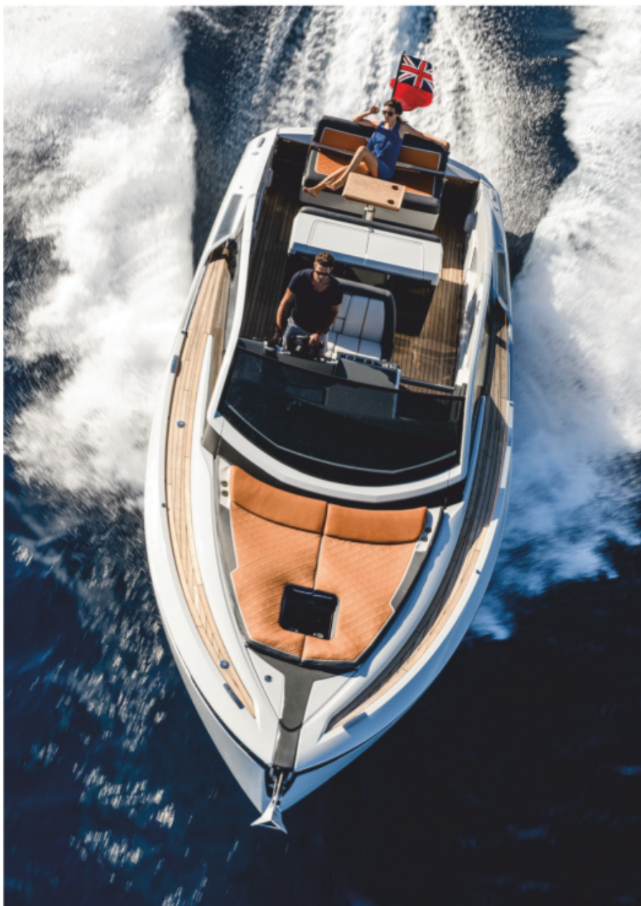
The Fairline cuts a sharp offshore shape with 22 degrees of dead-rise at the transom and a pad in the keel aft to add stability.
