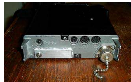
The additional heatsink in position.
