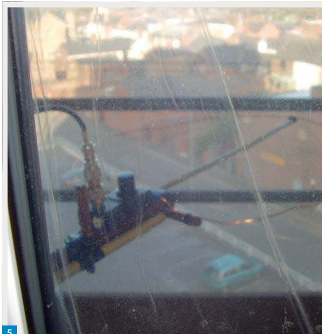
Fig. 3: The loop mounted on bamboo cane.
