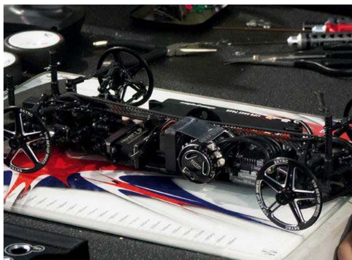
Note the Lexan piece that controls the airflow from the fan and over the motor
