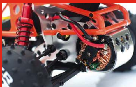
Here you can see the shaped moulding that allows access to the slipper clutch nut
