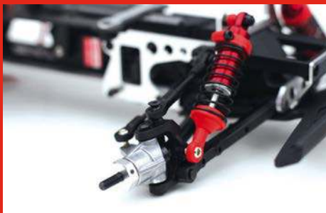
The front shock absorbers actually pivot off the caster block
