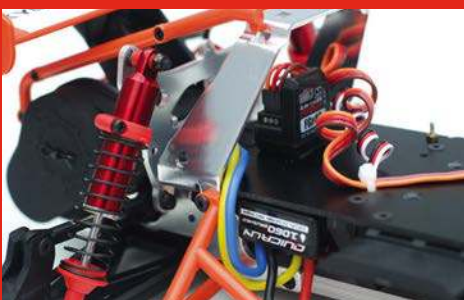
The speed control is positioned upside down on the upper chassis plate
