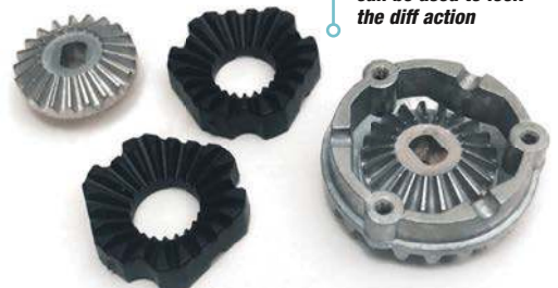
The moulded pieces can be used to lock the diff action
