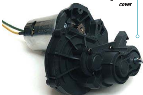
The pinion/spur gear mesh can be checked by removing a small cover
