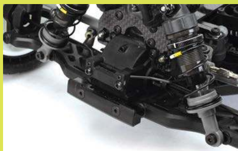
For high-grip tracks like carpet and dry Astroturf the front anti-roll bar will aid handling
