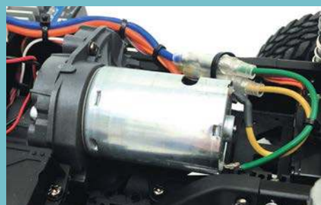
A Mabuchi 540-size 27-turn brushed motor is supplied in the kit
