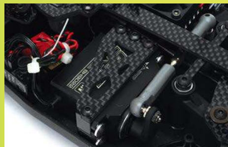
The SRT BH9022 HV Brushless servo is fitted to a floating mount to prevent chassis tweak
