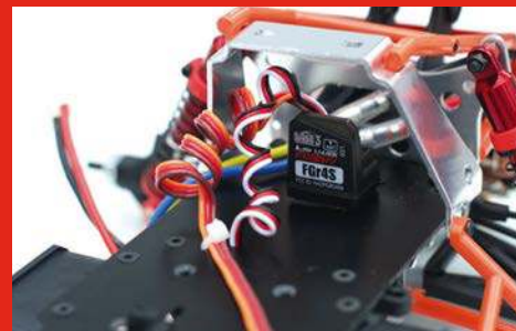
A tiny FlySky 2.4GHz receiver was used and sits on the upper deck
