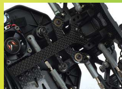
The front half of the chassis features plenty of carbon fibre like the steering brace and drag link
