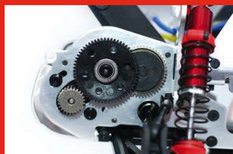
Side on of the motor plate showing the pinion, spur and layshaft gears
