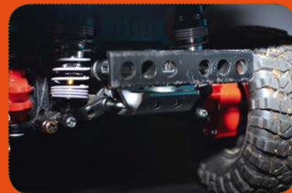
We fitted a set of Fastrax shocks all round
