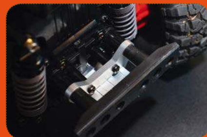
A Tamiya sump-guard was bolted on
