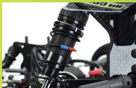
The PR Racing springs are identified using small pieces of heat shrink
