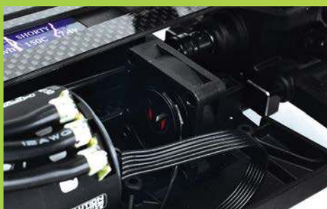
An additional fan was installed to draw hot air away from the motor
