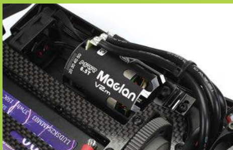
Maclan powered. We chose a MRR V2m 6.5T Sensored Competition motor for the SB401R-T
