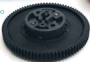
The spur gear is screwed to an adapter moulding
