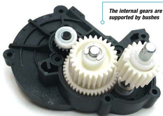
The spur gear is screwed to an adapter moulding
