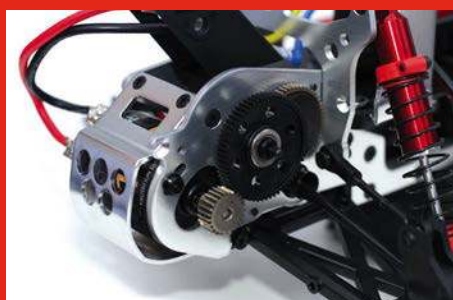
With the Absima Thrust B-Spec 19T brushed motor installed
