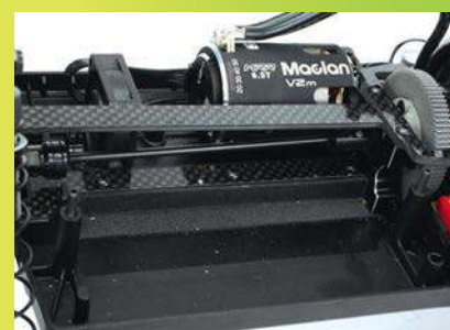
With the battery removed the moulded spine and lower carbon fibre braces can be seen
