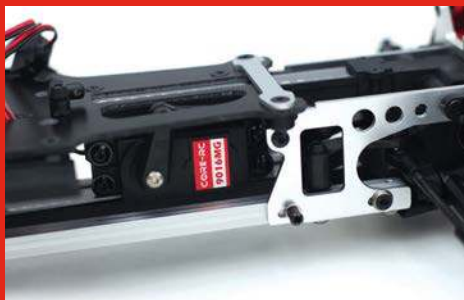
The steering servo is positioned above the channel where the chain (or belt) sits
