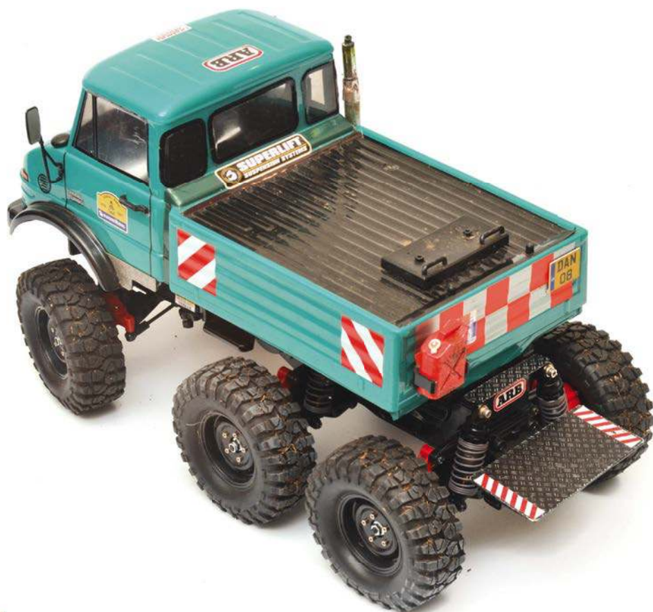
We fitted a set of Fastrax shocks all round
