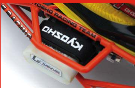
Kyosho-branded Velcro straps secure the battery in place
