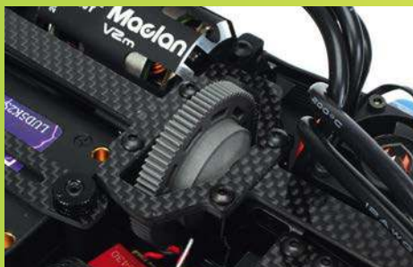
The grey plastics are used for the ball joint mouldings as well as the centre diff
