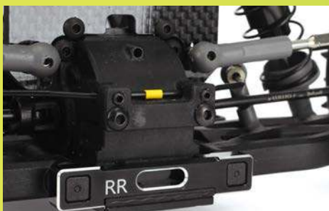
An insert system allows easy set-up changes to be made
