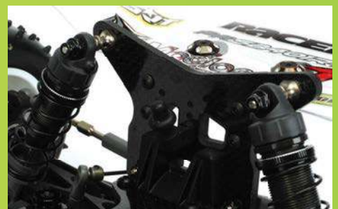
Carbon fibre features on both the front and rear shock towers
