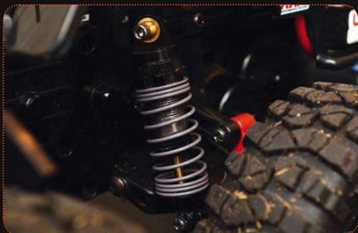
The Fastrax oil-filled shock absorbers feature threaded bodies
