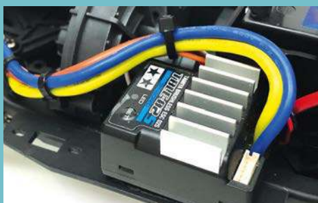
The included Tamiya TBLE-02S speed controller is 2S LiPo-compatible
