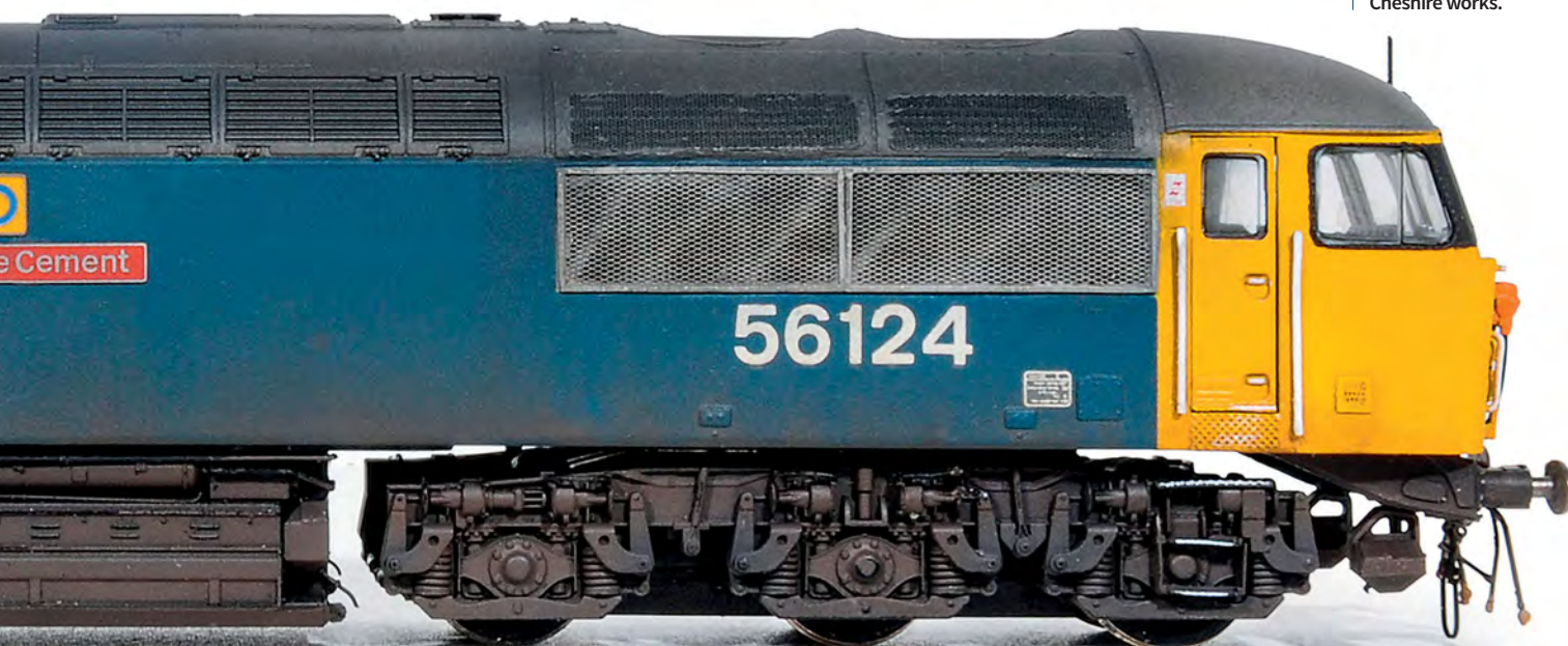
BELOW: The bodyside radiator grille and surrounding frame to be finished in Rail grey, which was a trademark of the 'Grids' painted in BR large logo blue by the Cheshire works.
