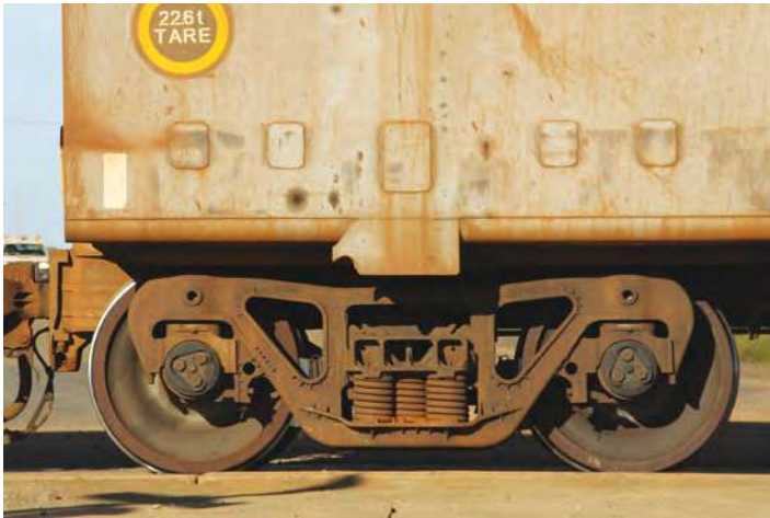
Right: The Builder's plate of a CNR ore car: 15 June 2015 Far right: The builder's plate of a CSR ore car: 15 June 2015 Below: The bogie of an empty CSR ore car departing Boodarie on 15 June 2015. The axleboxes and the pockets for the coil springs indicate that these bogies have primary suspension. Below right: The bogie of an empty CNR ore car departing Boodarie on 15 June 2015. The rubber pads above the axleboxes provide much the same reduction in impact forces as the coil springs on the CSR bogies, and allow limited steering of axles in curves. The mounting points of the diagonal braces are visible next to the bolster springs.
