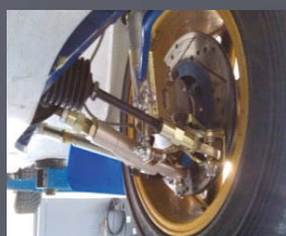
GRP4 MODULAR FRONT SUSPENSION
