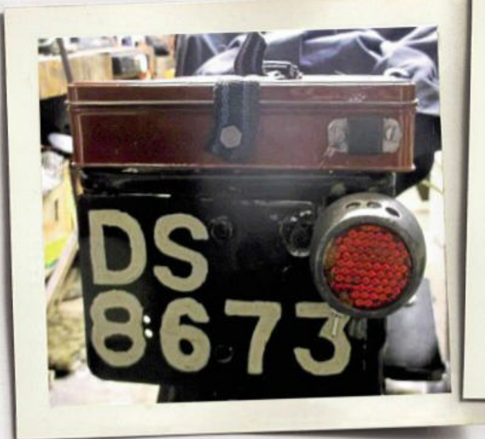
When the Invicta arrived it had been using a clip-on bicycle rear lamp, although also fitted with this old and non-working acetylene lamp shell. Oddly there is no door through which the gas could be lit, probably replaced by the modern plastic reflector. A little bracket on the new toolbox above will allow one of her cycle lamps to be clipped on
