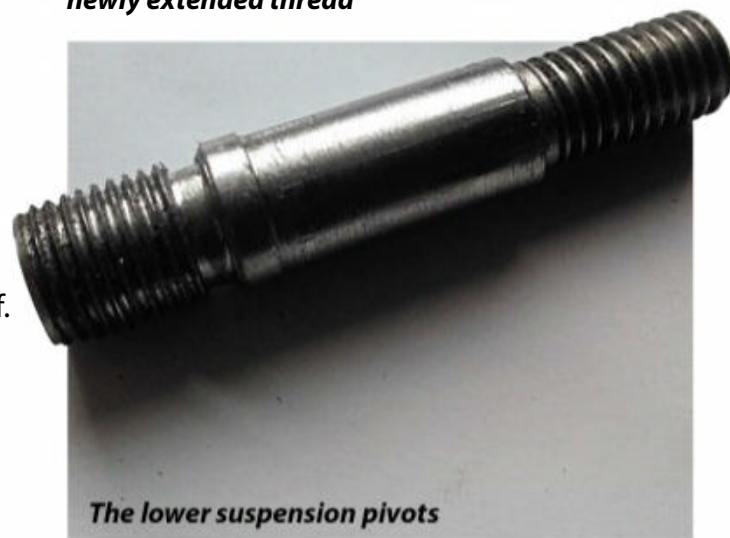
The repaired top suspension fitting, showing the newly extended thread
