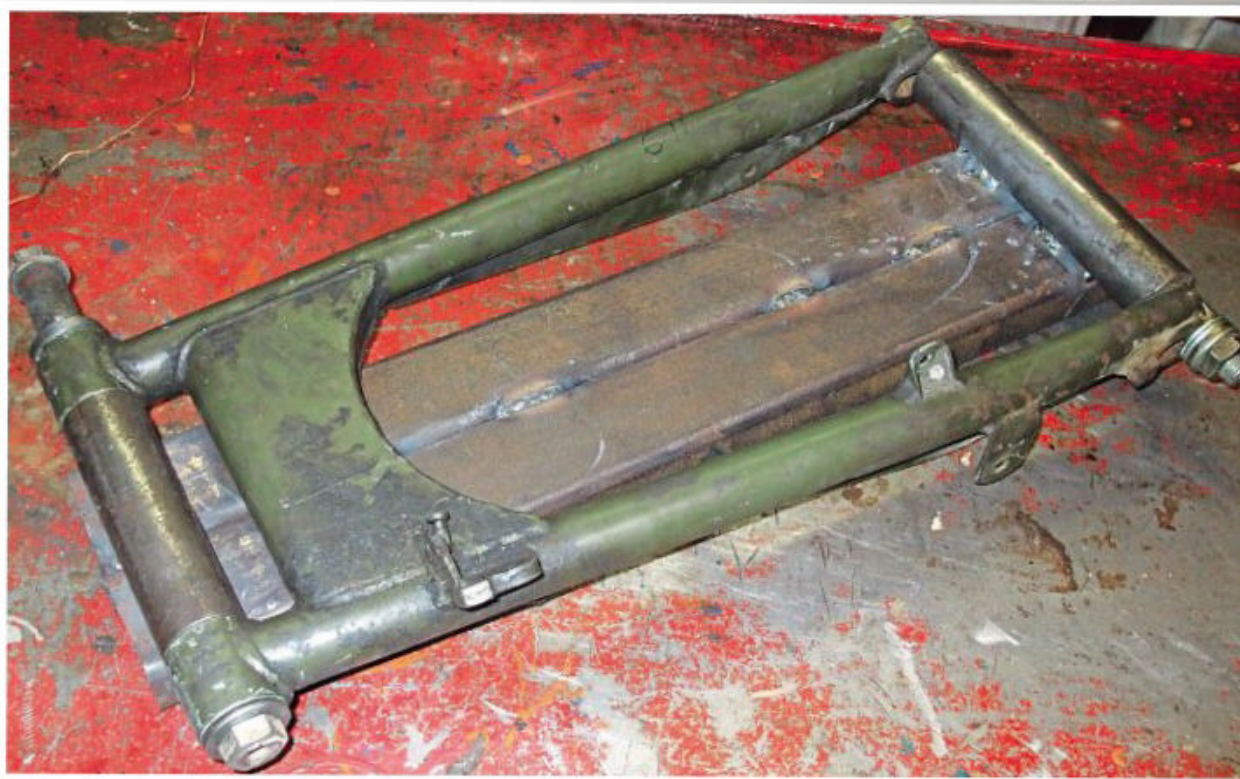
Here you can see the jig, two lengths of thick-wall box section welded together, and the two lengths of bar turned down to the correct width, bored to the spindle size, and clamped securely front and rear. That will now maintain the correct alignment of everything
