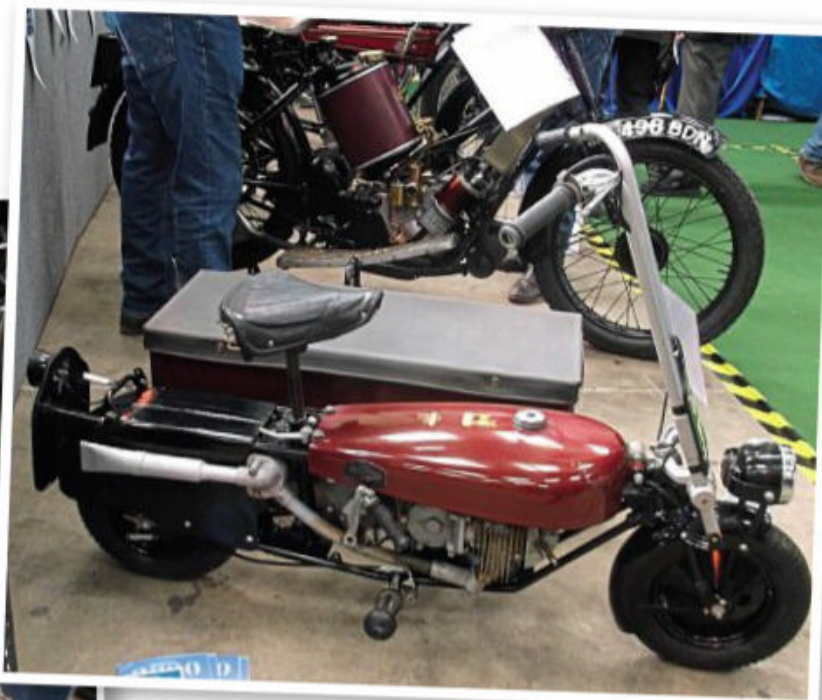
Back in the day Brockhouse really did list, and supply, sidecars for the 98cc Corgis. The Corgi, as everyone knows, is the same as a wartime Welbike. Well, it is except for the frame (different and longer on the Corgi), the wheels (discs on Corgi and spoked on Welbike), handlebars (Corgi single fold, but double folds for Welbike), petrol tank (saddle tank with gravity feed to carb on the Corgi and twin pannier tanks with pressure feed for the Welbike), and the engine (Excelsior 'Spryt' for the Corgi and Villiers 'Junior' for the Welbike). Yes apart from those 'little' differences they are the same!
