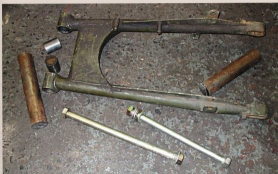
First order of the day is a new swinging arm, to save a little weight, but mainly to give a lot more adjustability to the wheelbase. The starting point is the original swinging arm, and two lengths of solid steel round bar. Note that I've already pressed out the swinging arm bushes from the front, as they have rubber inserts which won't take too well to welding. They'll be replaced with solid steel slugs which will stop everything moving as well
