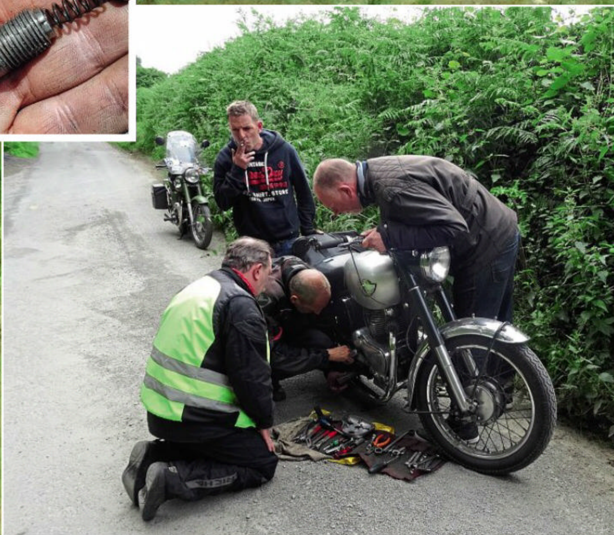
The culprit, an escaping detent plunger. Fixed by the roadside
