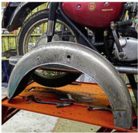
The new(ish...) guard FW found online. It's another Matchless mudguard, but is not for a G12CSR. It's bigger than the G12's and has a centre rib, too. Nicely patinated, however!
