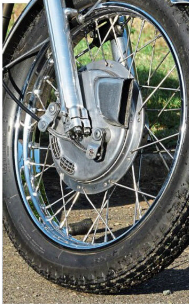
BSA-Triumph's often derided conical hub TLS brake. Very effective when set up properly. Stainless steel rim and spokes, as for the rear wheel also
