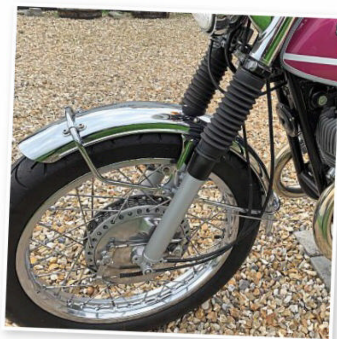
The T500 bowed out in 1975. It was replaced by the GT500 which looked much the same but boasted a disc brake up front and electronic ignition. The earlier drum looked nice and worked at least as well as the disc
