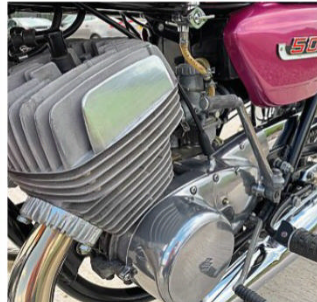
Suzuki's positive feed oiling system was considered more efficient than the lubrication on Kawasaki and Yamaha's two-strokes. The T500 should merely sip its oil, so if you find one that drinks lube then something is rotten in the state of Denmark...
