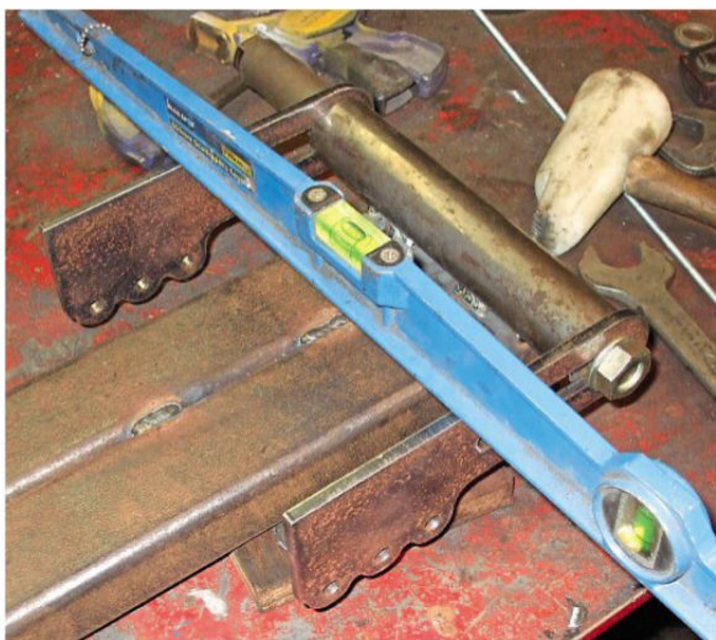
At the front I've cut the pivots off the old swinging arm and left them bolted them in place. At the rear here I've bolted up the new axle plates, cut from 6mm steel, and am just making sure they're both aligned correctly
