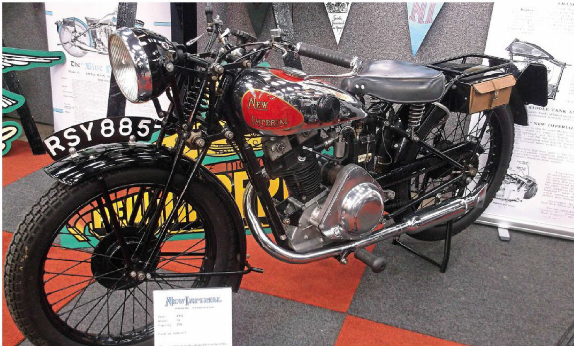
1934 model 30 New Imperial. This is a 250cc bigger brother to the more famous model 23 150cc bike, which gave good service and some of which were sleeved down for post-war 125cc racing. New Imperial adopted the more compact, and lighter, unit construction, like many continental manufacturers, whereas most of the British industry continued with separate gearboxes into the 50s and 60s
