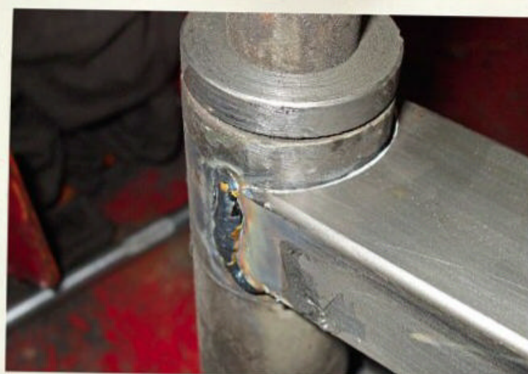
Here you can see the jig, two lengths of thick-wall box section welded together, and the two lengths of bar turned down to the correct width, bored to the spindle size, and clamped securely front and rear. That will now maintain the correct alignment of everything
