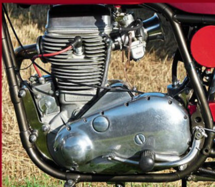
Very clean drive side using the original BSA primary chain cover
