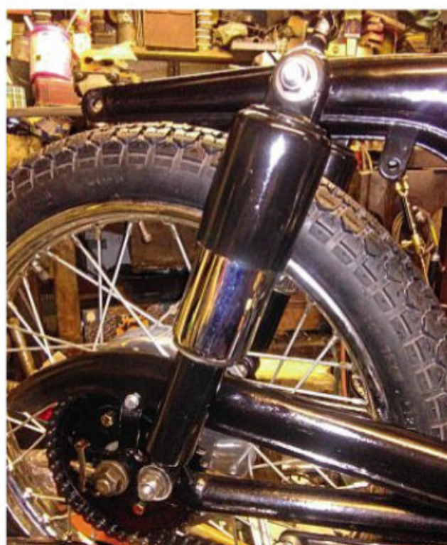
The little MV came without a chainguard, so John found some photos online and adapted a jumble find accordingly
