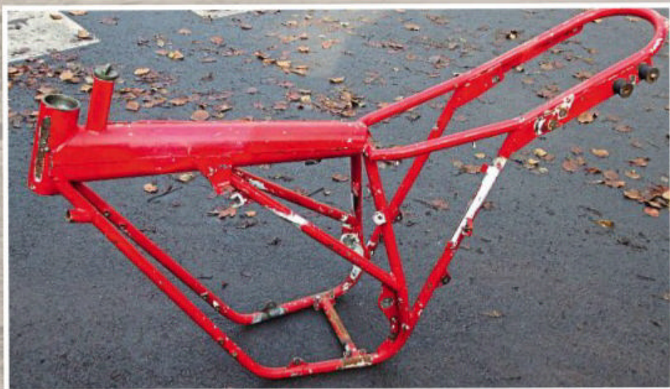
The starting point: one bog standard military Can-Am frame, for some reason with red Dulux covering its original Olive Drab
