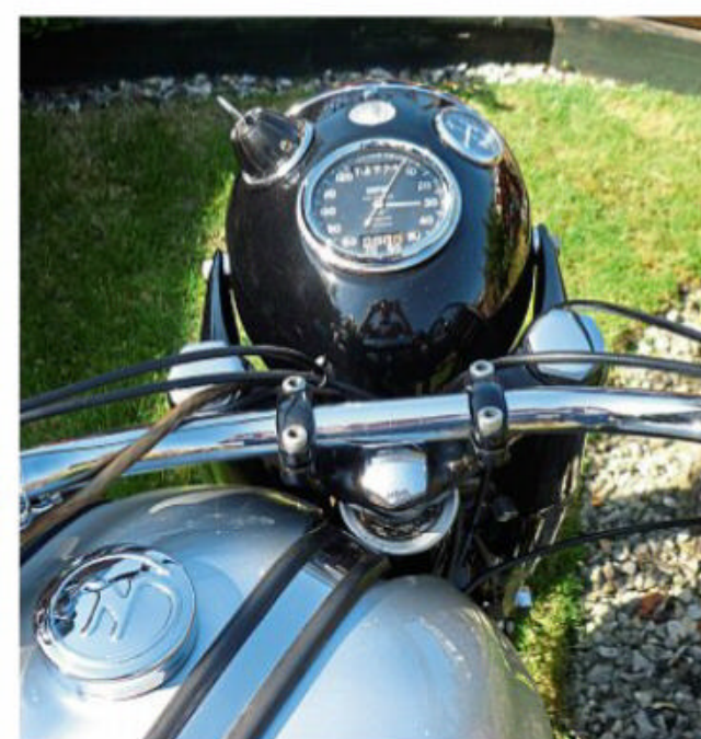
Flat Norton bars, with the choke on the right and ignition advance on the left. Lucas PRS8 switch and Smiths speedo share space in the headlamp shell
