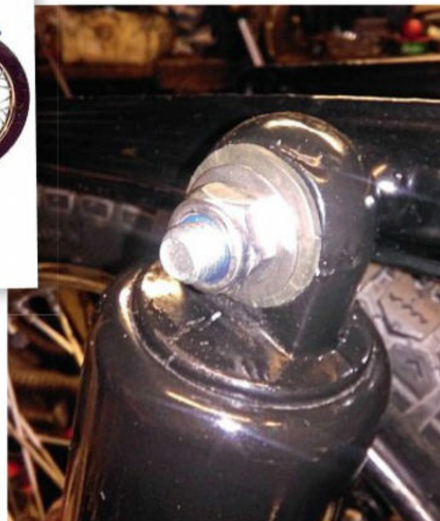
The repaired top suspension fitting, showing the newly extended thread
