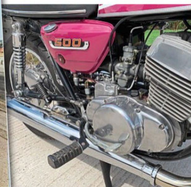
Unusually tractable for a modern two-stroke, the T500 will pull smoothly from 2000rpm in top gear. Vibes only start to become uncomfortable above 5000rpm when your foot could easily be shaken off the footrest
