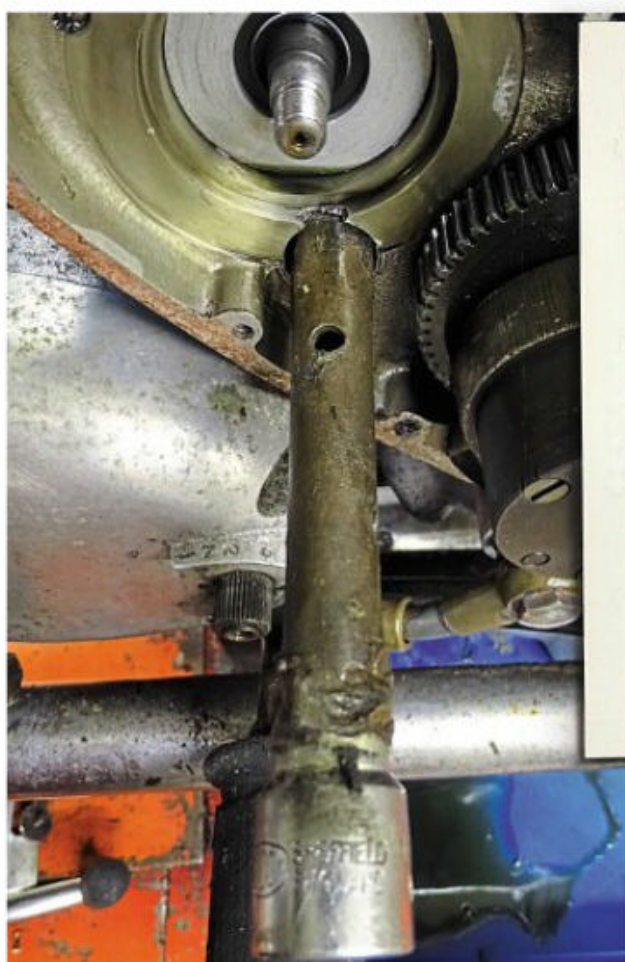
Sometime in the past, someone has struggled to remove the lower of the three magneto mounting fasteners. But FW has the correct (home-made) tool. Welding has never been an obvious skill, we observe
