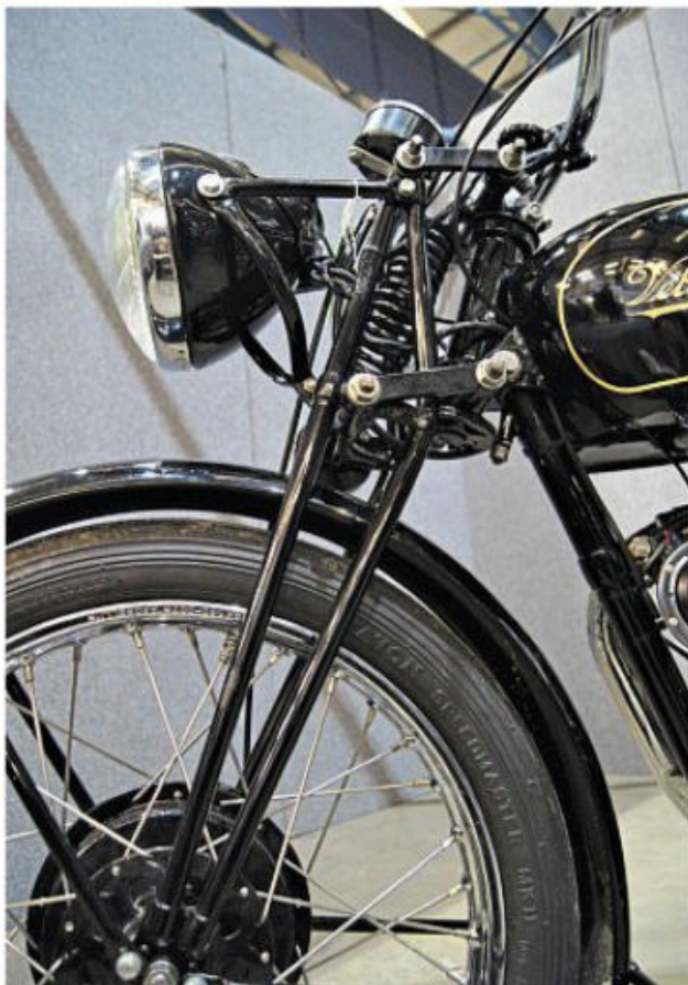
The MAC's Webb-style front forks weren't the cheaper type you might expect to find on a ride-to-work roadster, but were hand adjustable and fitted with a steering damper
