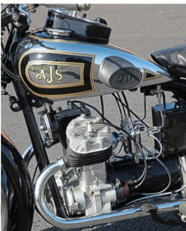
The AJS S3 is a sidevalve design, so it makes sense to hang the sides of the cylinders where the hot valves live out into the breeze
