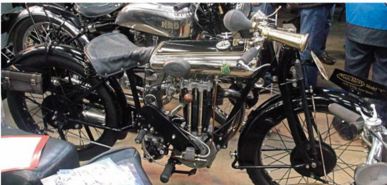
Brough Superior were not the only make to use long, shiny and bulbous saddle tanks in the 1920s. Here is one fitted to a Matchless 495cc ohv Super Sports model of 1926. It even sports BS-type tommy bar tank filler caps! Interestingly, neither of the two shiny tanks in this photo is chromed. The Matchless pre-dates the general adoption of chrome plating, so would be nickel, whilst Phil Vincent did not like chrome, so the HRD behind has an all stainless tank
