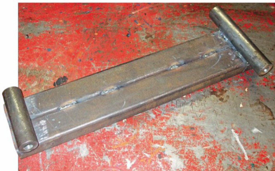
This gives a better view of the jig itself, with everything being welded securely in place
