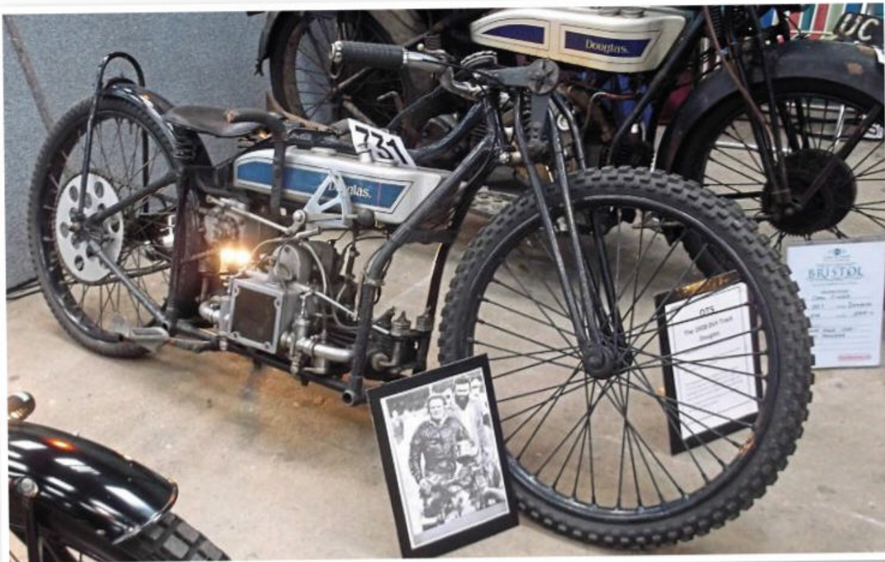
Long and low, the 'dirt track' Douglas (this being a 1928 500cc DT5) was the first king of the tracks, with riders using a leg-trailing style, before JAPs eventually changed and dominated the sport. It cost £85 and a factory tuned engine might produce 32bhp
