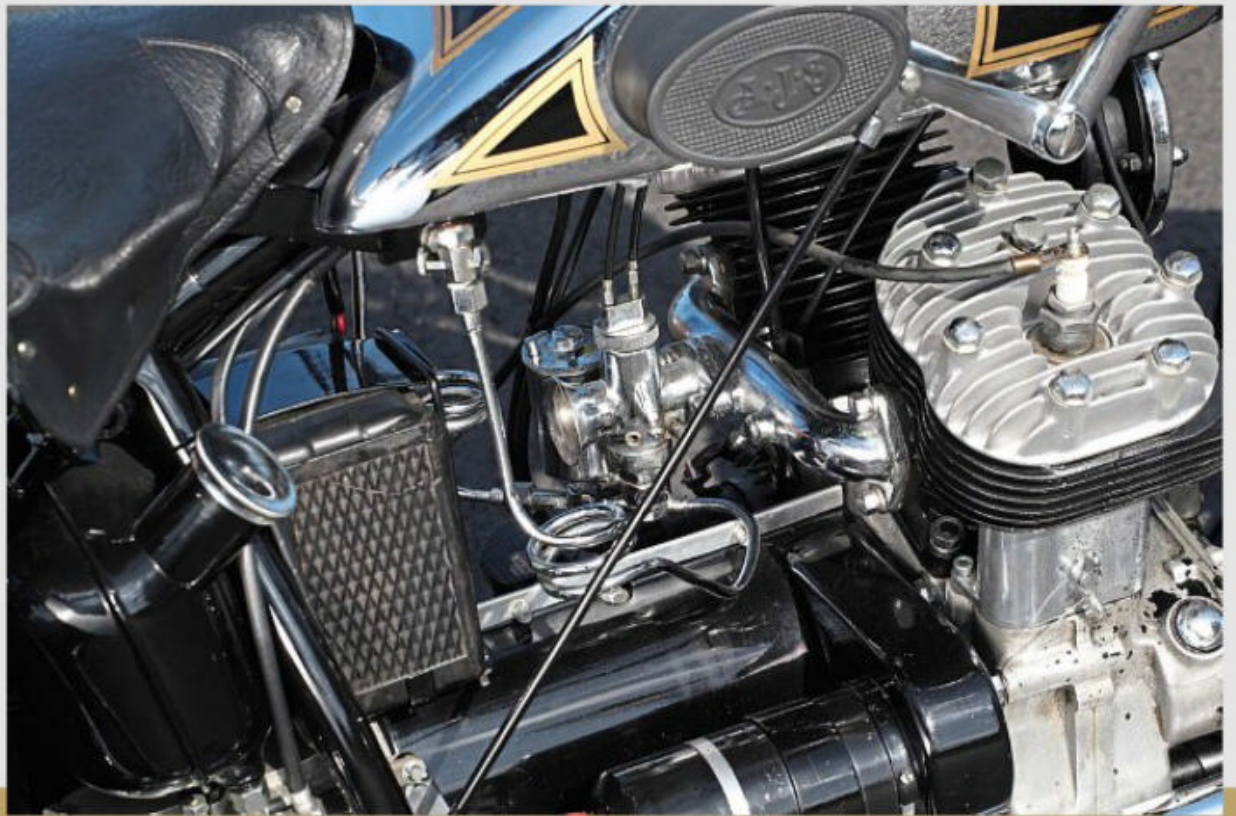
Layout is logical. A single carb feeds the engine, while the gearbox lives directly behind it, with the battery above
