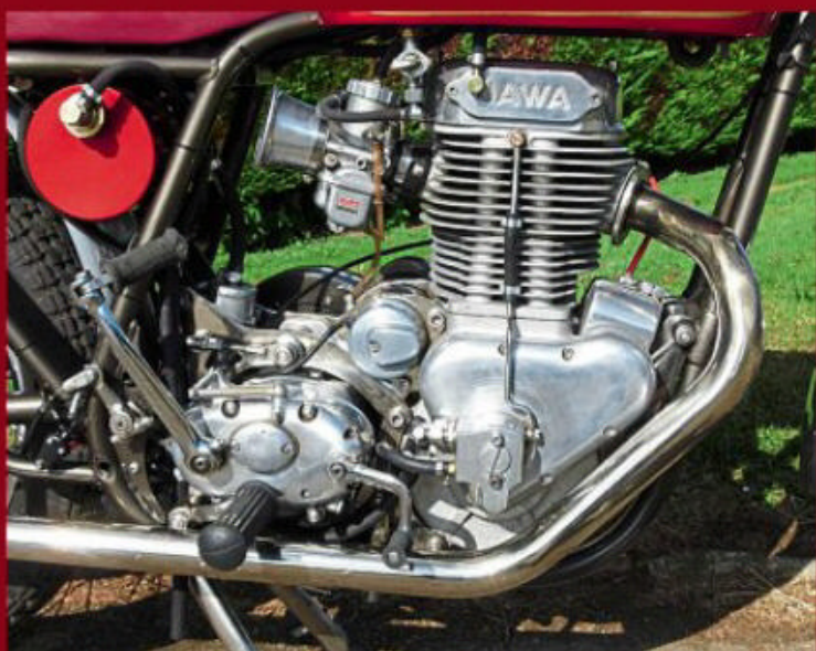
The heart of the matter. David's oil pump with rocker box feed and breather by the 'J'. Magneto up front and dynamo behind
