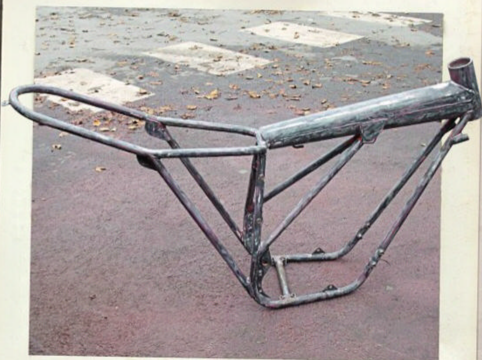
It's surprising just how much weight you can lose just by removing superfluous brackets. Note also the removal of the long bracing bars that carried the silencer and supported the subframe, and the elongated oil tank filler stem
