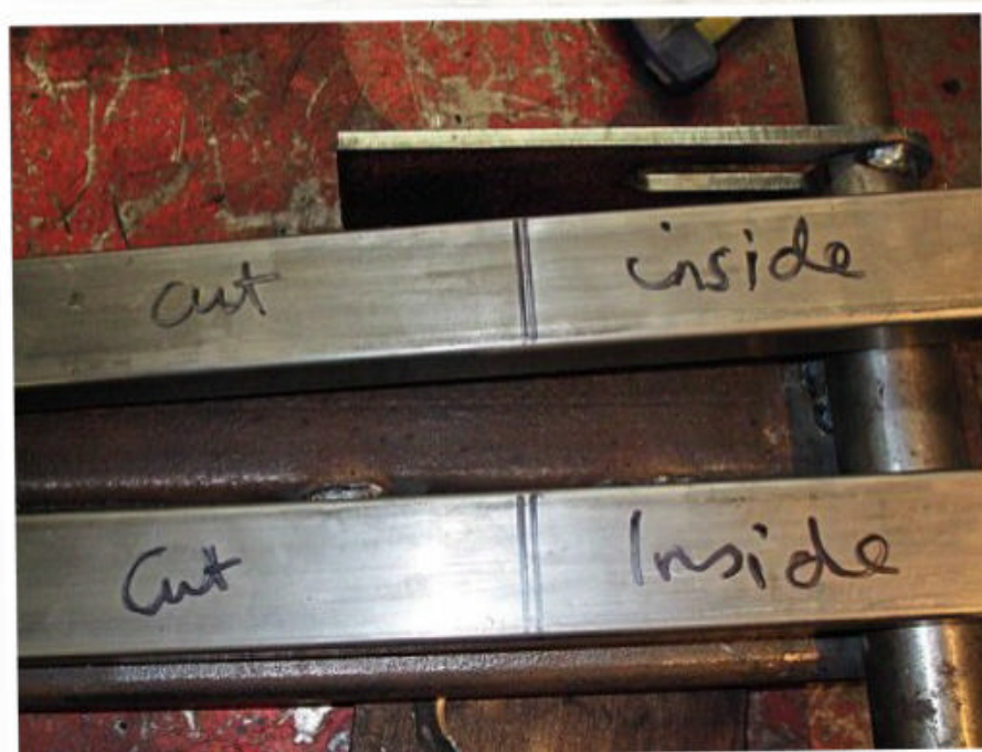
It's very easy to make simple mistakes on simple jobs. I've learned to mark things as I go along, in this case the cut marks on the box section. You might think it's impossible to make two rights or two lefts instead of one each, but it isn't (don't ask me how I know that...)
