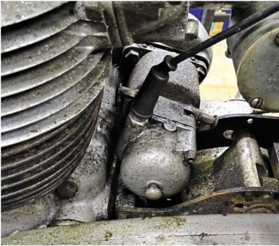
While pondering the anorak delights of AMC rear mudguards. FW decided to remove the sparkless magneto. Here it is now. Observe the cunning shrouded retaining nuts
