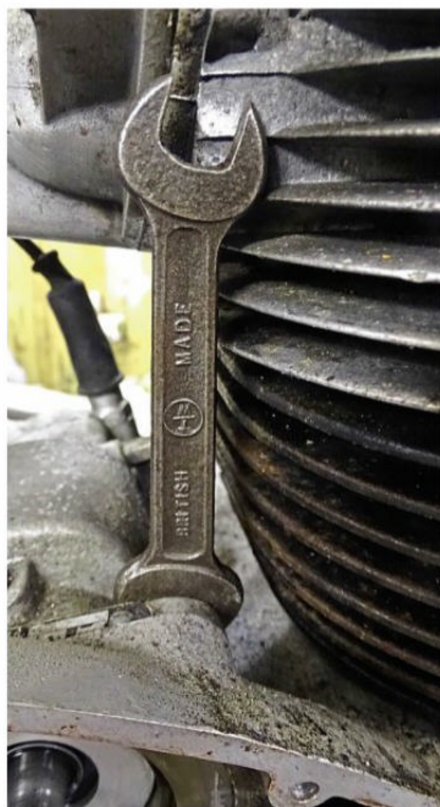
But finally, the unexpected halt. There's no room to move the spanner, and neither a ring nor a socket will fit
