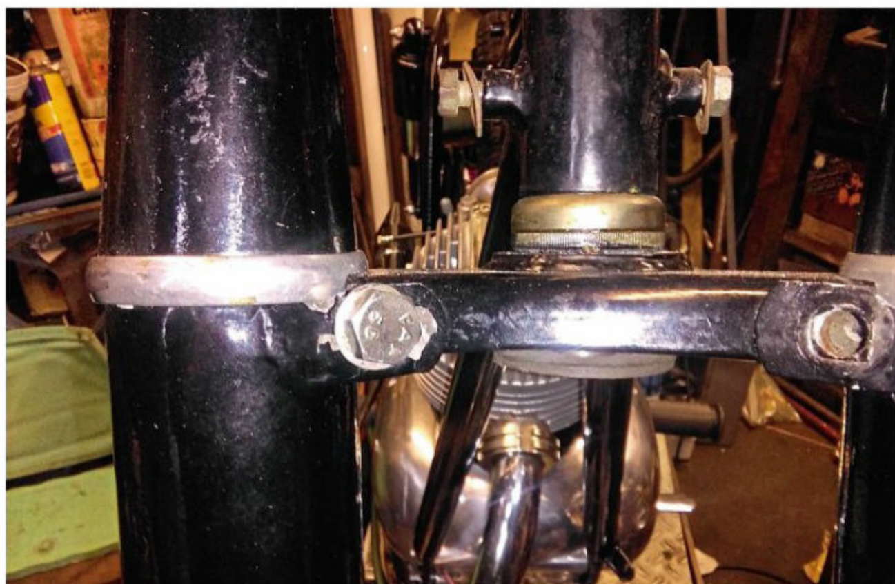
The fork pinch bolts replacement
