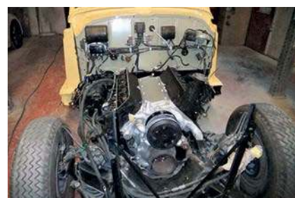
The car's engine and gearbox were stripped and rebuilt during the restoration
