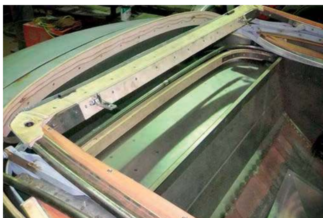
Thanks to Tony's ingenuity, the Silver Cloud's hood folds extra-low for good visibility
