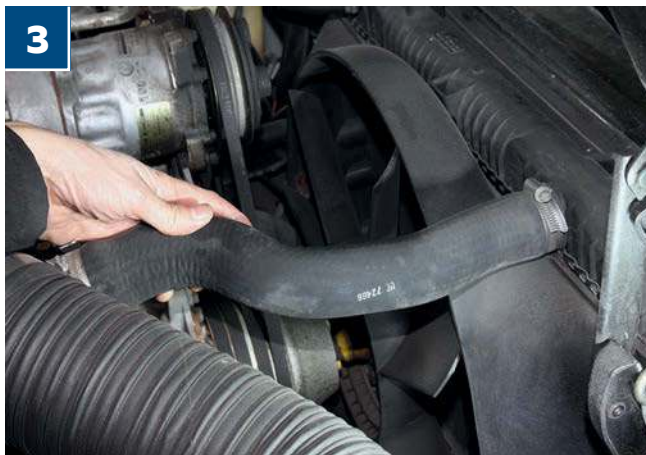
Rubber coolant hoses can perish during cold weather, resulting in leaks. When the engine is cold, pinch each hose to look for cracks. Check that all hose clips are secure, but avoid overtightening them, which risks cutting into the rubber.
