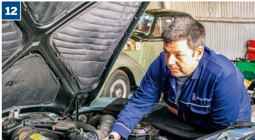
Daniel confirmed engine timing was as close to perfect as it could be, ruling out another possible cause for the presence of the blip under load; it was time to raise the car in the air for further scrutiny, as well as for an impromptu oil change
