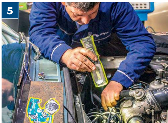
5 The time-served Rolls-Royce & Bentley specialist started by inspecting the new ignition components in order to rule out incorrect installation or faulty equipment
