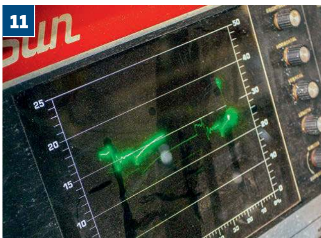
11 Aha! There's the little blighter, over on the right. It's a very occasional misfire, hardly noticeable on idle, but Daniel's trusted diagnostic equipment proved we weren't going mad
