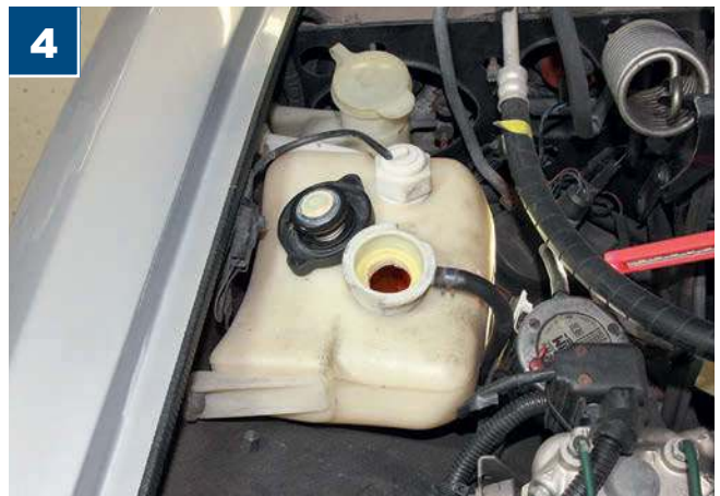
The coolant expansion tank is located on the nearside front of the engine bay. There are minimum and maximum markings on the side to help check the level. Top up with whatever colour of coolant has been used before.
