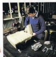
Far left. Perfectly matched holes of Connolly leather are carefully marked out and cut individually.
