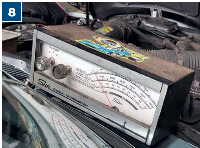
8 ...and his dinky Dwell Tachometer. Keep it steady Dan, and whatever you do, don't accidentally knock that shift lever into Drive mode, else that Twenty is going to need even more restorative work!
