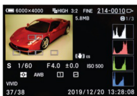
▲ Replay screens include a thumbnail with a full set of histograms. The right-hand panel can be cycled through a number of additional info displays.
