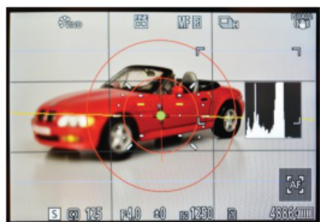
▲ Live view screen can be configured with quite a number of elements, including the novel 'I.S. Status Scope' and a dual-axis level indicator (left), or exposure compensation scale and real-time histogram (right).
