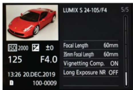
▲▼ The review/replay split screen can be cycled through (from left) additional capture data, a set of RGB and brightness histograms, the 'Photo Style' parameters, the white balance mode with any fine-tuning settings, and the lens details, including the in-camera corrections.
