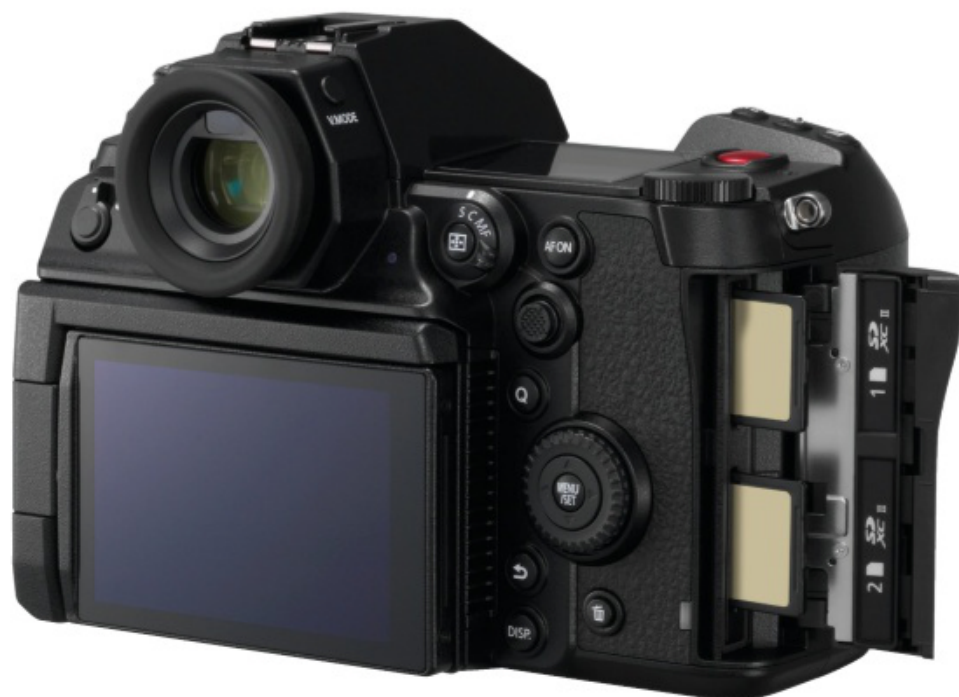
▲ Dual card slots are both for SD format devices and both have UHS Speed Class 3 and UHS-II Speed Class 90 support.
