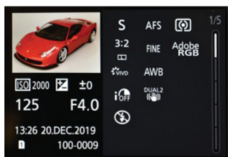
▲▼ The review/replay split screen can be cycled through (from left) additional capture data, a set of RGB and brightness histograms, the 'Photo Style' parameters, the white balance mode with any fine-tuning settings, and the lens details, including the in-camera corrections.
