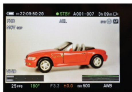
▲ Live view screens automatically switch between photo and video displays, the latter including a waveform graph (lower right).
