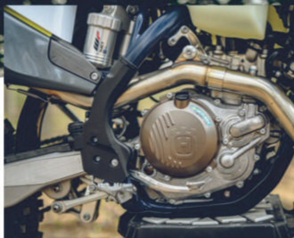
Two-piece header is easier to remove
