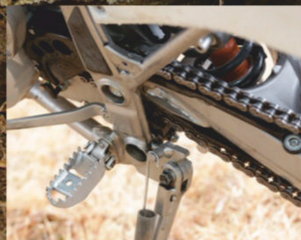
Subframe is steel and not removeable
