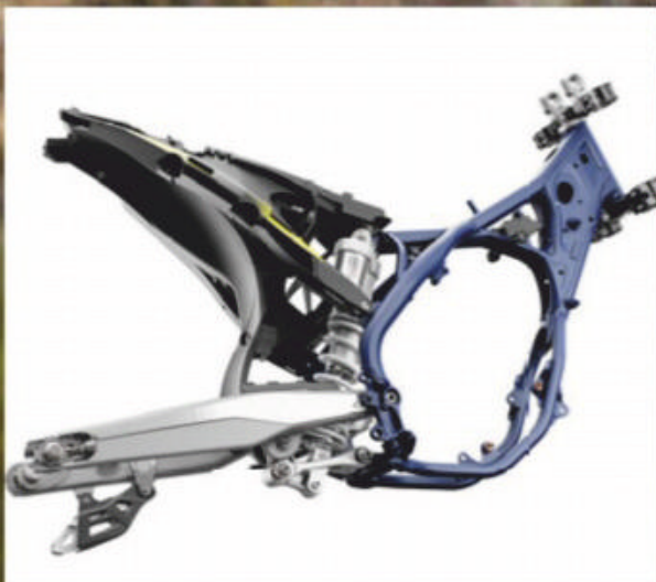
Carbon subframe is now two pieces and lighter
