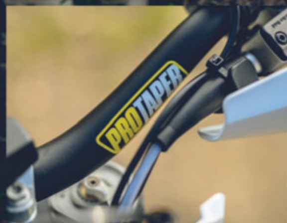
Pro Taper handlebar and Magura clutch
