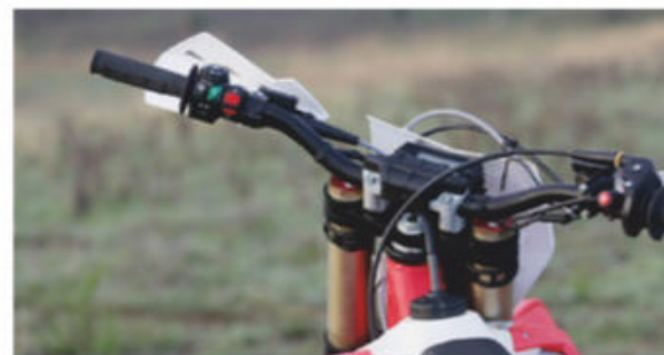
EC300 runs Neken handlebar and a map switch
