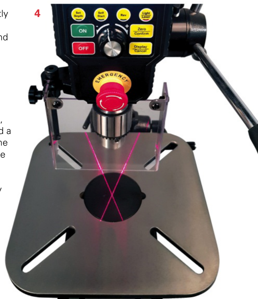
4. Large 16mm quill, safety guard and adjustable laser.
