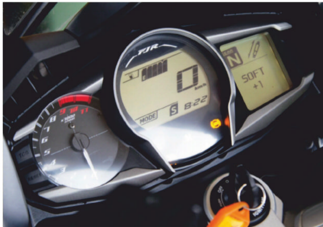
Analog tacho, digital speedo, LCD info panel – easy to read and use, although not as fancy as many bikes these days.
