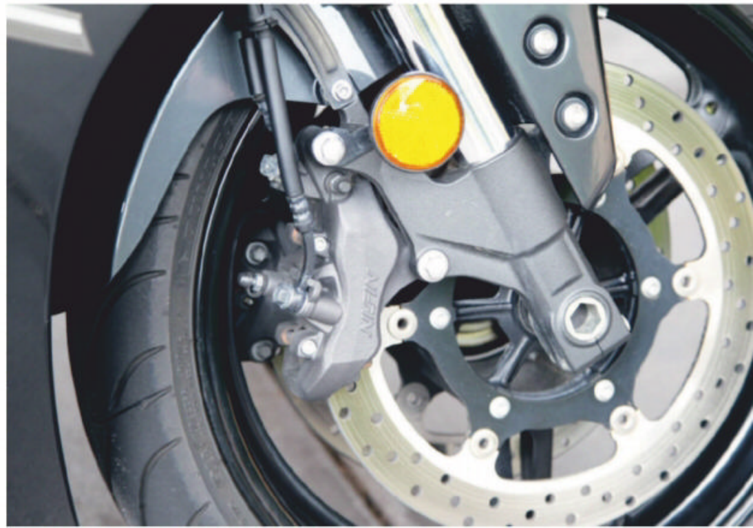
The FJR's brakes are only OK, hard braking riders may want to look for pads with more bite.
