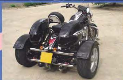
Kawasaki VN1700 with chain drive conversion, panniers, stainless bull bars, tow bar.
