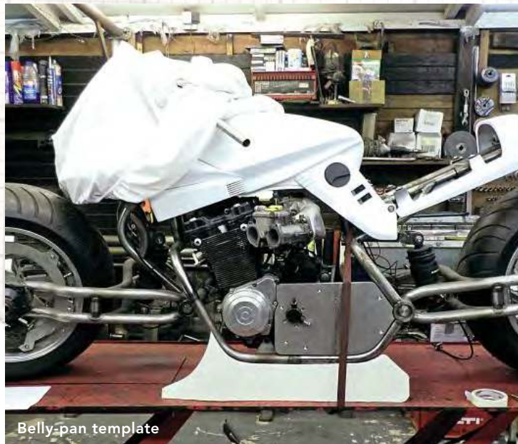
Sides and front welded together
