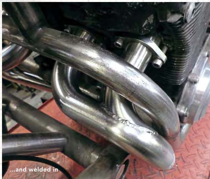
Slip-joint to make Nos 3 and 4 join up with 1 and 2
