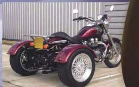
Triumph Bonneville America with reverse transfer gearbox, stainless rack, electronic gear shifter.
