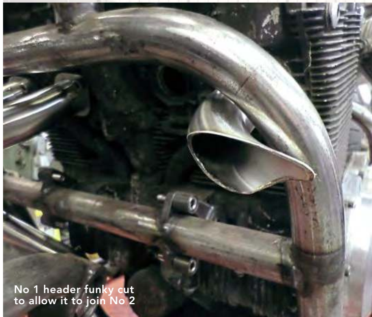
Roughly cut hole in No 2 to take No 1 header
