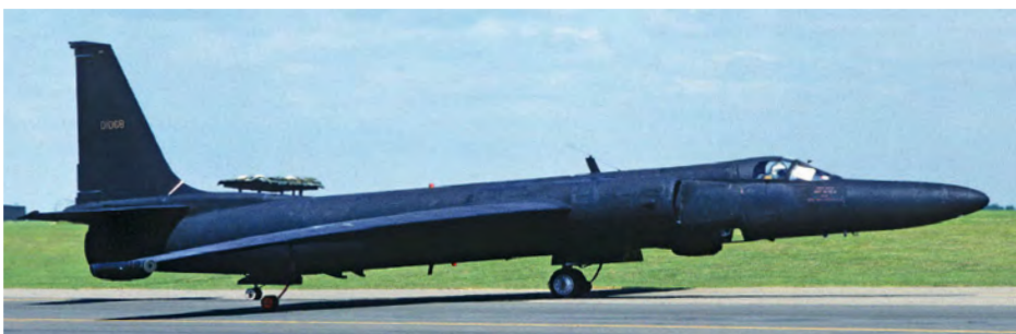
The KA-80 camera was sometimes fitted and its window is visible below and behind the cockpit of this TR-1A at Alconbury. Peter R Foster
