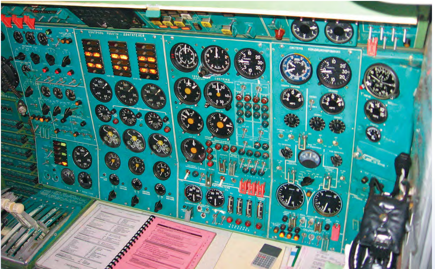
The Tu-154M flight engineer's workstation, crammed with instruments for engine and systems monitoring and control. Alexander Mladenov
