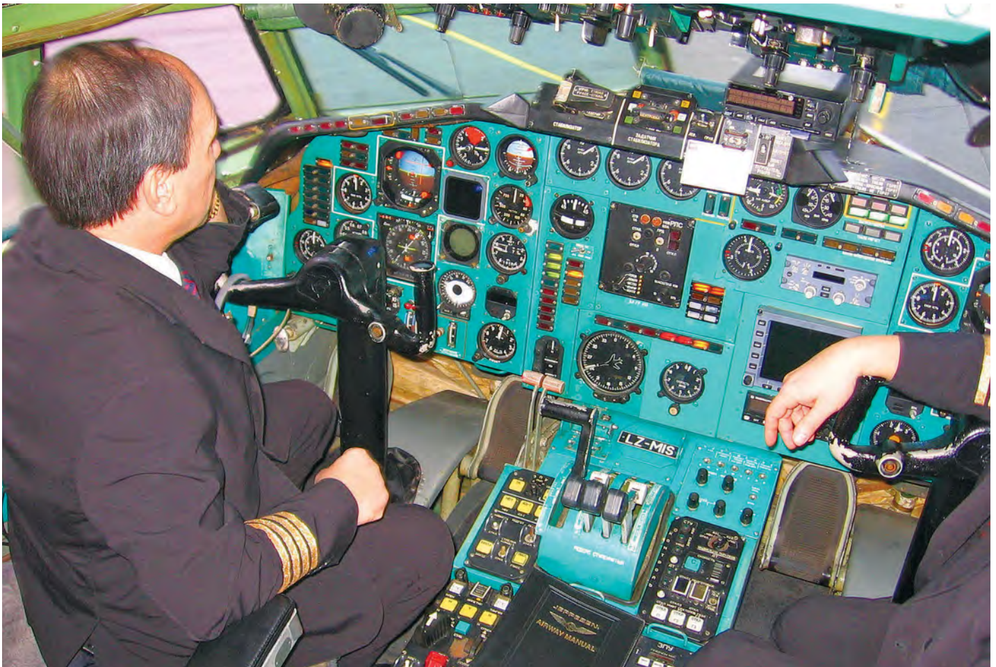
The Tu-154M's cockpit offers a 1970s-vintage working environment for the three crew members, comprising the pilot, co-pilot and flight engineer. Alexander Mladenov
