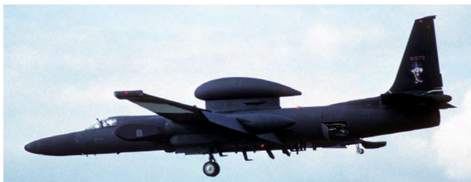
Sporting the large Senior Span antenna and chalk tail art, TR-1A 80-1070 lands at Alconbury in April 1989. The system allowed direct transmission of data to satellites. Peter R Foster
