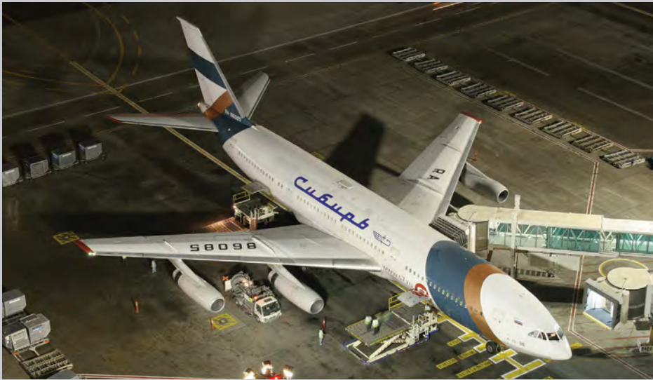
Sibir or Siberia Airlines, now operating under the S7 brand, had a fleet of nine Il-86s. All of these were grounded in August 2009 due to their excessive fuel consumption. AirTeamImages.com/ Serge Baileul
