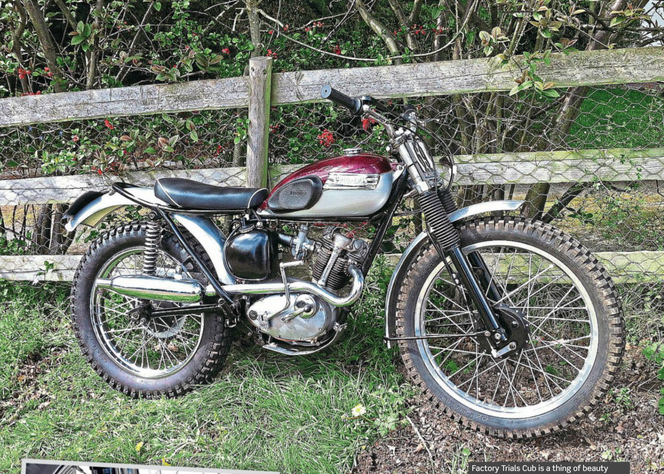
Narrower tank helps slow speed balance
