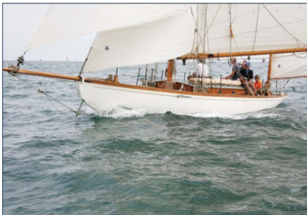
40' Alfred Mylne Island Class gaff yawl built in 1913 by John Hilditch. Total rebuild completed in 2015, hull repaired, new deck, rig, interior and systems. Mahogany and Pitch pine on oak, all bronze screwed. All hollow spars by Collars. 6 berths in new interior with good headroom. A beautiful and professionally rebuilt yacht, raced and cruised by the family in recent years, currently afloat and in commission. Devon £99,000
