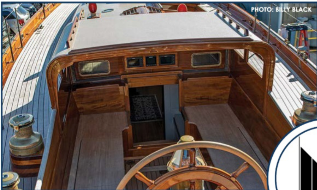
Kirawan's deck layout with refurbished cabin, signature doghouse, butterflies, new handrails, deck, caprails, coamings, bronze pedestal, wheel, winches and hardware i.e. "the works".
