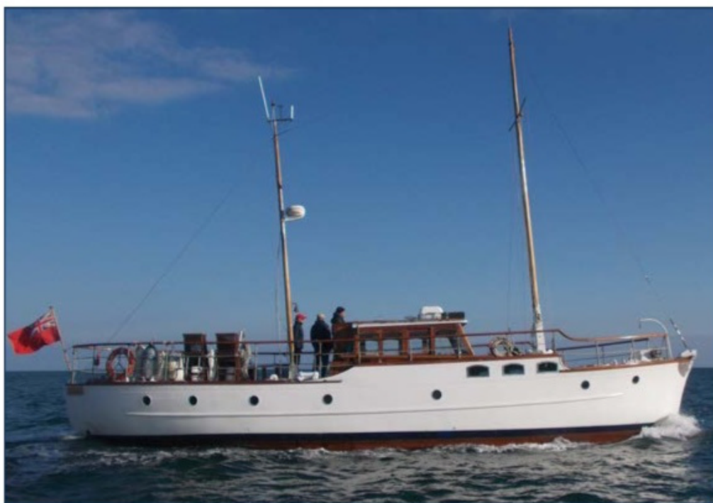
48' Mclean and Sons Motor Yacht launched in 1935. Major professional rebuild in current ownership including new decks, wheelhouse and lots of interior. Pitch Pine on oak hull with new teak on plywood decks. Twin Beta 90hp diesels fitted in 2005. 6 berths in 3 sleeping cabins with possibility for more. A very elegant motor yacht in good structural condition, in need of some minor works before launching. Wales £135,000
