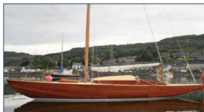
23' Varnished Day Boat built in Scotland and professionally rebuilt in 2013. Mahogany planking on steam bent oak timbers, sheathed plywood deck new in 2013. Large cockpit with a cuddy and space under the foredeck. Fractional bermudan sloop rig in nice condition, new genoa 2018. RM road trailer, new 2016. Smart boat, well equipped and apparently a joy to sail, a very easy and enjoyable way of getting afloat. 2018 survey. Cornwall £10,950
