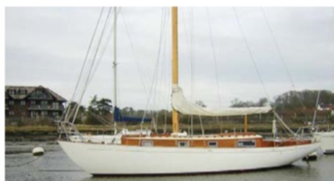
34' Buchanan Saxon sloop built by Priors in 1962 to Lloyds 100A1. Mahogany on CRE frames with a sheathed plywood deck and teak superstructure. Perkins 30hp diesel. 5 berths with good headroom and smart interior joinery. Superb example of the class, very nicely presented and ready to sail this season. recent survey available.
