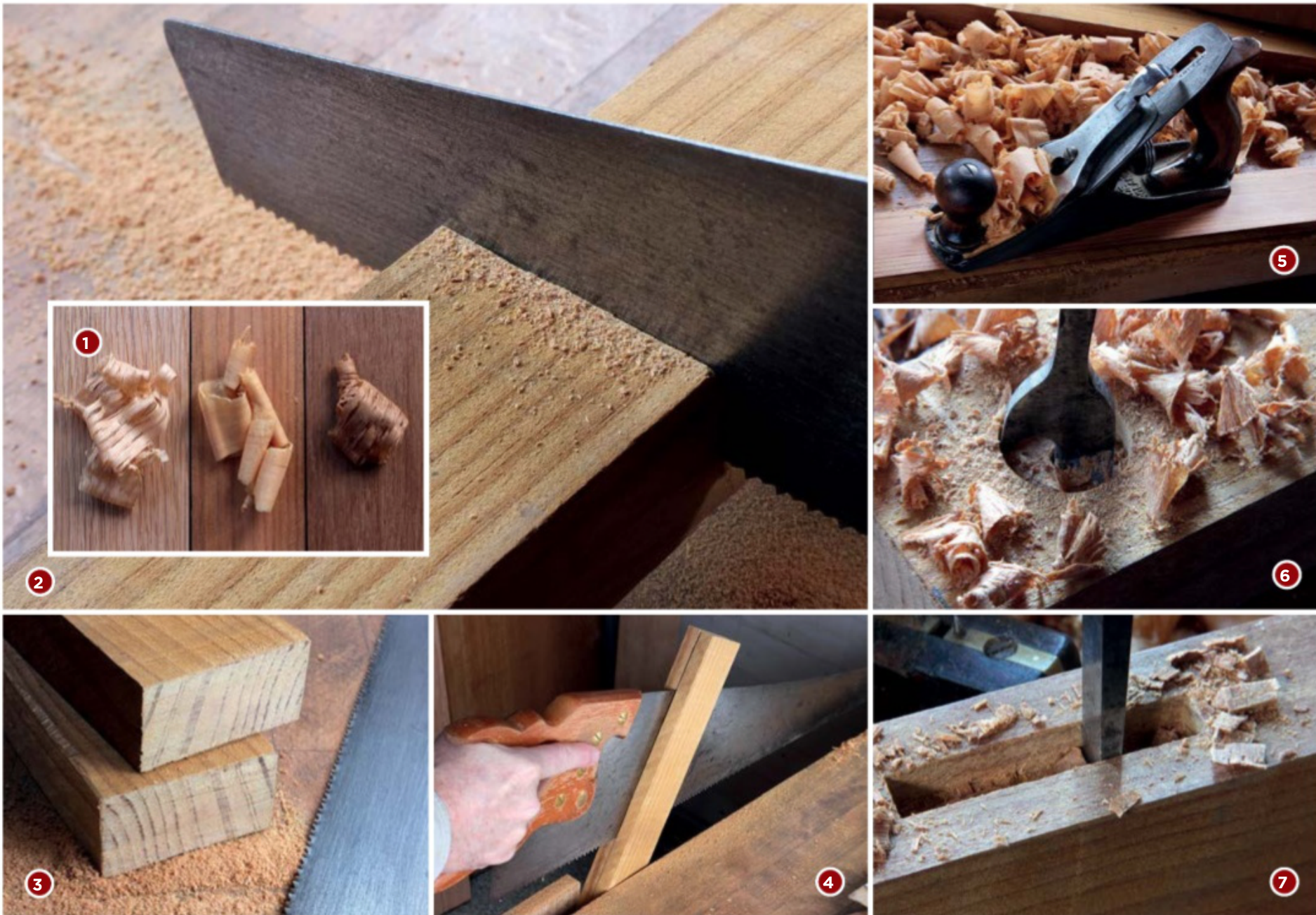
1 Lignia Yacht (centre) flanked by English oak (left) and teak; 2 Cutting to length with the panel saw; 3 Sawn ends show wide-apart growth rings; 4 Cutting lengthways with the rip saw; 5 Planing faces with the No 3 smoother; 6 Clean-cut edges with a centre bit; 7 Chiselling a mortise
