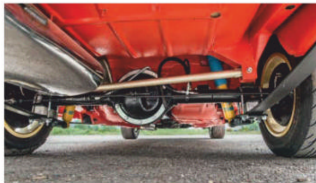
The Escort's now running an Atlas axle with 3.7 gears.
