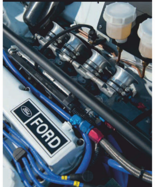
Compact GSX-R600 throttle bodies are off the Zetec mounted using a modified ST170 inlet.
