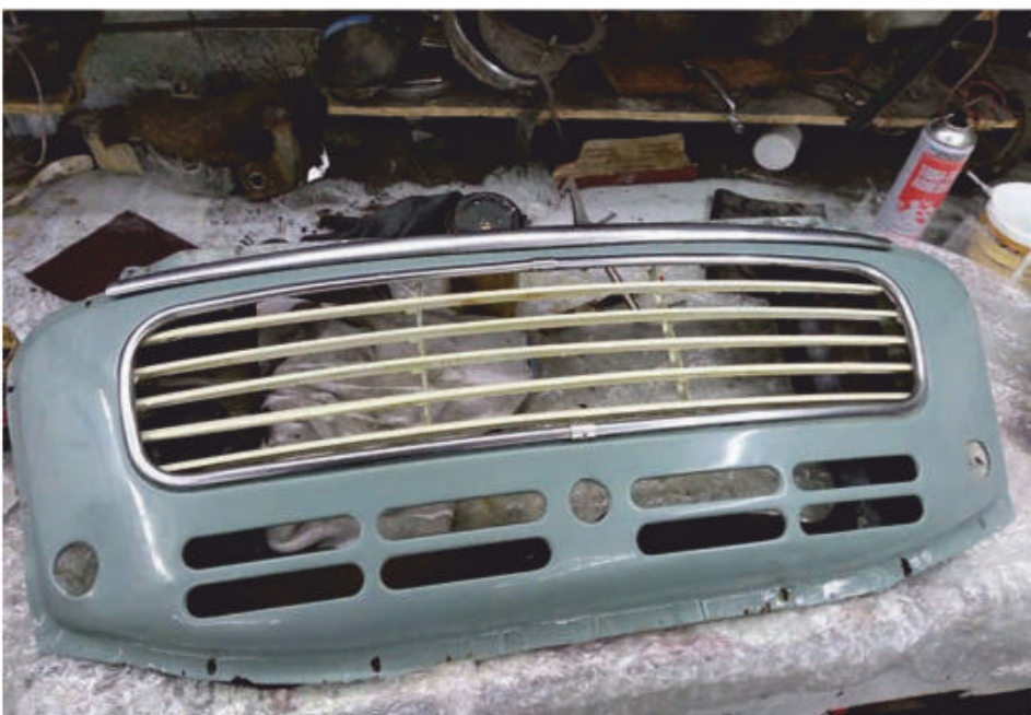
Front grille re-assembled and ready to fit onto the front of Lily.
