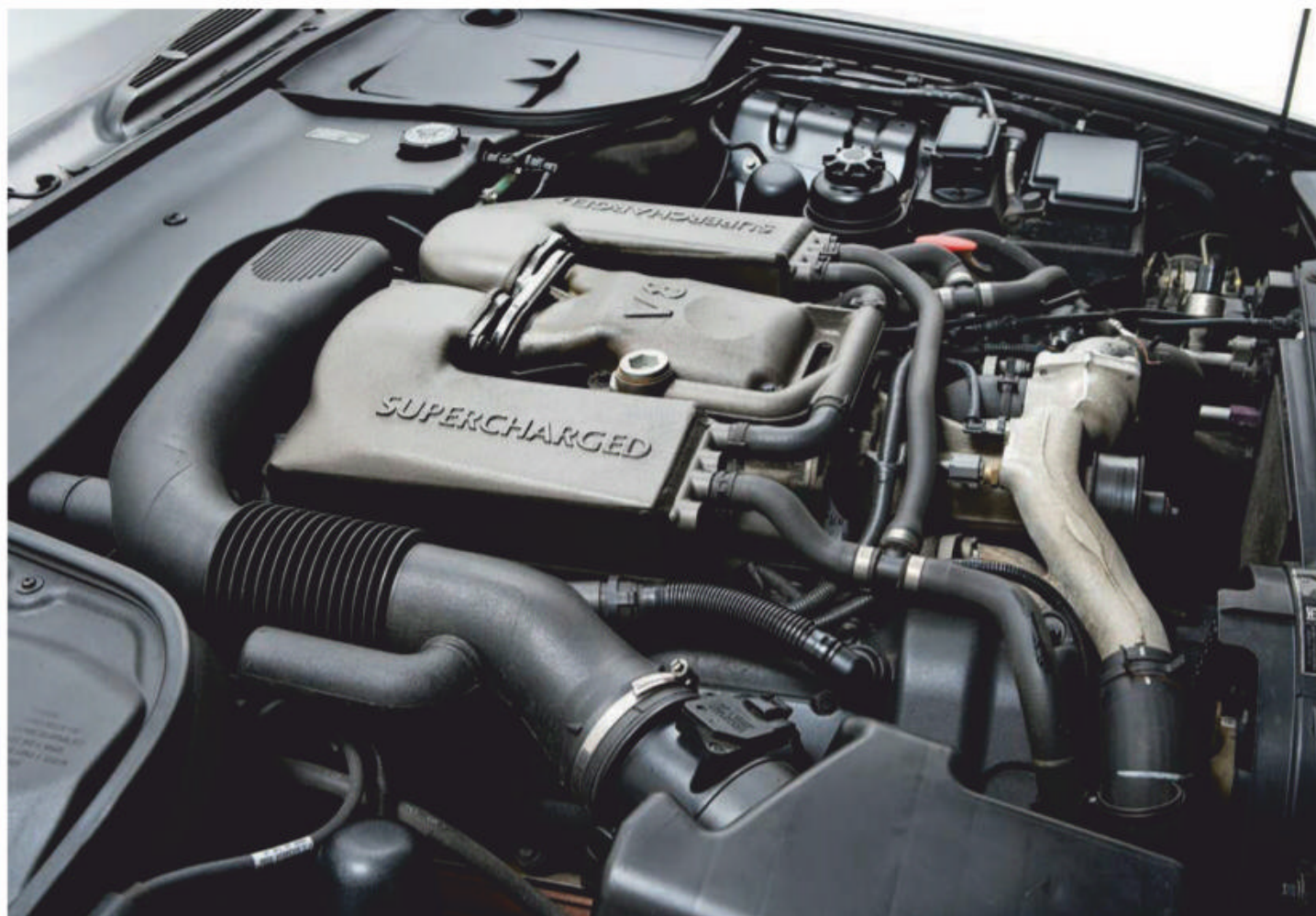
The supercharged 4.0-litre V8 in the XJR produced 370bhp and 387lb.ft of torque. There was no manual gearbox option, nor was a limited slip differential offered. 0-60mph times were just 5.6 secs.
