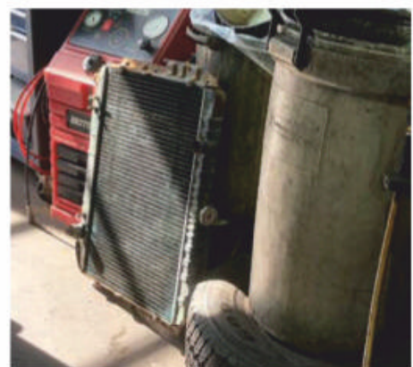
Transmission cooler inside the rad has split, allowing coolant to get into the transmission. It looks like the 1984 original, so complaining is unreasonable.
