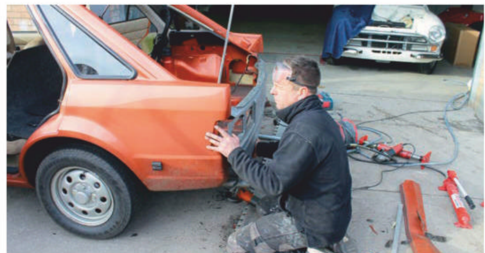
Lining up the new back panel to gauge where we would be at the end, before final cleaning up of edges prior to welding.
