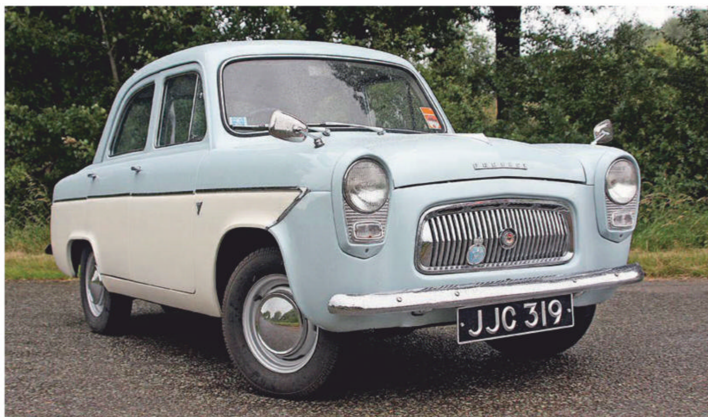
The 107E was faster, accelerated more quickly and was more frugal than its sidevalve predecessor.
