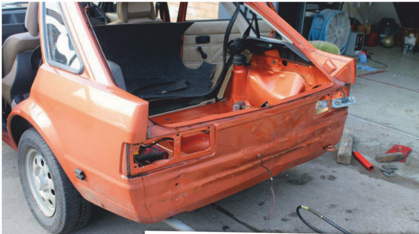
ABOVE AND RIGHT: Hydraulic ram was used to ease the back panel straight again.
