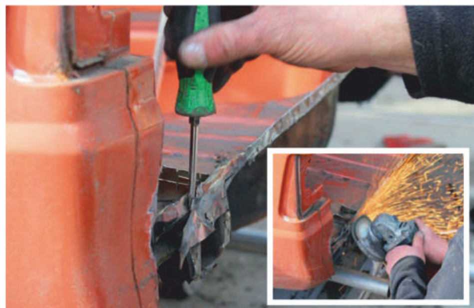
Ford's welds were so tidy and have lasted so well that Paul had to thin the metal before prying this section away.
