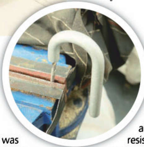
ABOVE: Not a pretty sight – the hidden part of the overflow pipe had seen better days.
