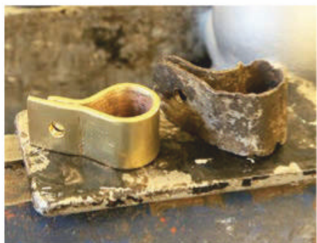
The replacement over flow pipe clip which Peter bent to shape after warming it up on the cooking hob.
