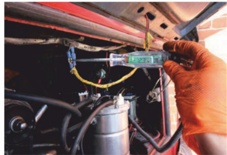
Compact circuit tester from Rally Design costs £15.48 (part number SWE652) and helps with checking for live earth wires as well as testing battery voltage. An essential tool for solving electrical problems.
