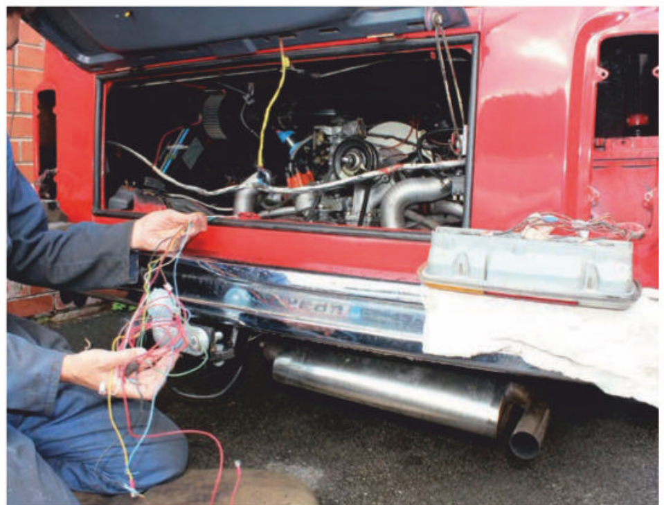
With a vague knowledge of vehicle electrics, Rob followed the instructions and wired up the electrics for a seven-pin socket.
