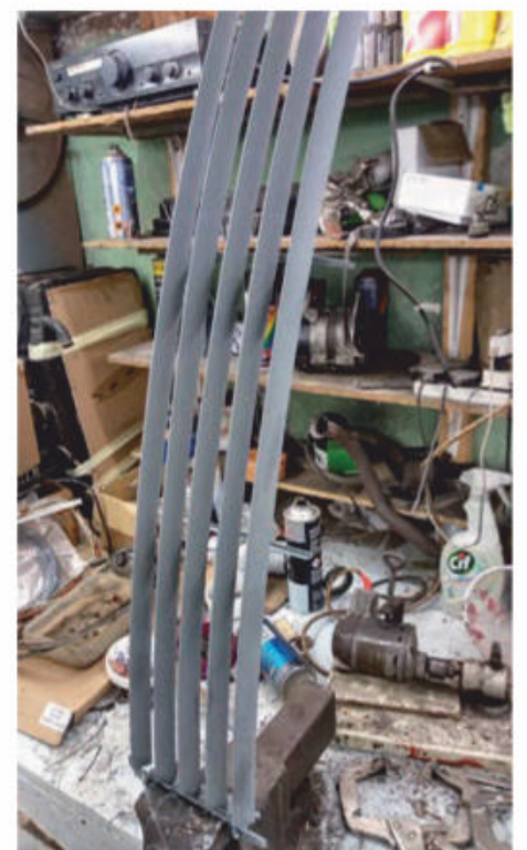
The rusty front grill was de-rusted and repainted in zinc primer.
