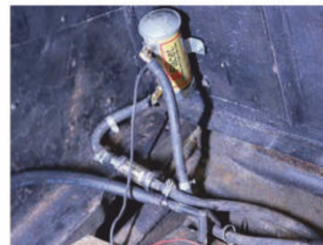
The old fuel pipework with the new overflow hose temporarily placed on.
