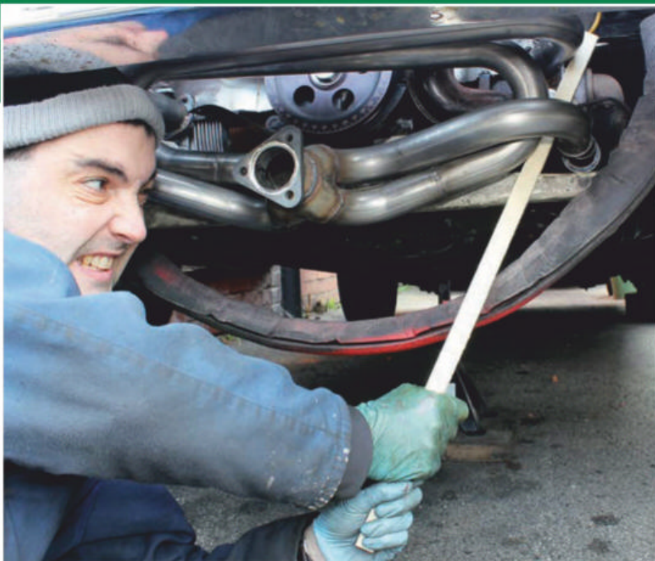
Brute force or ignorance? Rob could have slackened the exhaust manifold nuts and saved himself from swearing.
