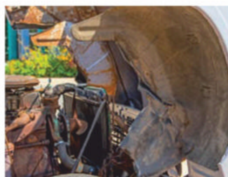
ABOVE and BELOW: The Herald was powered by Standard-Triumph's rugged and well-proven SC (Small Car) engine which had debuted at 803cc in the Standard 8 of 1953. Access to it in the Herald was superb.
