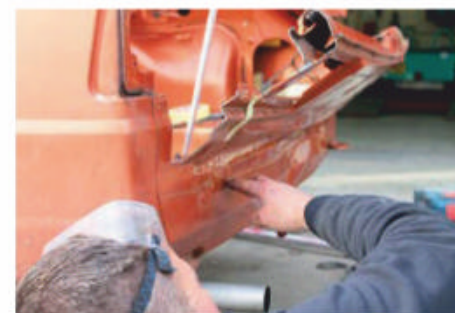
Tracking the seam weld.
