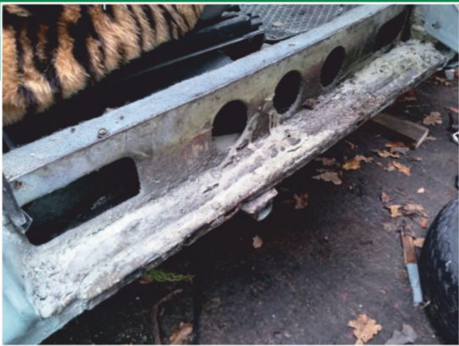
Although there are some rust flakes, the wax inserted into the sills seven years ago has done a good job at keeping rust at bay.
