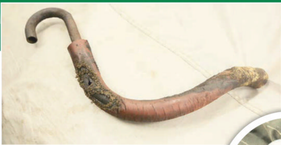
ABOVE: Not a pretty sight – the hidden part of the overflow pipe had seen better days.
