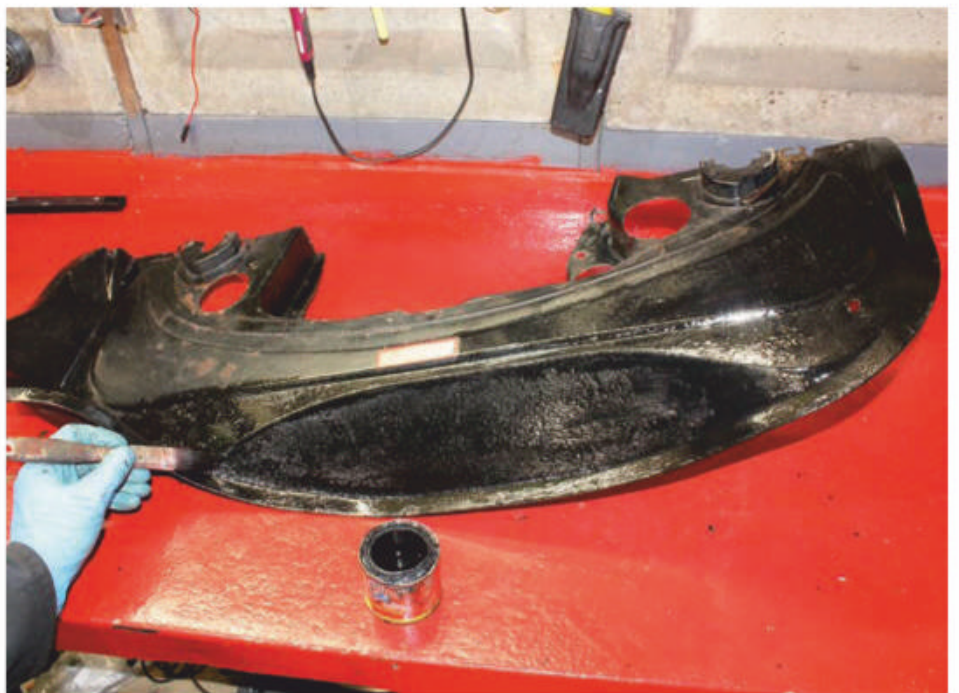
Surface corrosion on the engine tinware was cleaned off before a couple of coats of POR-15 were applied to protect it.
