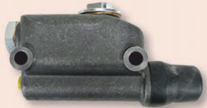
The Morris Minor brake master cylinder which is hidden in a chassis rail under the floor.
