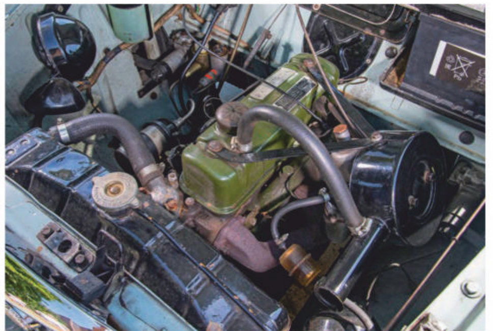
ABOVE and BELOW: For such a small car, the 1489cc B-series was a decent sized motor. It was Wolsley's first small car since 1948, but the traditional illuminated Wolseley badge on the radiator grille remained.
