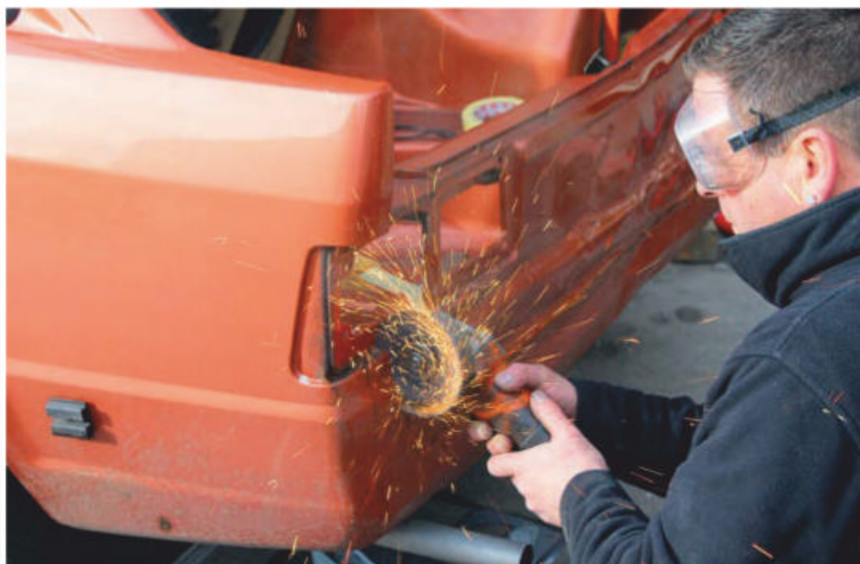
Paul cuts into the damaged back panel, leaving plenty of space away from the sides of the panel during this initial stage.
