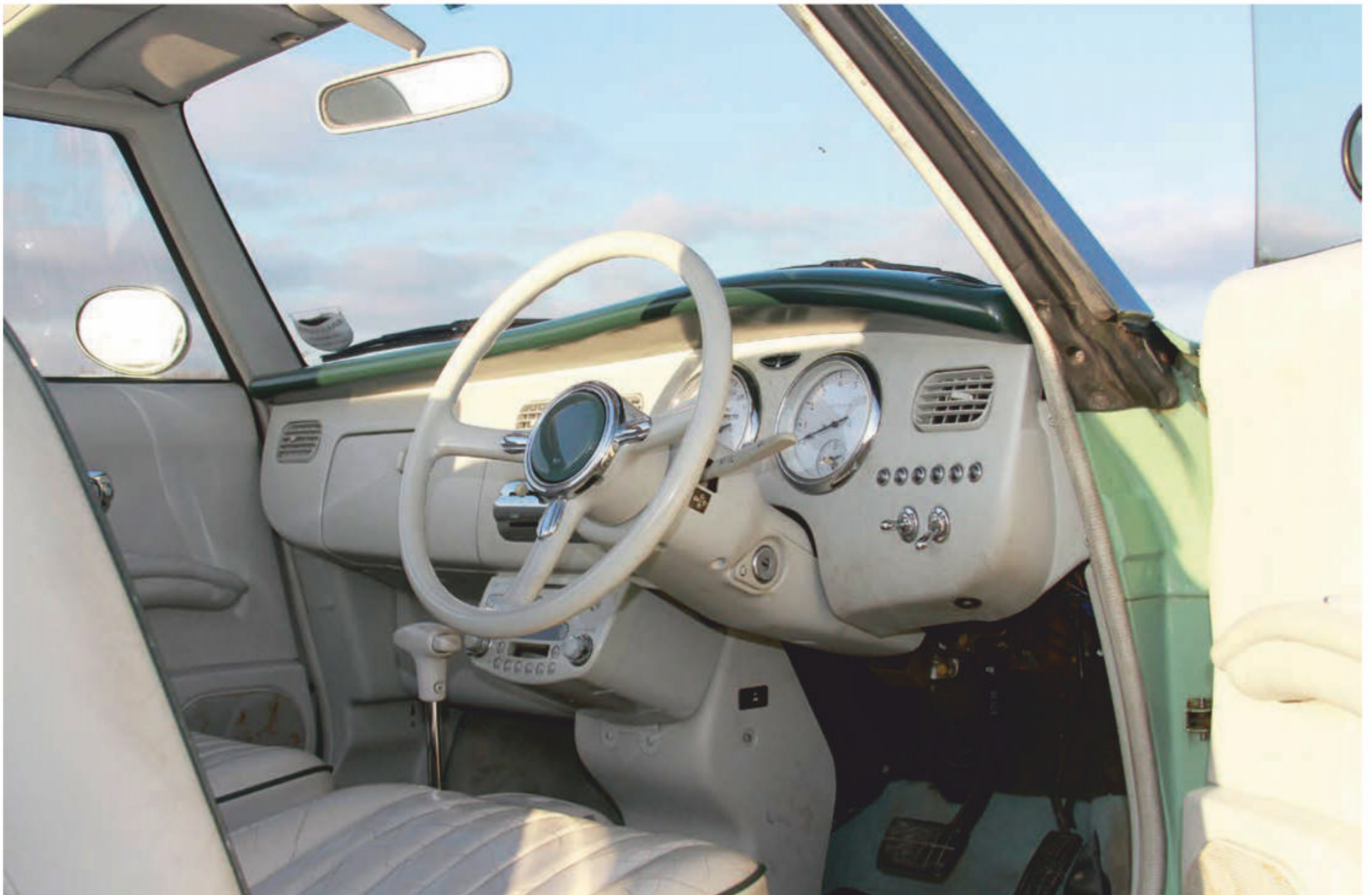
The Figaro's interior is as beautifully styled as the exterior. Initial issues are a cracked top to the dash, indicators that are temperamental, a non-functioning electric window and a handbrake lever that's been wrapped up in insulating tape.
