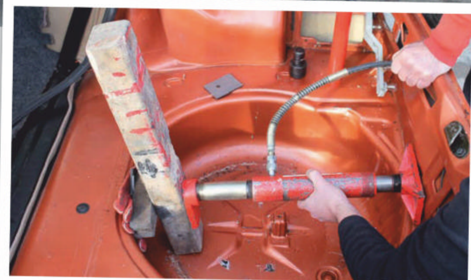
ABOVE AND RIGHT: Hydraulic ram was used to ease the back panel straight again.
