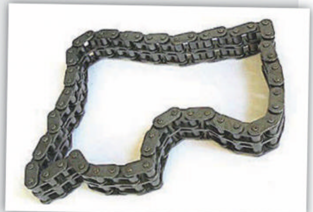
Perhaps modern car makers could learn from the older engines – the chain on this 1956 engine is a duplex chain and has lasted over 60 years.
