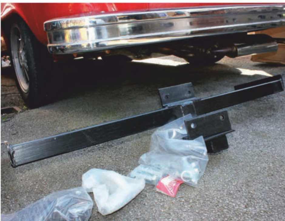
The tow bar is designed to fit neatly behind the rear bumper and onto the existing bumper mounting points.
