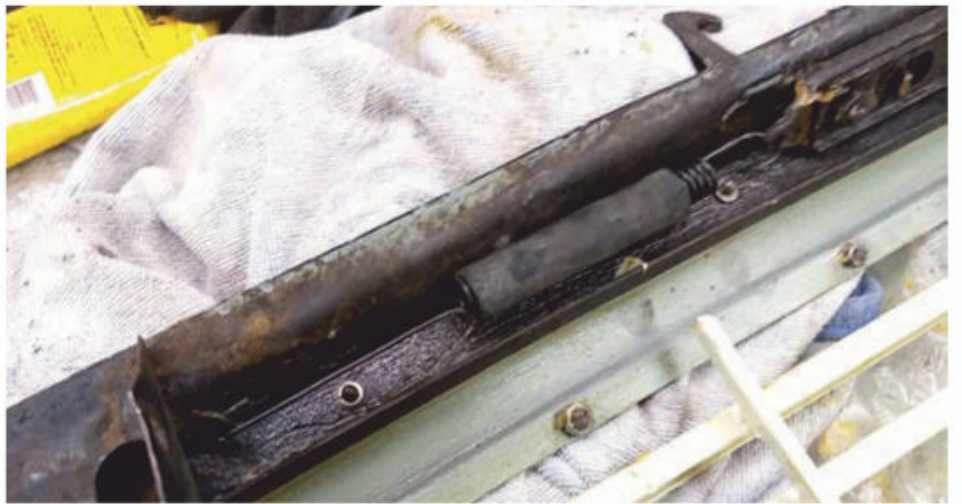
When re-assembling the front panel, it became necessary to replace the bonnet spring after the original broke on re-fitting.
