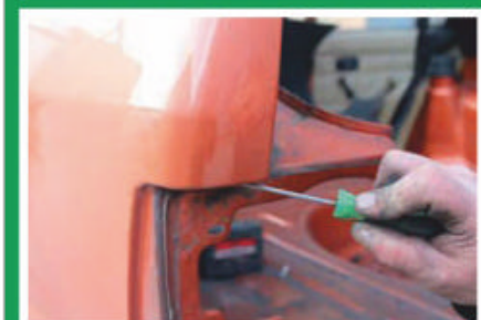
Tracking the seam weld around the taillight.
