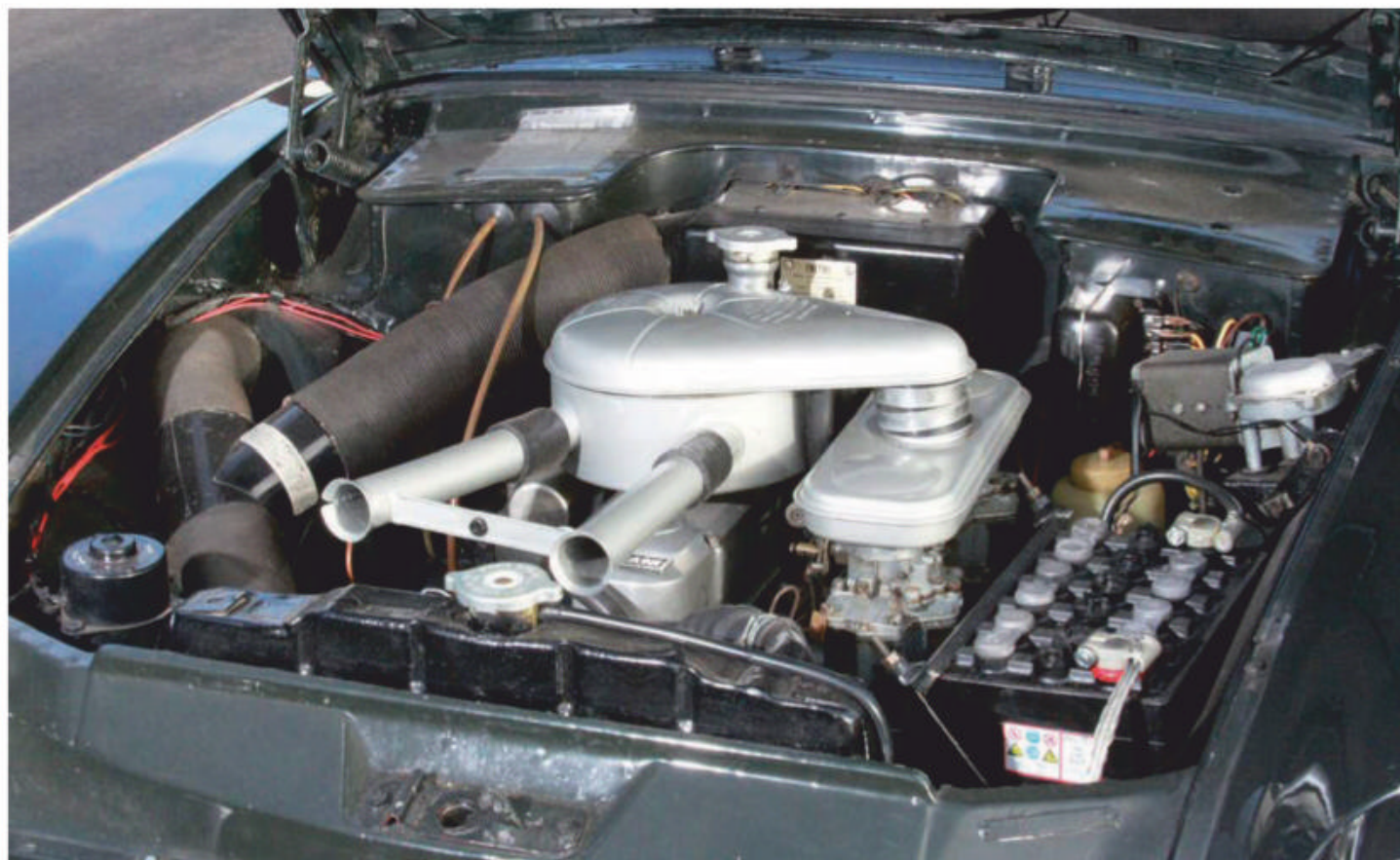
For the Series IIIA Rapier, the engine grew to 1592cc, which produced up to 80bhp@5100rpm. With an aluminium cylinder head, not to mention front disc brakes, it was very well spec'd for the early 1960s.
