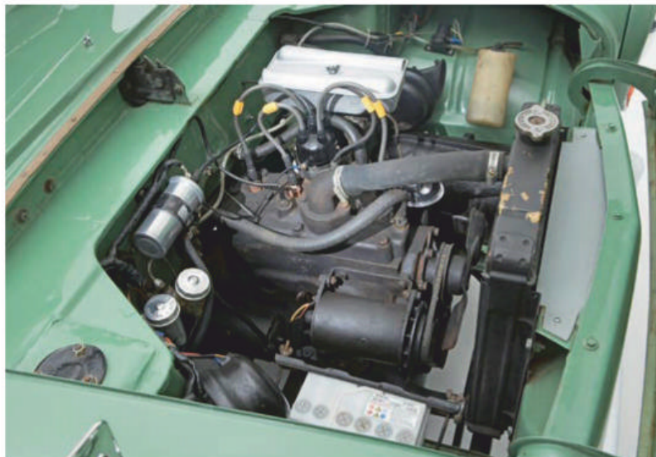
The 1172cc sidevalve engine of the 100E could trace its lineage back to the 1930s, but it was a quiet and willing performer.
