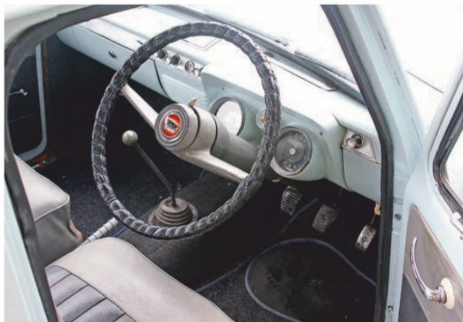
Worm and peg steering was never exactly pin sharp, but when it is in good condition the car should feel light and pleasant to drive.
