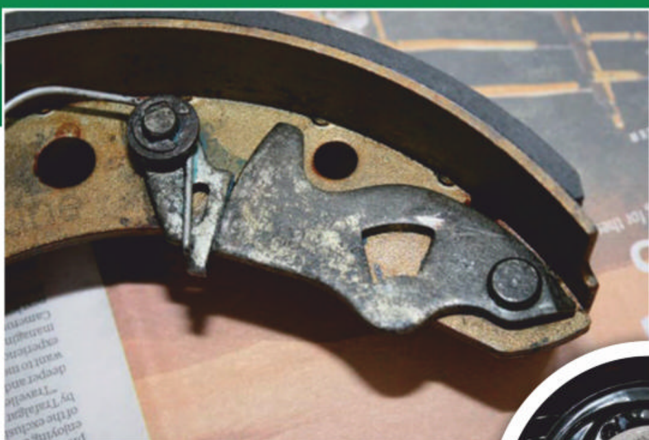
Prior to fitting the new brake shoes, the adjusters had to be transferred from the old ones.
