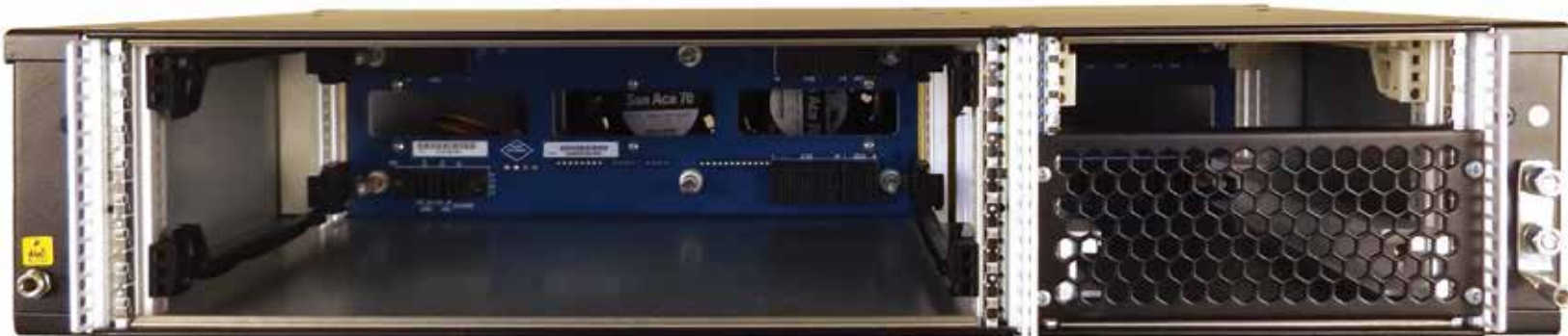
Figure 4 - Horizontal-mount OpenVPX chassis platforms can save significant rack space. The 2U high chassis in this example pulls air in a front-to-rear airflow configuration, but can be modified for side-to-side cooling requirements.
