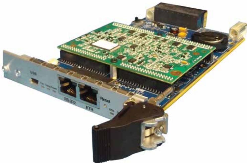
Figure 2 - The SOSA/HOST effects are beginning to employ VITA 46.11 Chassis Managers for OpenVPX. This example board can plug into any standard OpenVPX slot via the P0 connector.
