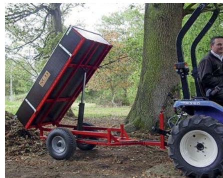
ABOVE FROM LEFT The GWT415 features four wheels, giving it stability over rough and wet terrain; The HTRL is the largest of the wooden trailers and it boasts four hydraulic options
