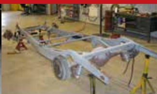
Truck owned by Bill Leohr Installed IFS electric steering & power windows
